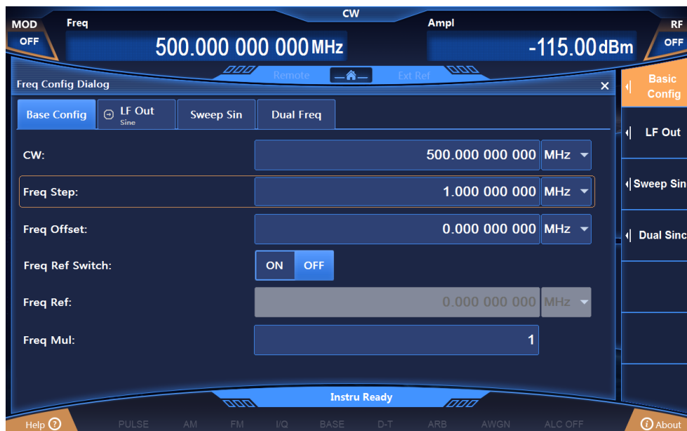
Figure 3.1 Setting CW to 500 MHz and frequency stepping value to 1 MHz
