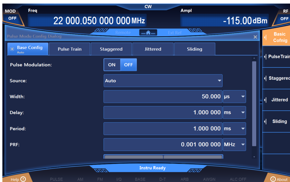
Figure 3.4 Setting pulse modulation signals
