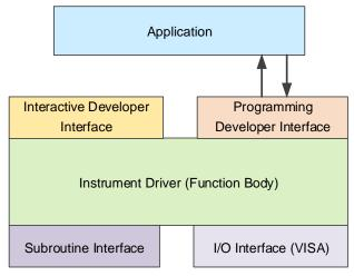
Figure 5.2 Structure Model of Instrument Driver
