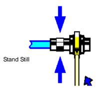
Figure 3.5 Tighten with A Torque Wrench to Complete Final Connection
