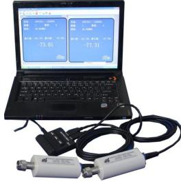
Figure 4.4 Multi-Channel Power Measurement by Using USB HUB
