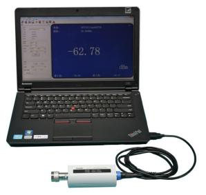
Figure 3.2 Connection of 87230 Series USB Continuous Wave Power Sensor to a Computer
