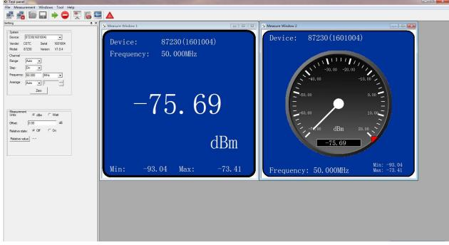
Figure 4.2 Power Measurement Virtual Panel
