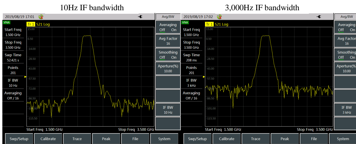
Figure 4-2 Effect of IF Bandwidth on Measurement Results
