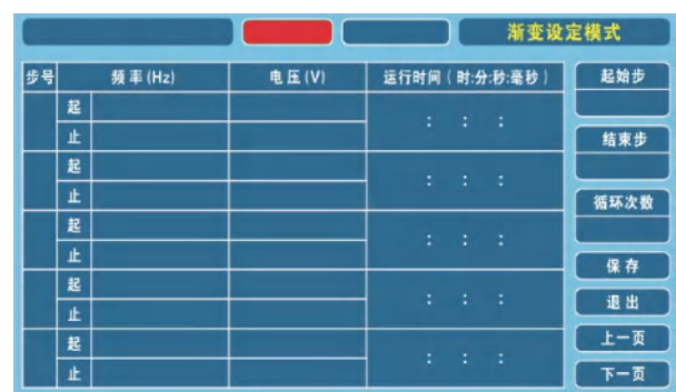
The gradient settings page allows you to set the required voltage and frequency Run time, initial step, end step
