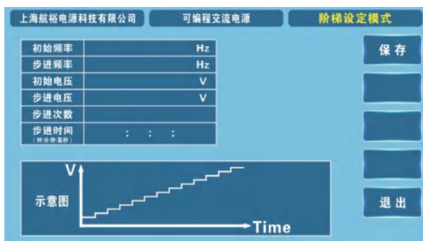
The ladder setting page can set the desired initial frequency, Step frequency, initial voltage, step voltage, number of steps, and Step time
