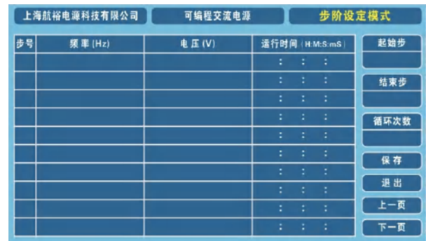
The step setting page allows you to set the required frequency, voltage Run time, initial step, end step, and number of cycles
