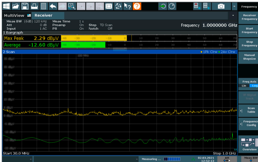
Displayed average noise level (DANL) up to 1 GHz. The noise figure with the preamplifier switched on is approx. 8.5 dB.
