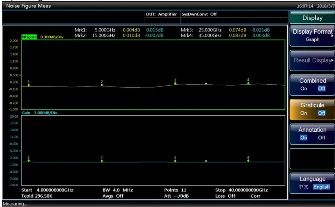
Fig. 3.36 Typical graph display with graticule switched off
