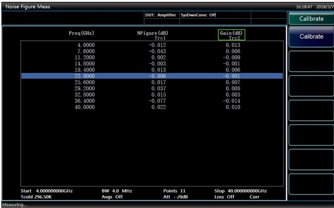
Fig. 4.11 Typical Table Display Result after Calibration
