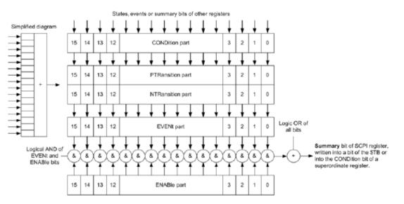
Figure 2.5 Structure of status register
