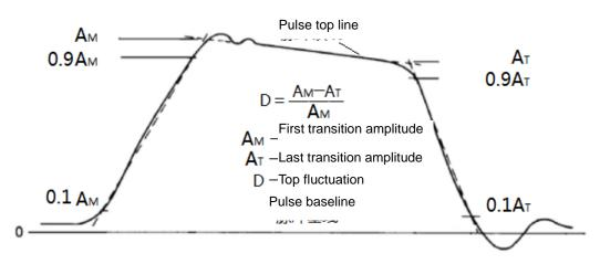
Figure 3.3 Pulse top fluctuation
