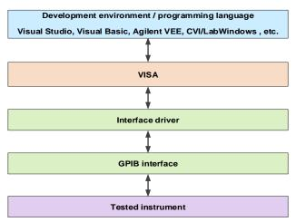
Fig.4.1 Programmable software/hardware layer
