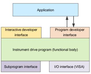
Figure 2.7 Structure model of instrument driver
