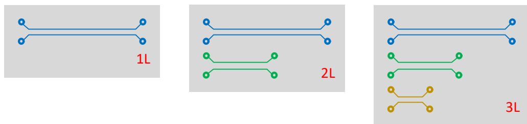
Figure 4-35: Test coupons for 1L, 2L and 3L measurements
