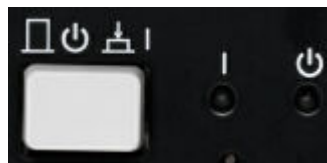
Figure 3-13: Standby switch and LEDs
