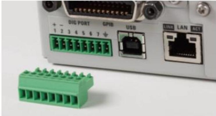
**Figure 10.** Digital control port on rear panel
