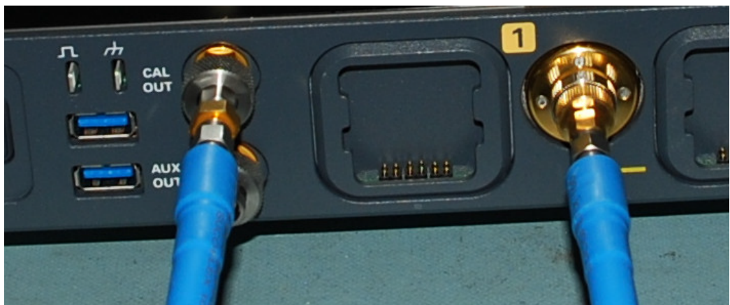
Figure 8 Verifying basic oscilloscope operation -- models with 1.0 mm connector types
