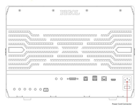
Figure 4.3 To Connect to AC Power
