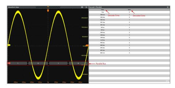
**Figure 18.3 Parallel Decoding Event Table**
