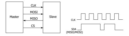
Figure 18.11 SPI Serial Bus
