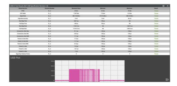
Figure 19.2 USB2.0 Signal Quality Compliance Analysis Test Result
