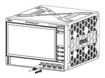
**Figure 4.6 Connect the Active Probe**
