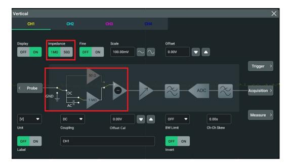
**Figure 5.2 Input Impedance Modification**
