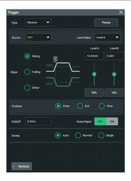
Figure 8.17 Window Trigger Setting Menu
