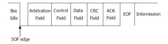
Figure 8.34 Data Frame Format of the CAN Bus
