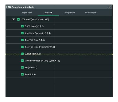
Figure 20.2 100Base-T Signal Test Items
