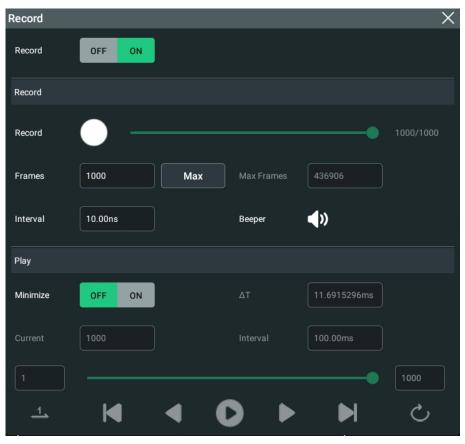
**Figure 23.1 Waveform Recording Interface**
