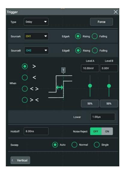
Figure 8.19 Delay Trigger Setting Menu
