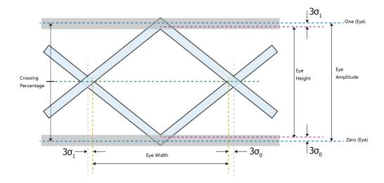
Figure 13.3 Diagram of Eye Measurement Parameters
