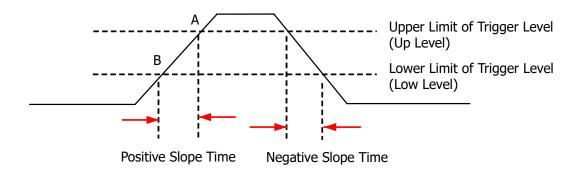
Figure 8.6 Positive Slope Time/Negative Slope Time
