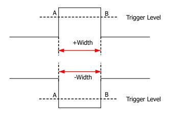
Figure 8.4 Positive Pulse Width/Negative Pulse Width
