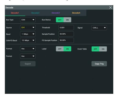
Figure 18.16 CAN Decoding Menu
