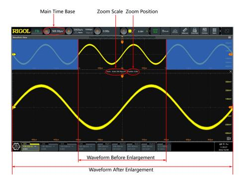
Figure 6.2 Delayed Sweep Mode
