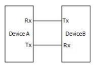
Figure 18.4 Schematic Diagram of RS232 Serial Bus
