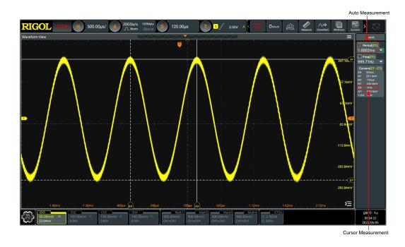
Figure 10.11 Manual Cursor Measurement Example
