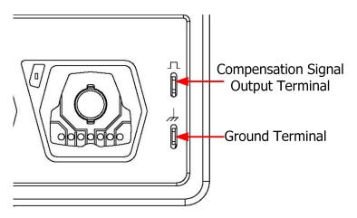
Figure 4.7 To Use the Compensation Signal
