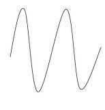
• **Waveform Leakage:** when the sample rate is too low, the waveform rebuilt from the sample data does not reflect all the actual signal information.
