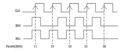
Figure 18.1 Schematic Diagram of Parallel Decoding
