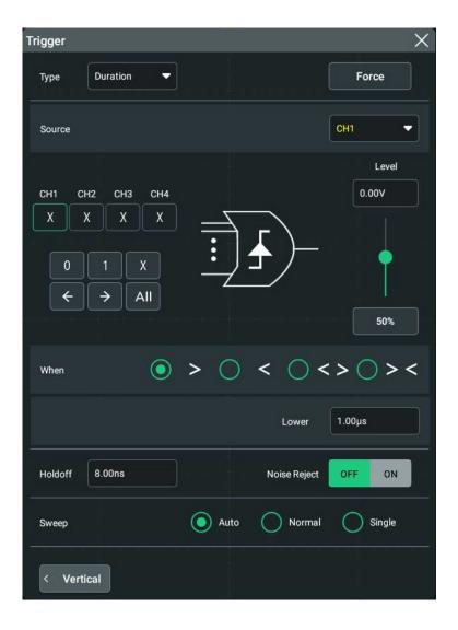
Figure 8.12 Duration Trigger Setting Menu
