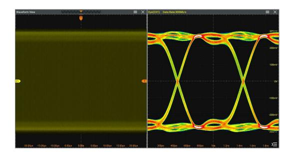
Figure 13.2 Eye Measurement Result
