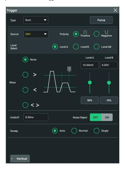
Figure 8.16 Runt Trigger Setting Menu
