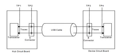
Figure 19.1 USB2.0 Test Model
