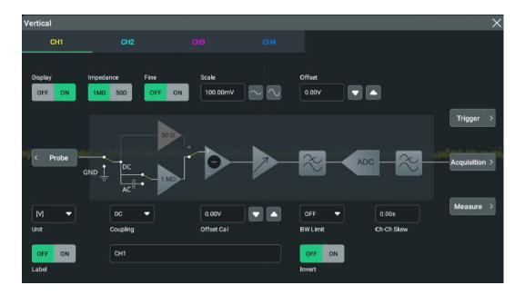
**Figure 5.1 Vertical Menu for Channel**
