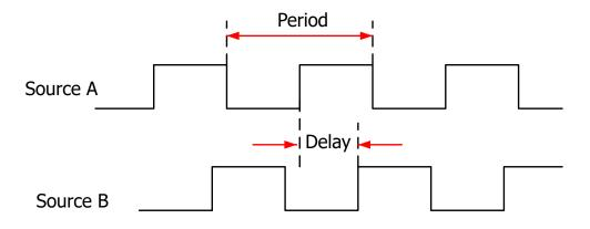
**Figure 10.2 Delay and Phase Parameters**
