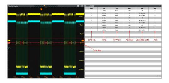
Figure 18.10 I2C Decoding Event Table
