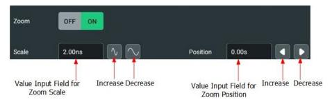
• **Scale:** Click or tap the icon at the right of the **Scale** input field under the **Zoom** menu to increase or decrease the zoom scale. You can also click or tap the value input box to input the specific value directly via the pop-up numeric keypad.
