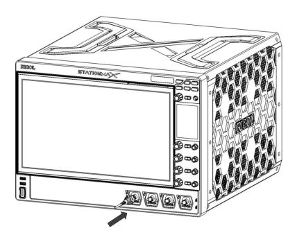
**Figure 4.4 Connect the Passive Probe**
