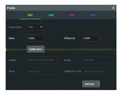
Figure 5.5 RP7000/PVA7000/PVA8000 Probe Setting Menu
