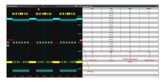
Figure 18.13 SPI Decoding Event Table
