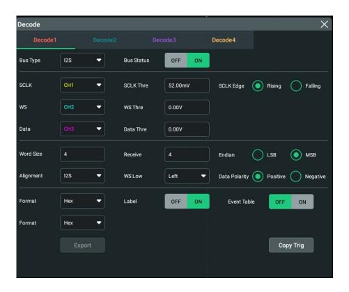
Figure 18.22 I2S Decoding Menu
