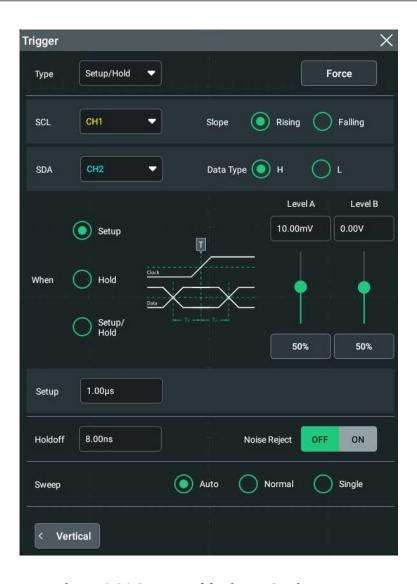
Figure 8.21 Setup/Hold Trigger Setting Menu
