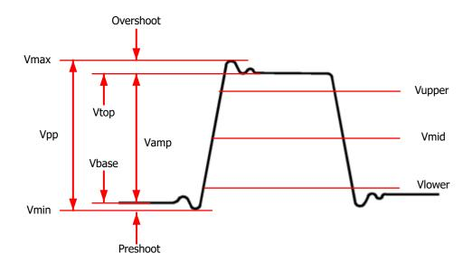
Figure 10.3 Voltage Parameters
