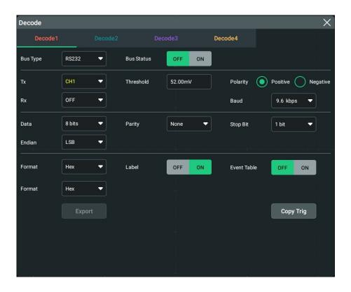
Figure 18.6 RS232 Decoding Menu
