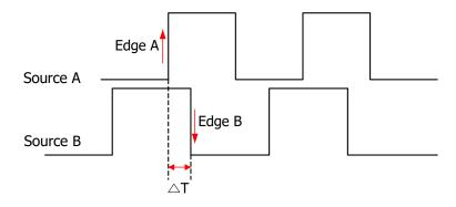
Figure 8.18 Delay Trigger
