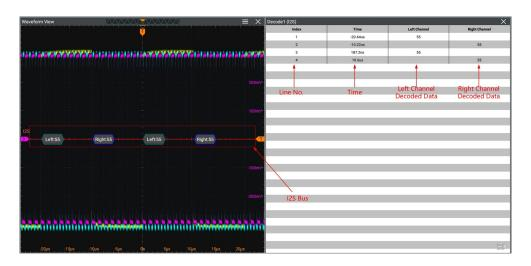
Figure 18.23 I2S Decoding Event Table
