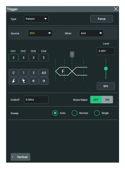
Figure 8.10 Pattern Trigger Setting Menu
