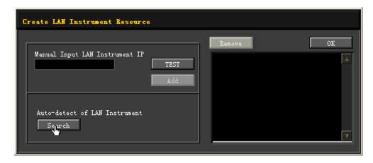
Besides, you can input the IP address of the instrument manually into the text field under "Manual Input LAN Instrument IP", then click **TEST**. If the instrument passes the test, click **Add** to add the instrument to the LAN instrument resource list in the right section; if the instrument fails the test, please check whether the IP address that you input is correct, or use the auto search method to add the instrument resource.
