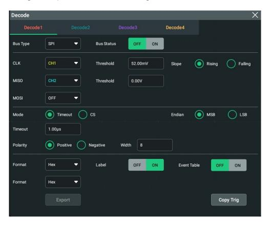
Figure 18.12 SPI Decoding Menu
