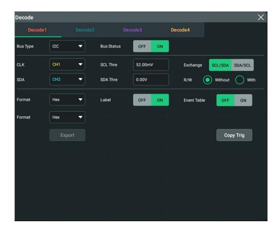
Figure 18.9 I2C Decoding Menu
