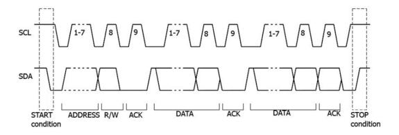
Figure 8.26 Schematic Diagram of I2C Protocol
