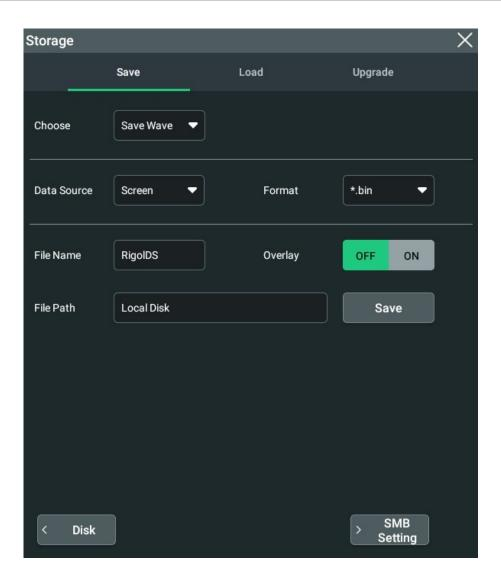
Figure 25.2 Waveform Saving Setting Menu
