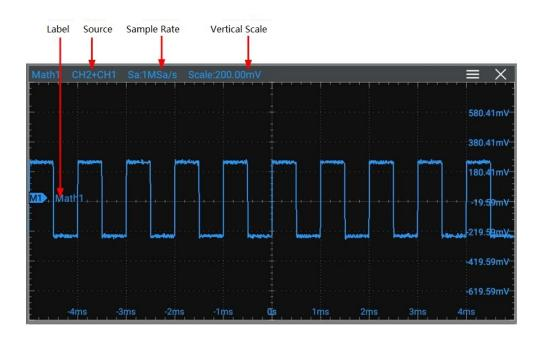
**Figure 9.4 Operation Result Display Window**
