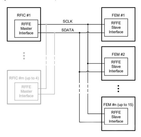
Figure 18.26 MIPI RFFE System Architecture
