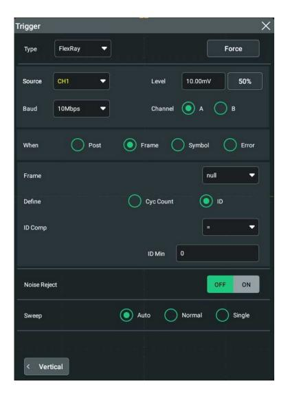
Figure 8.38 FlexRay Trigger Setting Menu
