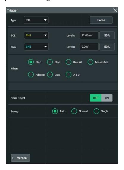
Figure 8.27 I2C Trigger Setting Menu
