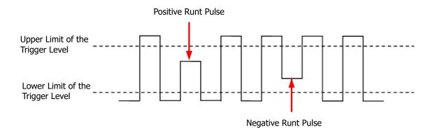
Figure 8.15 Runt Trigger
