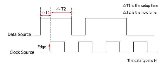
Figure 8.20 Setup/Hold Trigger
