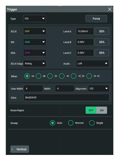
Figure 8.43 I2S Trigger Setting Menu
