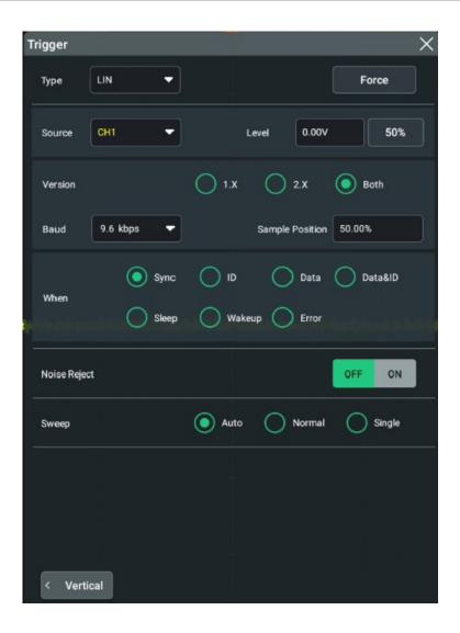
Figure 8.40 LIN Trigger Setting Menu
