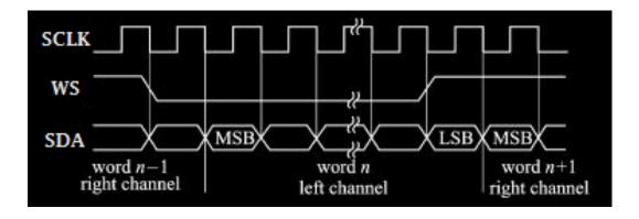
Figure 8.42 Sequential Chart of I2S Bus
