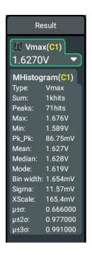
**Figure 10.16 Measurement Histogram Result**
