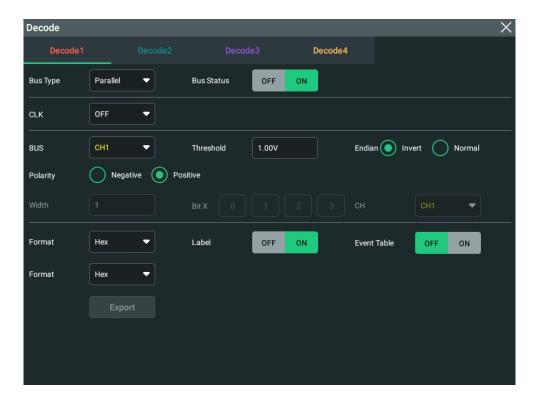
Figure 18.2 Parallel Decoding Menu
