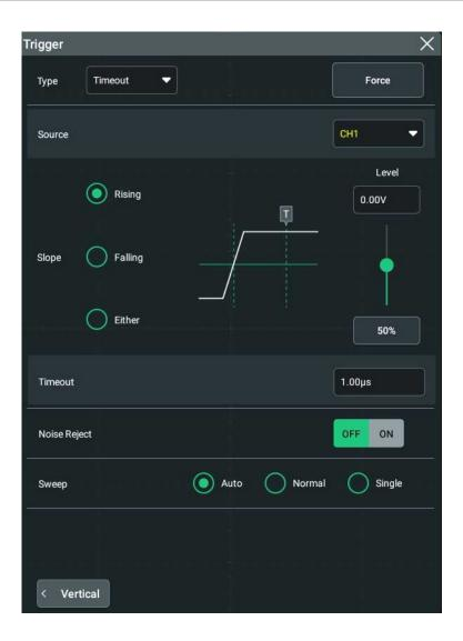
**Figure 8.14 Timeout Trigger Menu**
