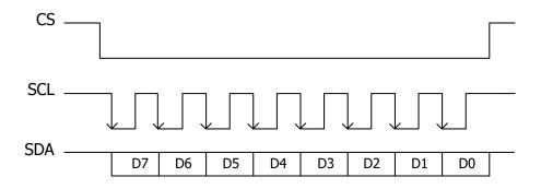
Figure 8.32 Sequential Chart of SPI Bus
