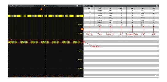
Figure 18.18 CAN Decoding Event Table
