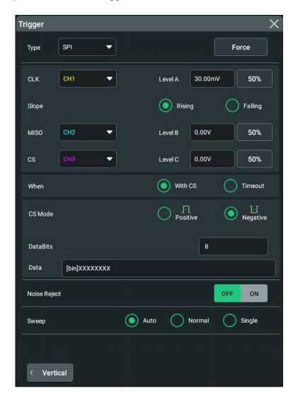
Figure 8.33 SPI Trigger Setting Menu
