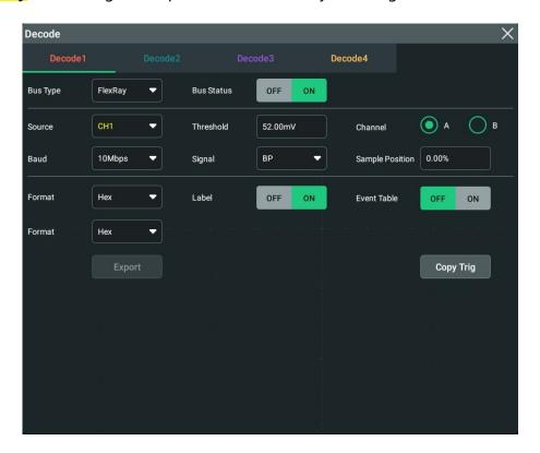
Figure 18.19 FlexRay Decoding Menu
