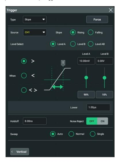
**Figure 8.7 Slope Trigger Setting Menu**
