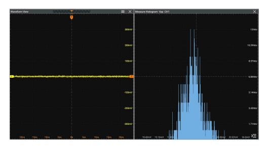
Figure 10.17 Measurement Histogram Window
