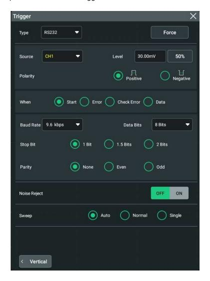
Figure 8.25 RS232 Trigger Setting Menu
