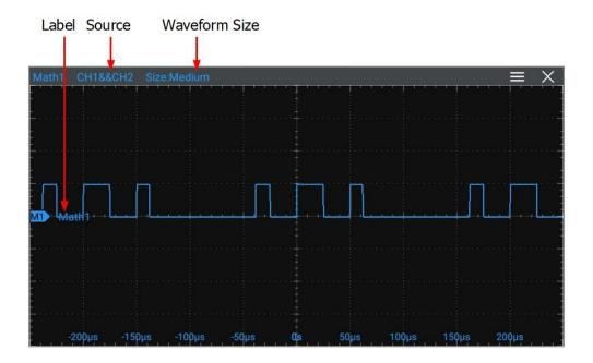
Figure 9.11 Operation Result Display Window
