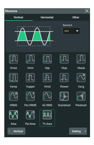
**Figure 10.4 Vertical Measurement Items**
