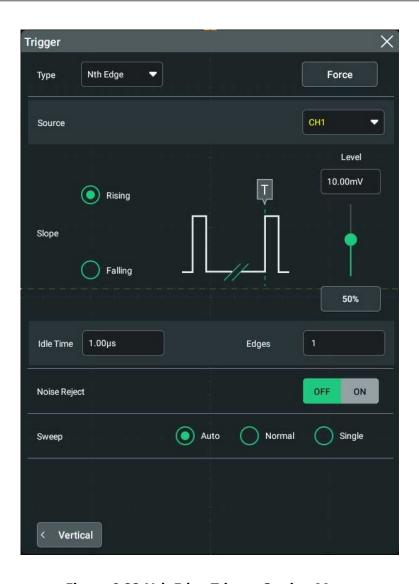
Figure 8.23 Nth Edge Trigger Setting Menu
