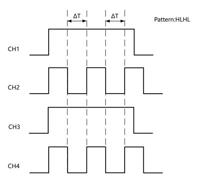
**Figure 8.11 Duration Trigger**
