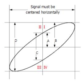
Figure 7.4 Measurement Schematic Diagram of Phase Deviation
