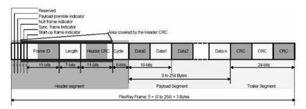
Figure 8.37 Frame Format of FlexRay Bus
