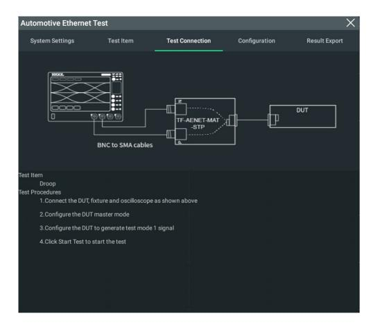
**Figure 21.8 Test Connection and Test Procedures**
