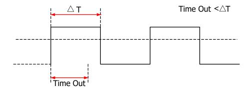
Figure 8.13 Timeout Trigger
