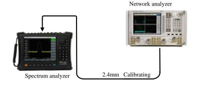
Fig. 12-18 Voltage Standing Wave Ratio Test of Input Port
