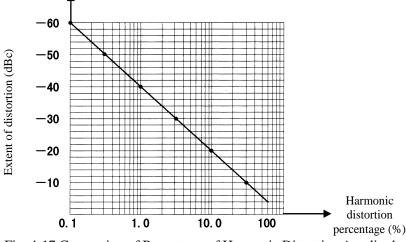
Fig. 4-17 Conversion of Percentage of Harmonic Distortion Amplitude
