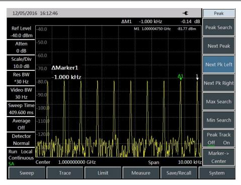
Fig. 4-24 Measurement of Pulse Repetition Frequency
