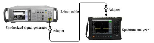
Fig. 4-1 Schematic Diagram of Connection of Signal Generator and Spectrum Analyzer
