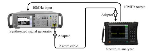
Fig. 12-6 Setting for Resolution Bandwidth Conversion Uncertainty
