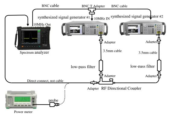
Fig.12-10 Setting for 3-order intermodulation distortion Test (50MHz~4GHz)
