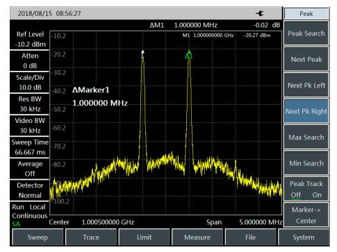
Fig. 4-6 Signals at Center of Display of Spectrum Analyzer e) Set the reference level and make the signal peak at the reference level:
