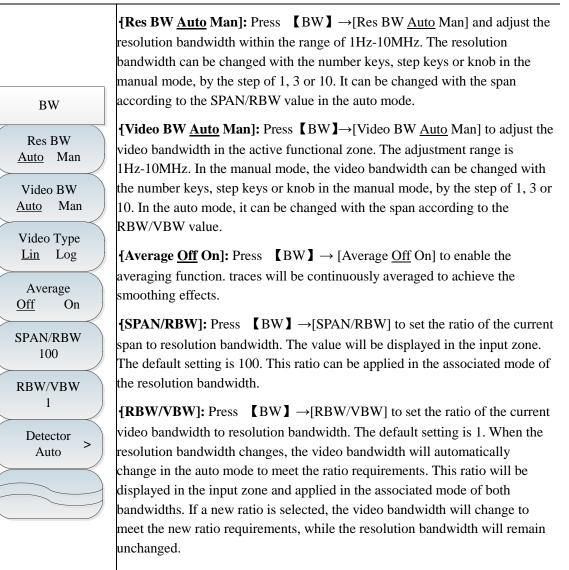
**[Detector]:** Press  $[BW] \rightarrow [Detector]$ , and the soft menu of detector mode will pop up. Refer to the [Detector] menu description for details.
