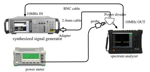
Fig. 12-16 Setting for Total Level Uncertainty Test
