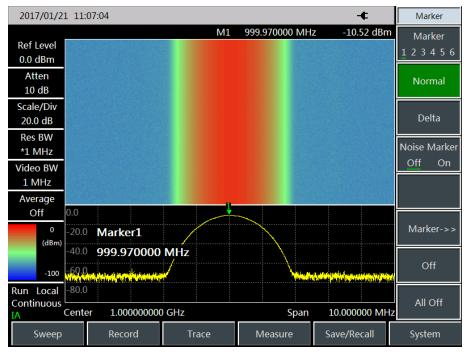
Fig. 5-1 Interference Analyzer Spectrogram
