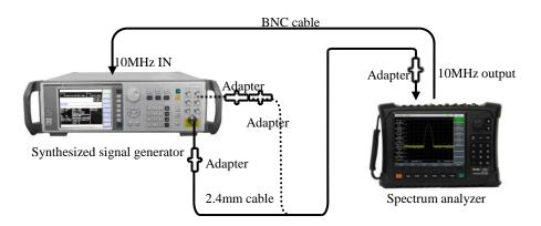
Fig. 12-1Frequency Range Test
