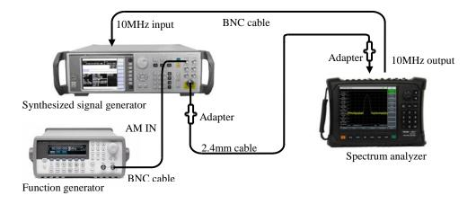
Fig. 12-4 Setting for Sweep Time Accuracy Test
