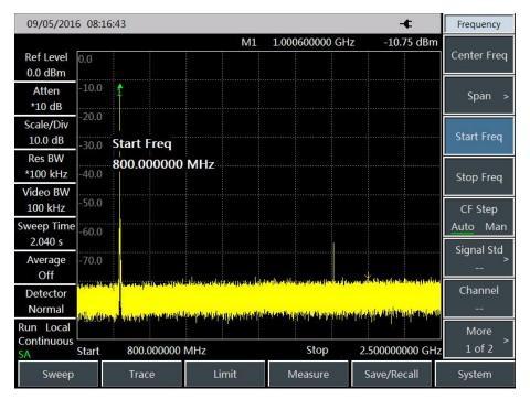
Fig. 4-14 Input Signal and Harmonic
