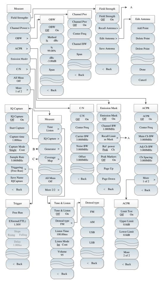
Fig. 4-32 Overall Block Diagram of Spectrum Analysis Menu (continued)
