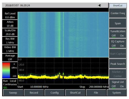
Fig. 10-1 Main interface display of signal analysis measurement mode
