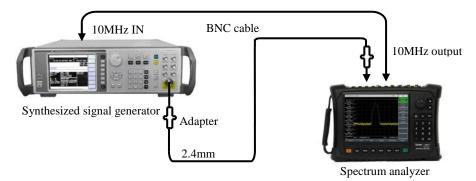
Fig. 12-17 Setting for Input Attenuator Switching Uncertainty Test
