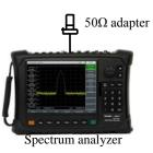
Fig. 12-8 Setting for Display Average Noise Level Test
