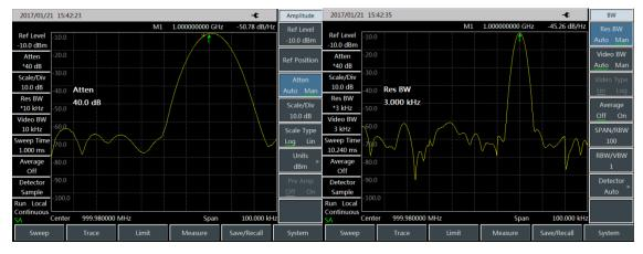
Fig. 4-11 Noise Measurement by Noise Marker Function
