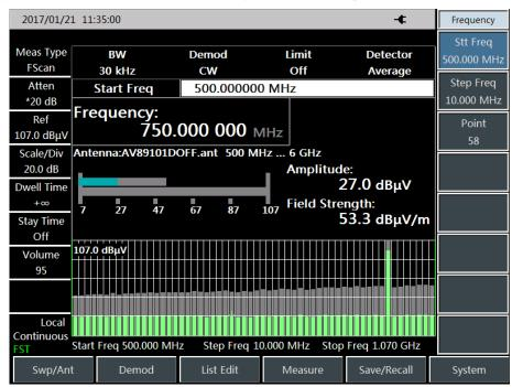
Fig. 9-2 Schematic Diagram of FScan Mode
