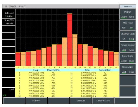
Fig. 8-1 Schematic Diagram of Channel Scanner
