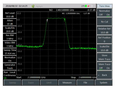
Fig. 4-27 Magnitude-frequency characteristics diagram of 2.3GHz~2.4GHz band-pass filter
