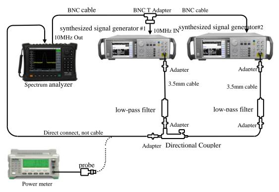
Fig.12-11 Setting for 3-order intermodulation distortion Test (4GHz~44GHz)
