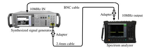
Fig. 12-3 Setting for Bandwidth Accuracy Test
