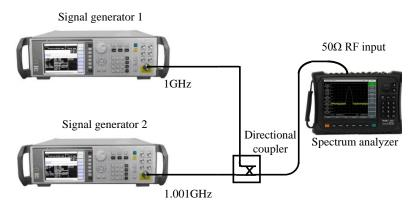
Fig. 4-5 Connection of Third-order IM Distortion Measurement System
