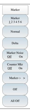
[Marker  $\underline{1} 2 3 4 5 6$ ]: press [Marker]  $\rightarrow$  [Marker  $\underline{1} 2 3 4 5 6$ ], to activate the different marker display. The selected marker will be underlined.
