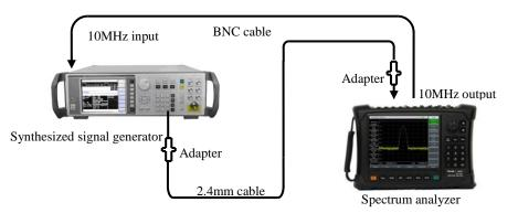
Fig. 12-5 Setting for Resolution Bandwidth Accuracy Test
