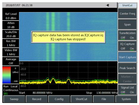
Fig. 10-3 Schematic diagram of IQ Capture function
