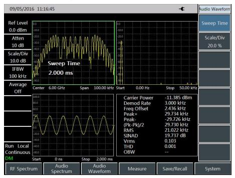
Fig. 7-1 FM Demodulation Analysis Results
