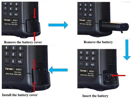
Fig. 2-1Battery Installation and Replacement Steps
