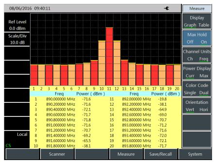
Fig. 8-3 Schematic Diagram of List Scanner
