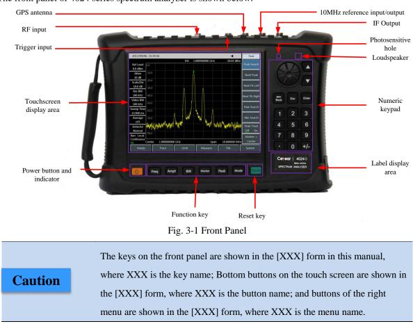
The front panel of 4024 series spectrum analyzer is shown below.
