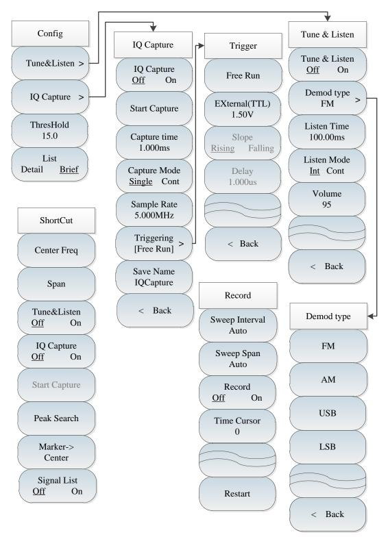
Fig. 10-6 Block diagram of signal analysis menu (continued)
