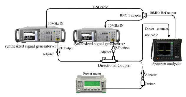
Fig. 12-12 1dB Gain Compression Test
