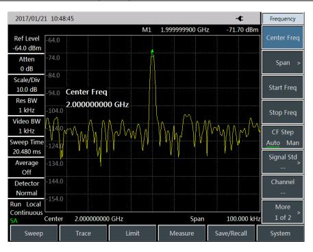
Fig. 4-19 Second Harmonic Amplitude
