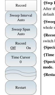
**[Swp Interval]:** press **[**Record **]**  $\rightarrow$  [Swp Interval Auto], to set the scan interval. After the sweep time is set, the trace will switch to the maximum hold mode by default to ensure that all measured signals within scan interval can be recorded.
