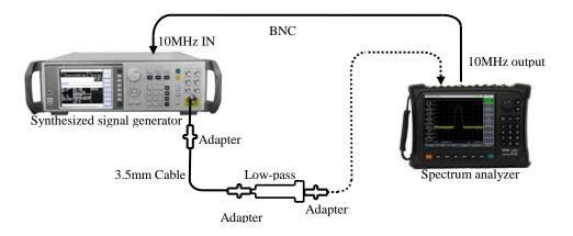
Fig. 12-9 Setting of Second Harmonic Distortion Test
