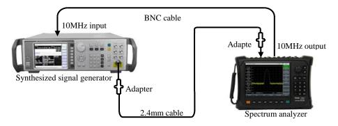
Fig. 12-7 Schematic Diagram of Sideband Noise Test
