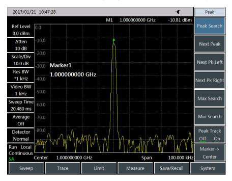
Fig. 4-18 Input Signal under 100kHz Span
