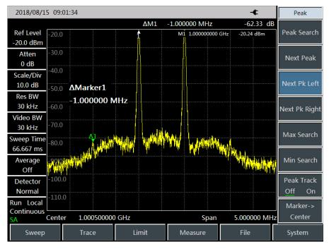
Fig. 4-8 Relative Measurement of Internal Modulation Distortion g) Calculation of third-order interception (TOI) point:
