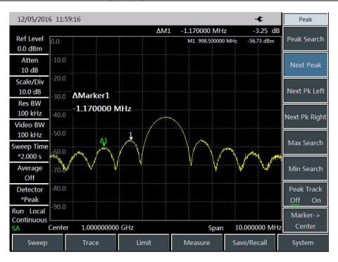
Fig. 4-23 Pulse Width Shown by the Marker
