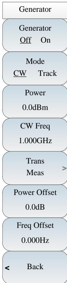
{**Signal Source Off On**}: press **【 Measure 】** → [More 1 of 2] → [Generator] → [Generator **Off On**], to activate or deactivate the signal source.
