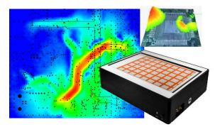
EMC and signal integrity are major concerns in the design of ultra-high speed (>2 GHz) PCBs. EMScanner enables the design engineers to diagnose EMC/EMI problems between 150 kHz and 8 GHz.
