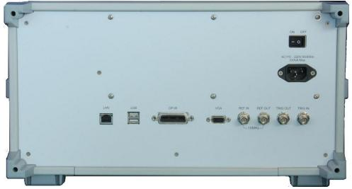
The rear panel of Analyzer is shown as the following Figure .:
