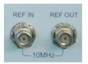
Fig. 4-17 10MHz Reference Connector
