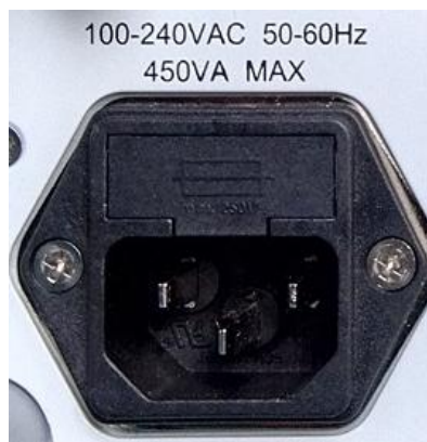
Fig. 3.1 Power Outlet on the Rear Panel of 2438 Microwave Power Meter
