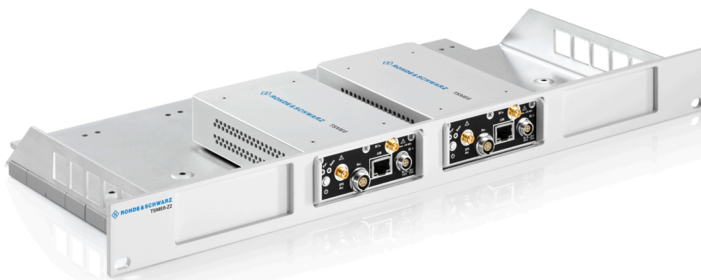
Figure 3-2: Rackmounting of 2 R&S TSME6s (reverse orientation of R&S TSME6s)
