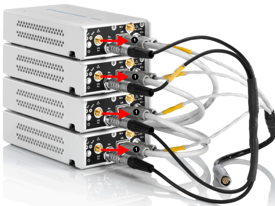
Figure 3-17: LAN cable connected to LAN connectors of 4 R&S TSME6 devices
