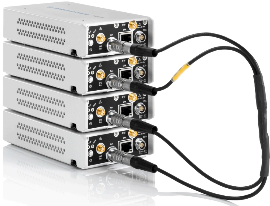
Figure 3-14: SYNC-cable connected to Aux. connectors of 4 R&S TSME6 scanners
