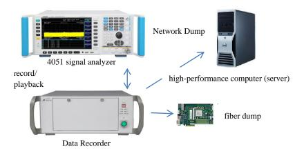
RF signal streaming and playback analysis function
