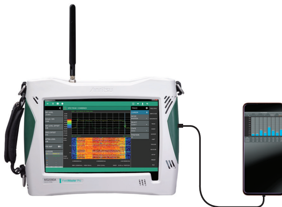
Field Master Pro MS2090A can be Controlled by an Android Smartphone
