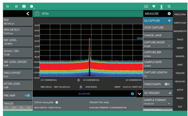
Free Run, External, Video, and Level Trigger Options are Available in the RTSA Mode to Initiate IQ Data Capture
