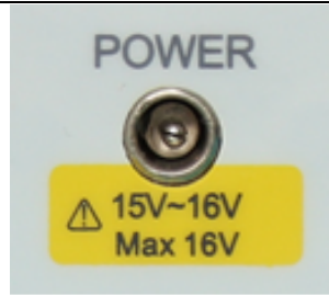
Figure 5-6 Power Input Port
