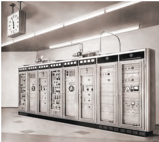
1963: VHF radio transmitter with 2 × 5 kW
