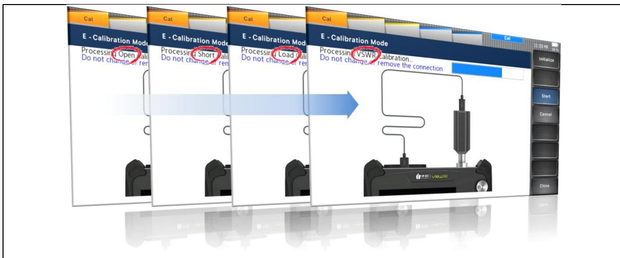
When calibration done successfully, the screen automatically returns to the measurement screen. CAL "On." Icon will be displayed.
