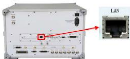
Fig. 2.7 LAN Interface of Rear Panel of Instrument
