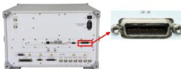
Fig. 2.10 GPIB Interface of Rear Panel of Instrument
