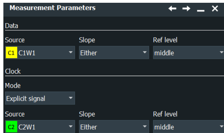
Figure 18-1: Settings for time interval error measurement with real clock signal
