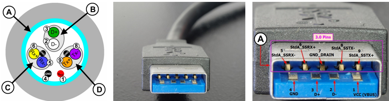
Figure 13-31: USB 3.1 cable cross-section and Standard-A plug - backward compatible with USB 2.0
