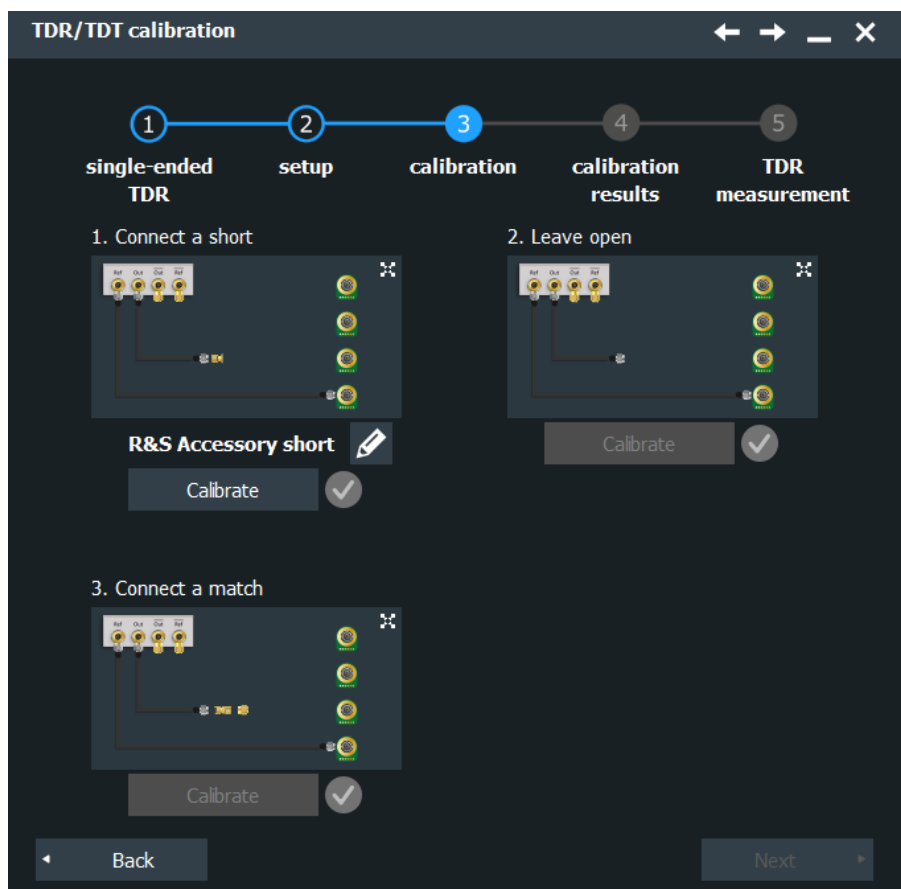
Figure 16-4: Calibration of single-ended TDR/TDT
