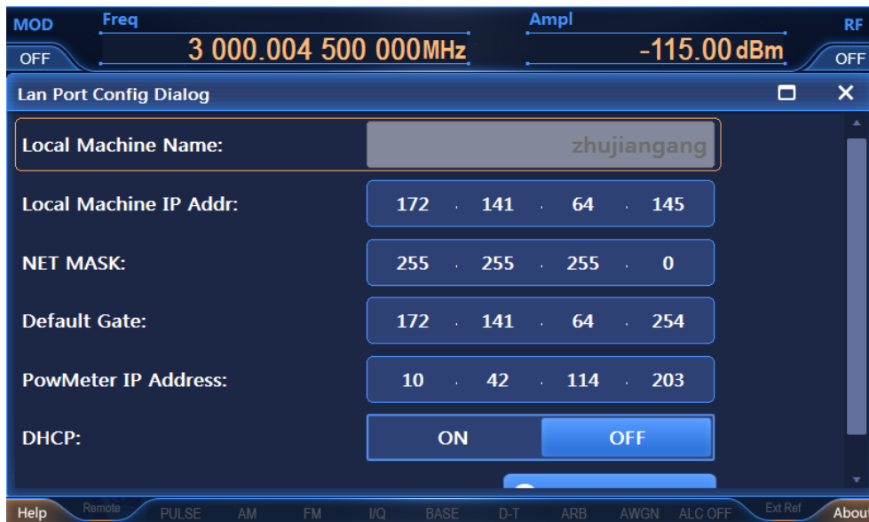
Figure 3.10 Lan port configuration
