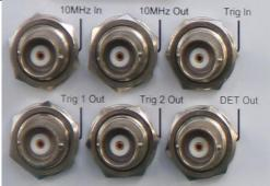
Fig. 3.16 BNC Ports on Rear Panel
