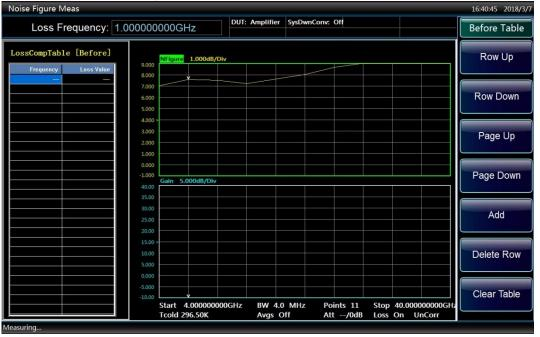
Fig. 4.53 loss table (Blank)
