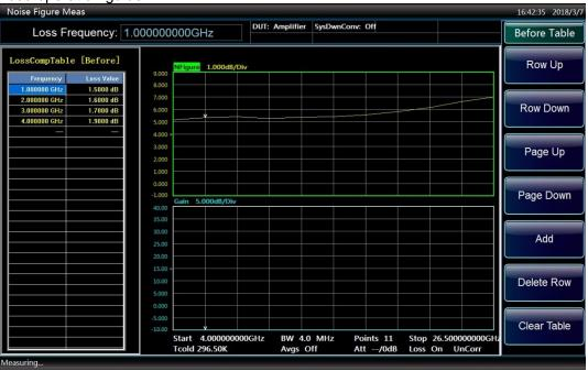
Fig.4.54 Loss Table after Data Input
