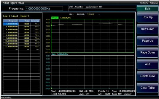
Fig.4.56 Typical Limit Line Table
