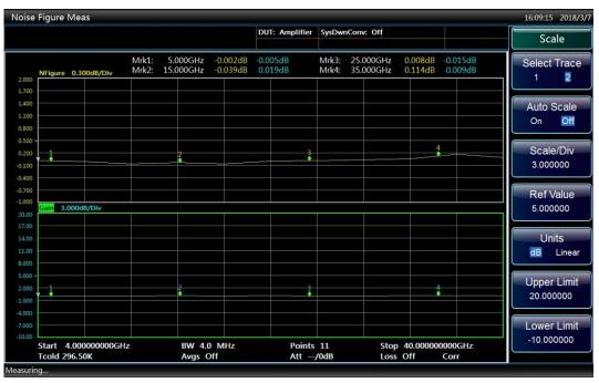
Fig. 3.38 Typical noise figure displayed on a graph
