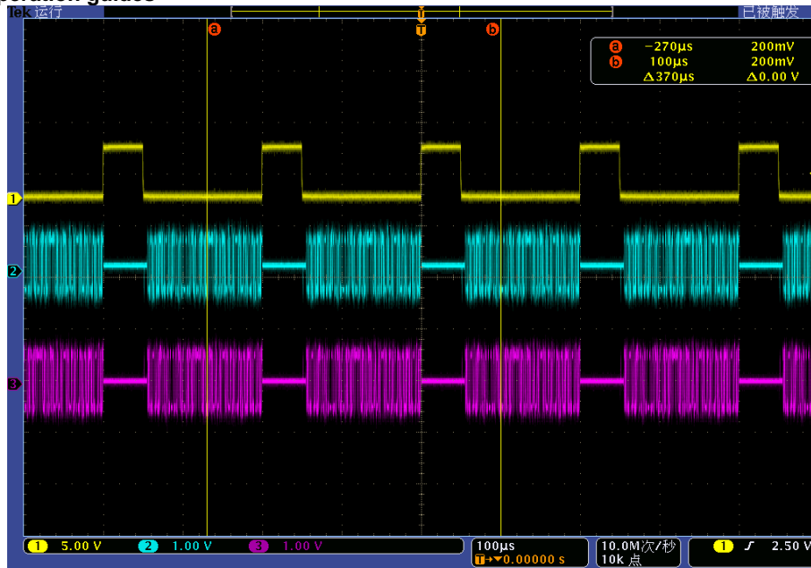
Fig. 4.23 Diagram of Baseband Triggering (Gate/Low)
