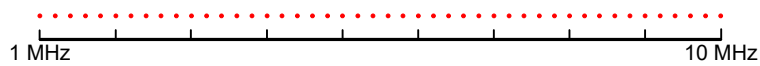
Figure 7-26: Linear x-axis scaling: the distance between the sweep points is equal, e.g. 200 kHz
