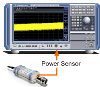
Figure 7-3: Connecting a power sensor using the POWER SENSOR interface
