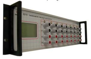
The optional 3210 Thermometry Adaptor with pre-heat enables multiple Resistance Temperature Devices to be calibrated at the same time along with providing programmable pre-heat capability. The Guildline SPRT Adaptor is the only scanner/adaptor that can provide programmed pre-heat currents on a per channel basis. Other manufacturers do not have pre-heat capability or only provide a single, fixed, preheat current.
