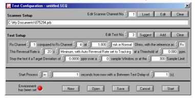
**BridgeWorks** software offers many routine **thermometry functions such as SPRT calibrations** to ITS-90 scale. It also provides comprehensive graphic display, math functions and trend analysis. Data can be **easily exported** to MS-Excel®, Crystal Reports® and in HTML format. All reports generated conform to traceability requirements of ISO 17025.
