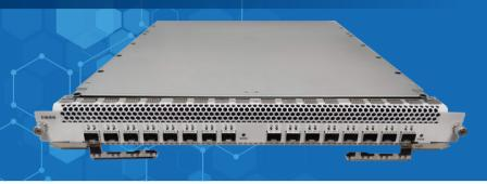
With professional L2-7 traffic generation and analysis capabilities, X2-10G multi-rate test module supports large-scale routing and switch protocols and traffic simulation, and benchmark tests (such as RFC2544/RFC2889/RFC3918), function tests, performance tests, long-term stability and reliability tests for ultra high-density 10GE network equipment.
