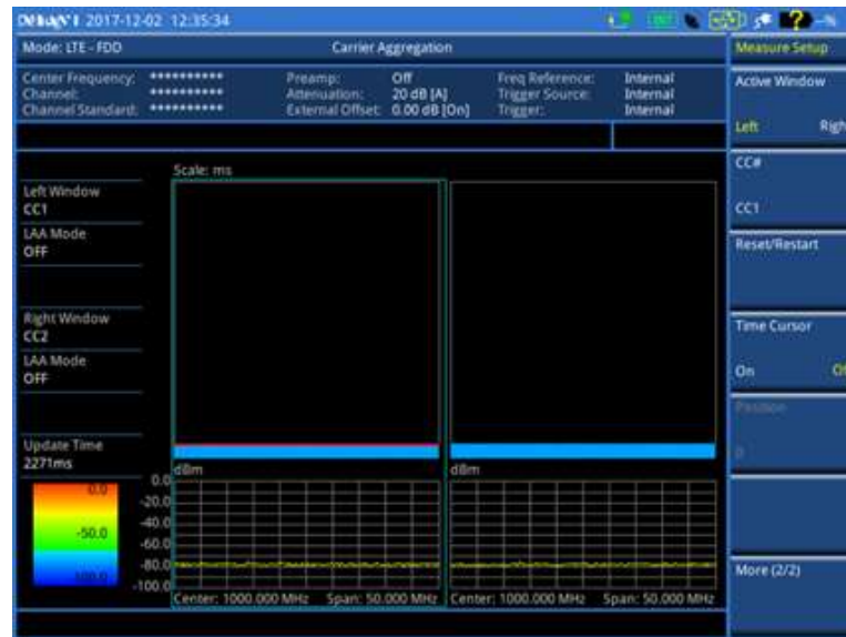
Figure 142 Carrier aggregation measurement with LTE-FDD signal analyzer (Dual Sp)
