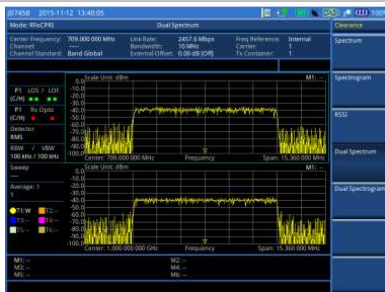
Figure 399 Example of dual spectrum analysis in BBU emulation
