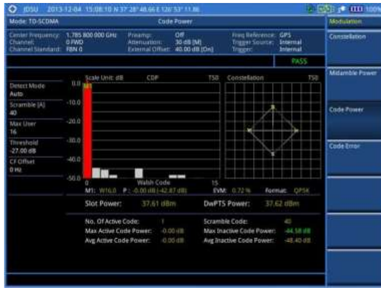
Figure 270 Code power measurement with TD-SCDMA signal analyzer
