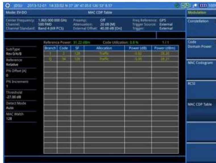
Figure 245 MAC CDP Table measurement with EV-DO signal analyzer
