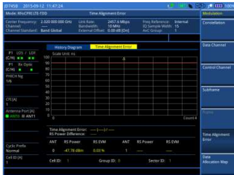
Figure 383 Time alignment error measurement with RFoCPRI LTE-TDD signal analyzer
