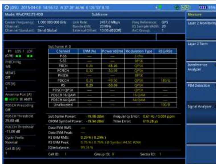
Figure 369 Subframe measurement (regular view) with RFoCPRI LTE-FDD signal analyzer
