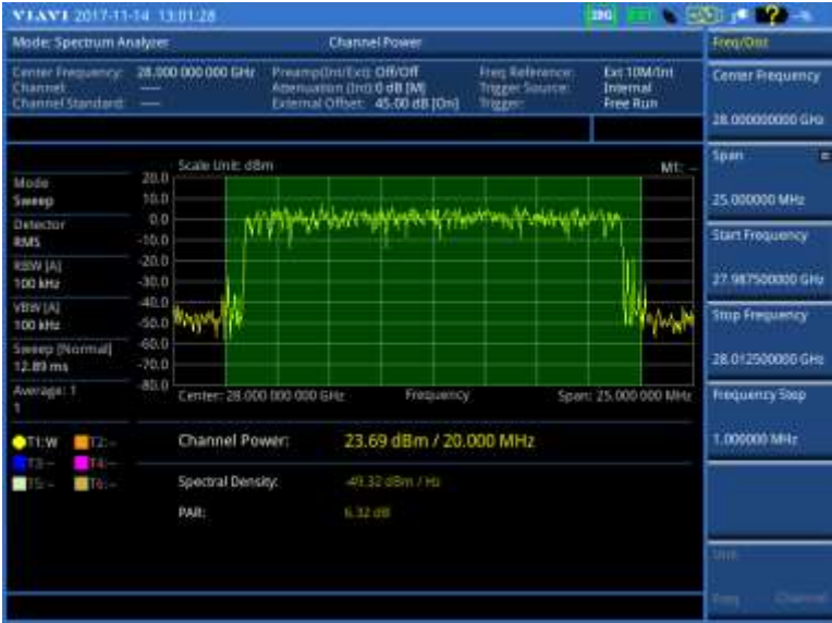
Figure 22 Channel power measurement with spectrum analyzer (on 28 GHz downconverter)
