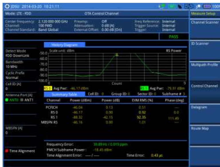
Figure 146 Control channel measurement with LTE-FDD OTA signal analyzer
