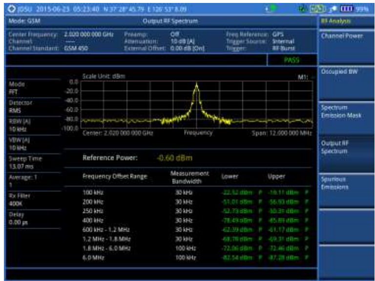
Figure 71 Output RF spectrum measurement with GSM signal analyzer
