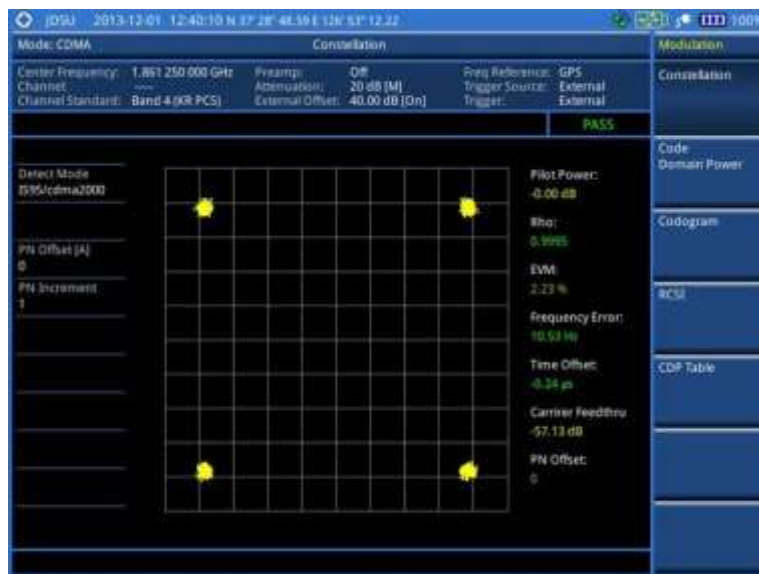
Figure 216 Constellation measurement with CDMA signal analyzer
