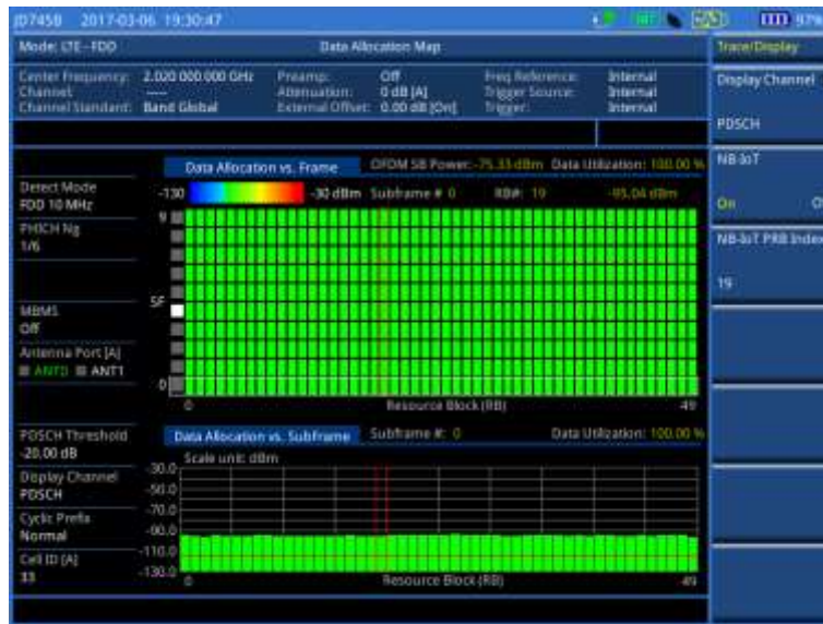
Figure 136 Data allocation map measurement with LTE-FDD signal analyzer (NB-IoT On)
