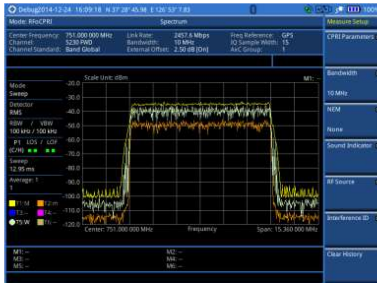
Figure 346 RFoCPRI spectrum analysis on LTE Uplink 10 MHz, antenna 1
