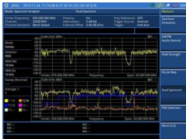
Figure 40 Dual spectrum measurement with spectrum analyzer
