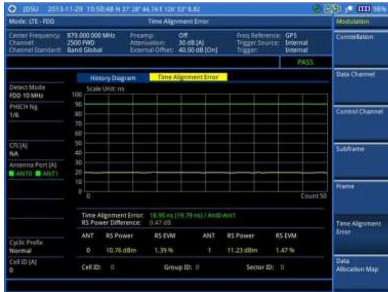
Figure 133 Time alignment error measurement with LTE-FDD signal analyzer
