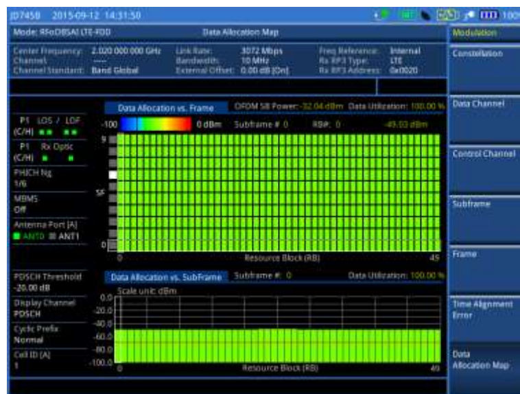
Figure 435 Data allocation map measurement with RFoOBSAI LTE-FDD signal analyzer
