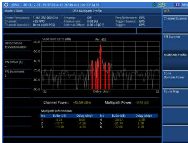
Figure 224 Multipath profile measurement with CDMA OTA signal analyzer
