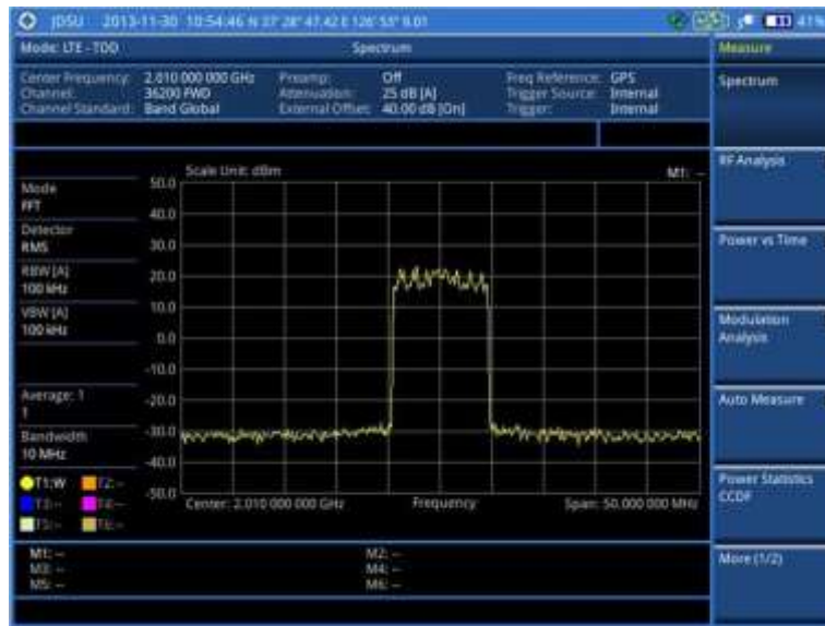
Figure 164 Spectrum measurement screen with LTE-TDD signal analyzer
