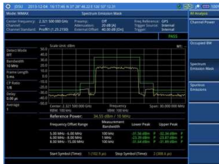
Figure 285 SEM measurement with Mobile WiMAX signal analyzer
