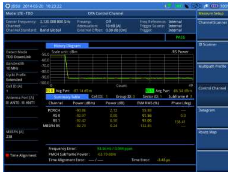
Figure 193 Control channel measurement with LTE-TDD OTA signal analyzer
