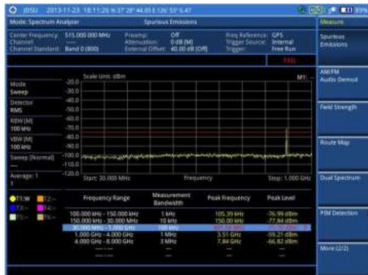
Figure 32 Spurious emissions measurement with spectrum analyzer
