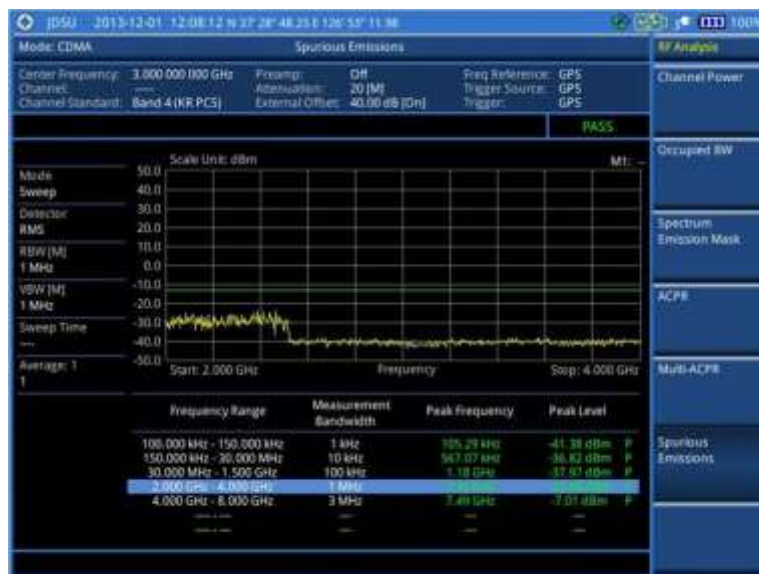
Figure 215 Spurious emissions measurement with CDMA signal analyzer
