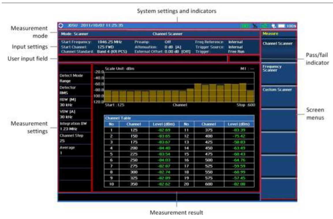
Figure 437 Channel scanner screen
