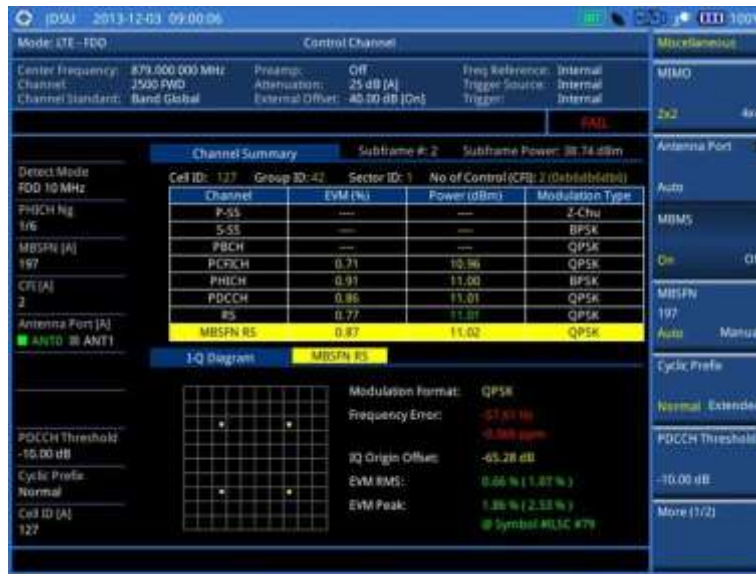
Figure 127 Control channel measurement with LTE-FDD signal analyzer (MBMS On)
