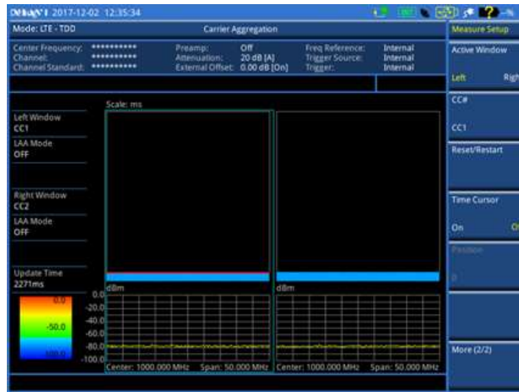
Figure 189 Carrier aggregation measurement with LTE-TDD signal analyzer (Dual Sp)
