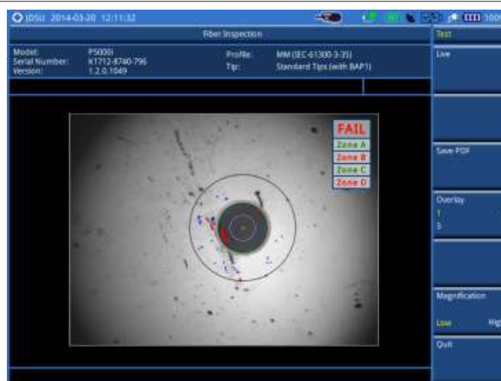
Figure 454 Analyzed fiber image and fiber inspection result
