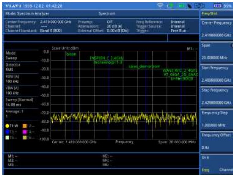
Figure 20 Wi-Fi SSID display with spectrum analyzer
