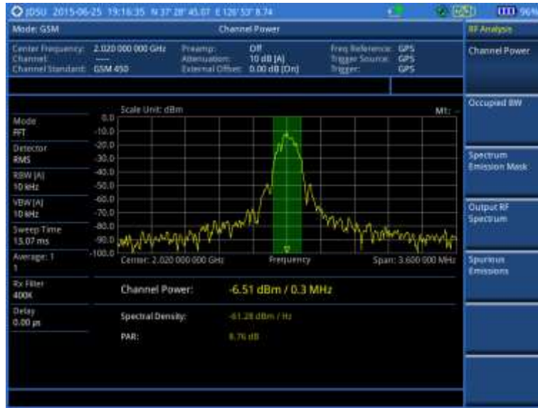
Figure 68 Channel power measurement with GSM signal analyzer
