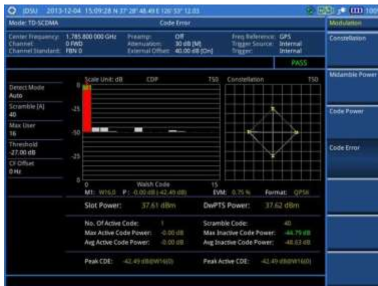
Figure 271 Code error measurement with TD-SCDMA signal analyzer
