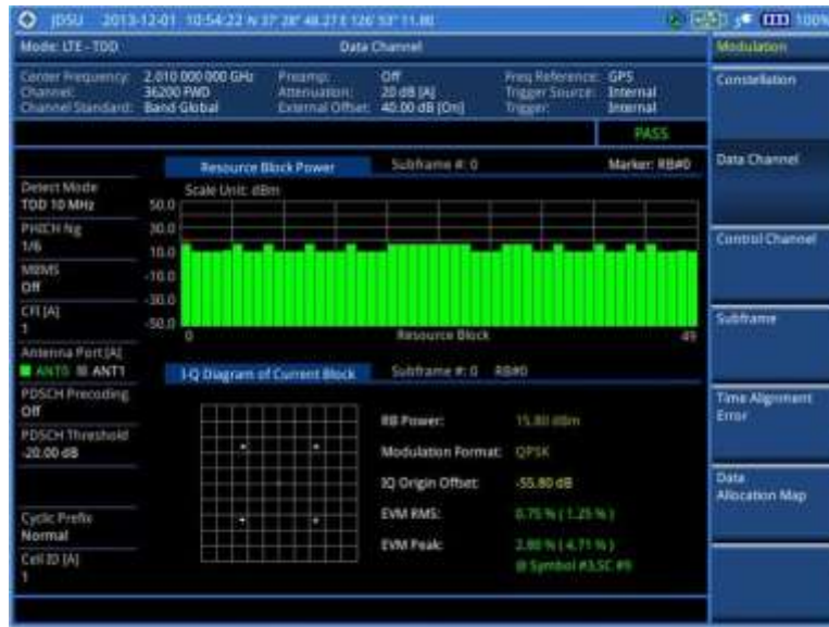
Figure 176 Data channel measurement with LTE-TDD signal analyzer (MBMS On)
