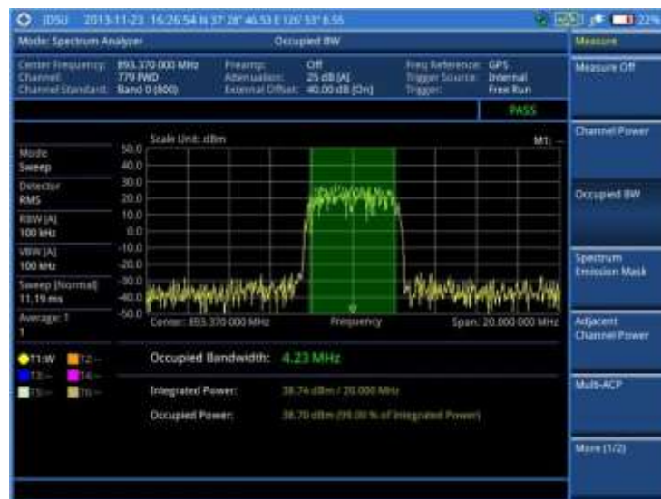
Figure 25 Occupied bandwidth measurement with spectrum analyzer (on 28 GHz downconverter)
