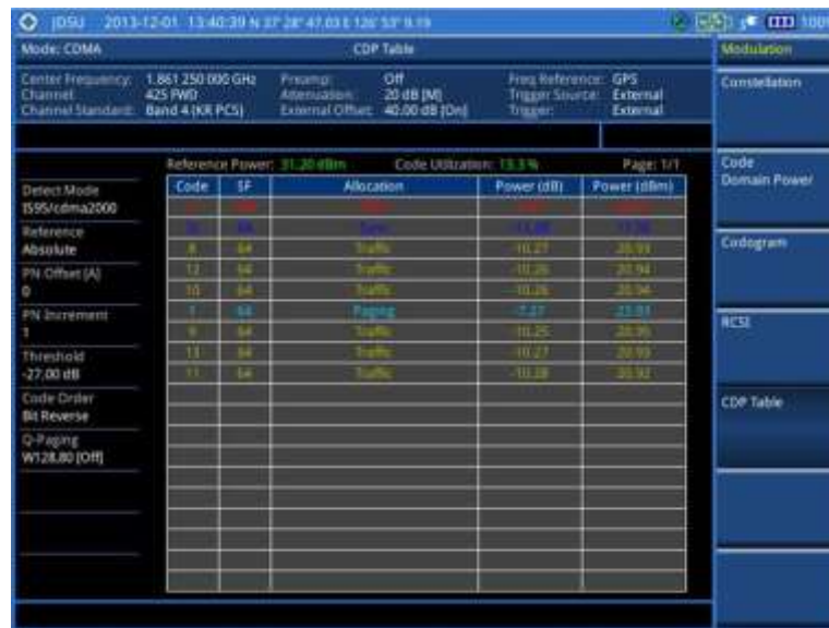
Figure 220 CDP Table measurement with CDMA signal analyzer
