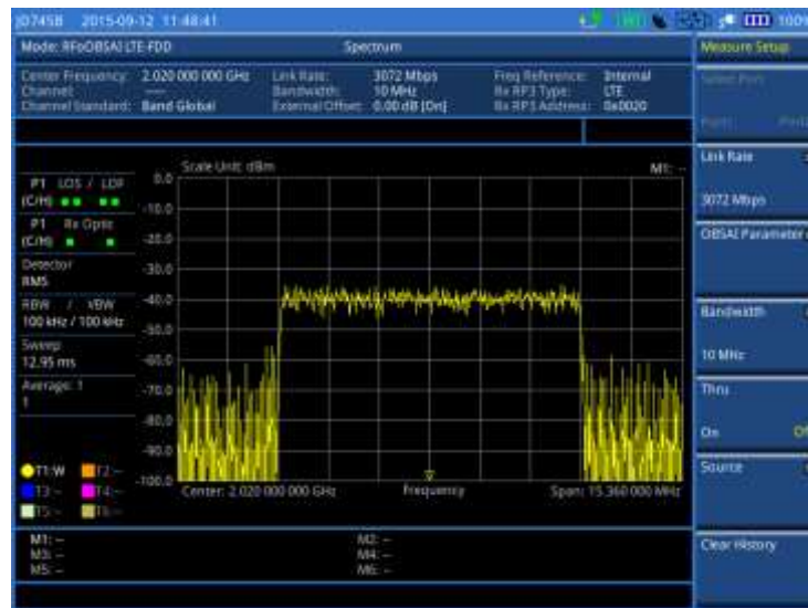
Figure 425 Spectrum measurement with RFoBSAI LTE-FDD signal analyzer
