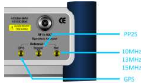
Figure 281 Connection ports for external reference clock
