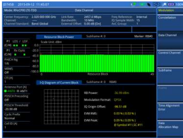
Figure 380 Data channel measurement with RFoCPRI LTE-FDD signal analyzer
