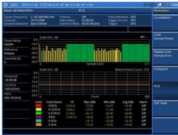
Figure 98 RCSI measurement with WCDMA/HSPA+ signal analyzer
