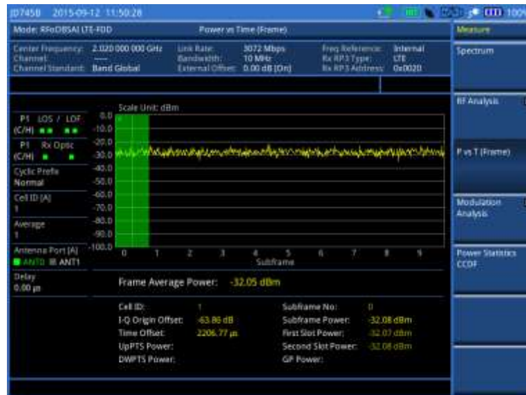
Figure 428 Power vs. time (frame) measurement with RFoOBSAI LTE-FDD signal analyzer
