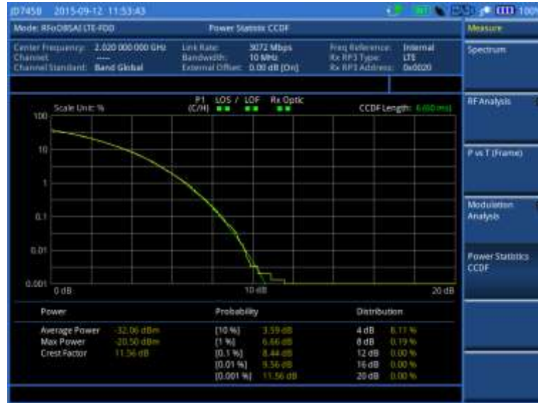
Figure 436 CCDF measurement with RFoBSAI LTE-FDD signal analyzer
