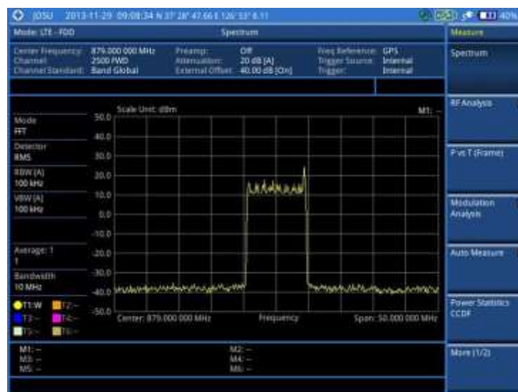
Figure 113 Spectrum measurement screen with LTE-FDD signal analyzer
