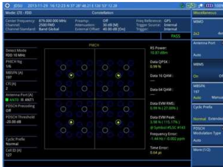
Figure 122 Constellation measurement with LTE-FDD signal analyzer (MBMS On)
