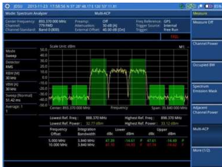
Figure 30 Multi-ACP measurement with spectrum analyzer
