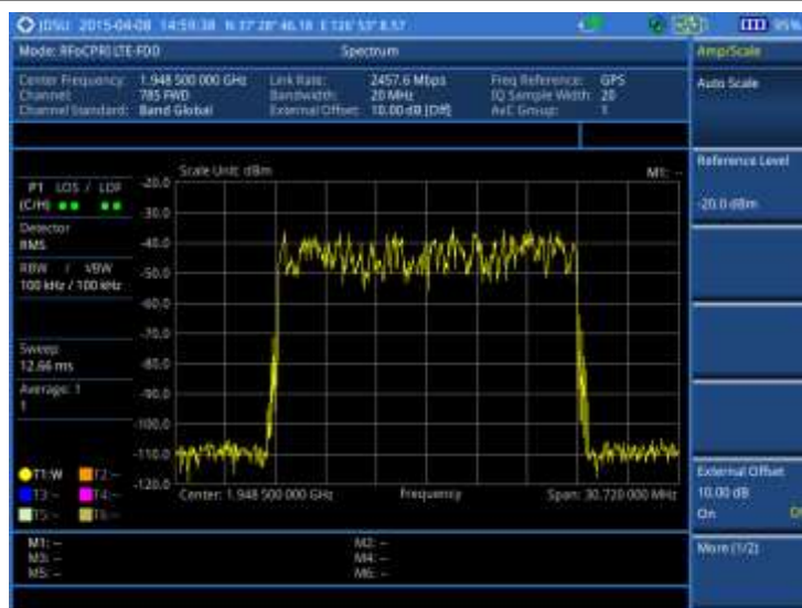
Figure 362 Spectrum measurement with RFoCPRI LTE-FDD signal analyzer
