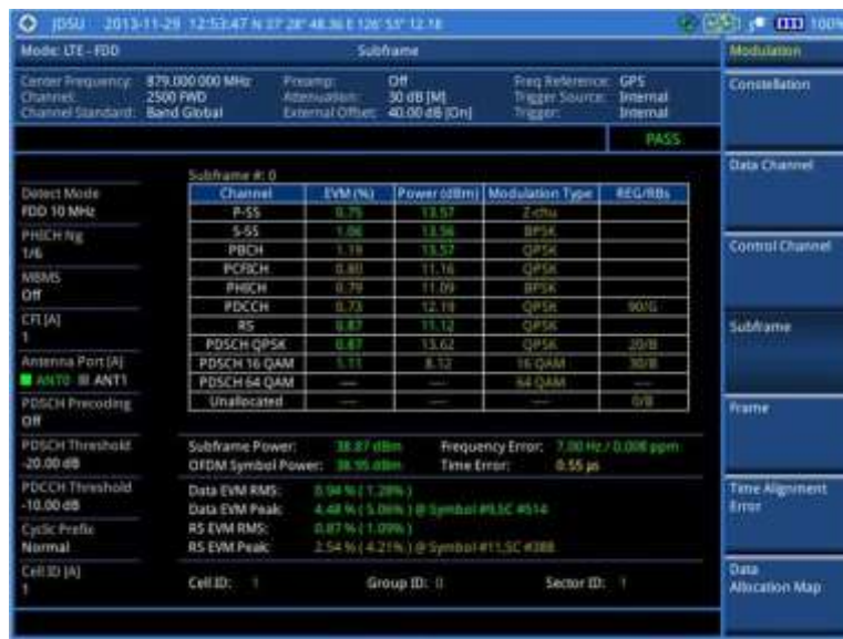
Figure 129 Subframe measurement with LTE-FDD signal analyzer (Chart On)
