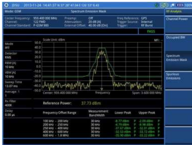
Figure 70 SEM measurement with GSM signal analyzer
