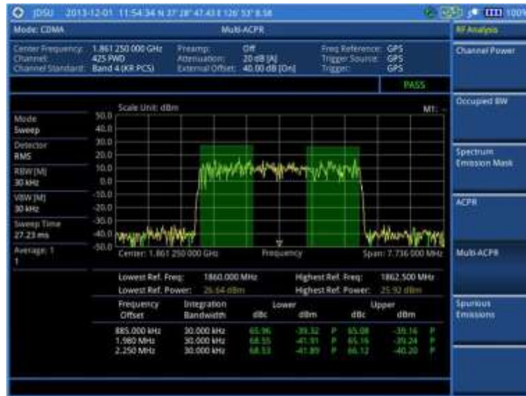
Figure 214 Multi-ACPR measurement with CDMA signal analyzer
