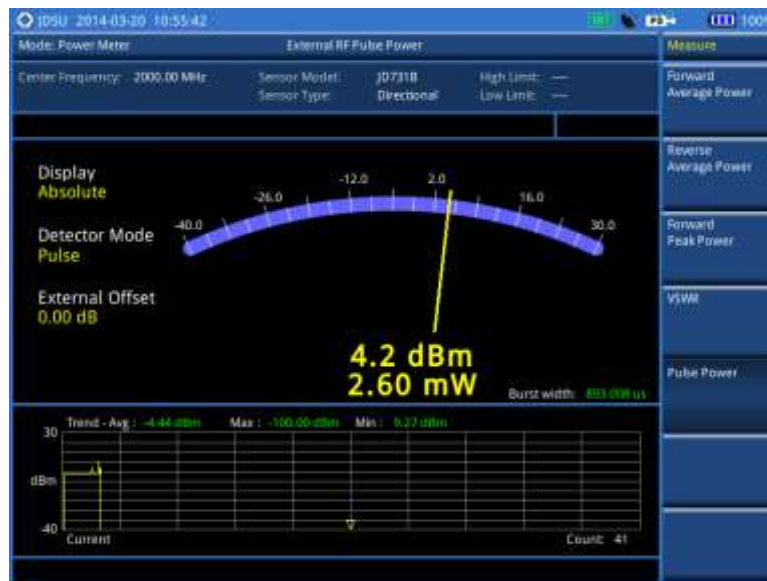
Figure 449 External power measurement of pulse power
