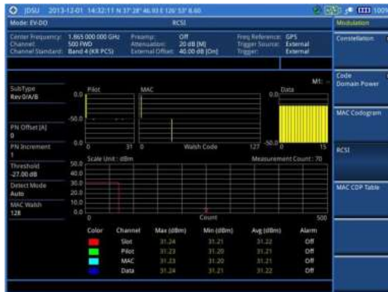
Figure 244 RCSI measurement with EV-DO signal analyzer
