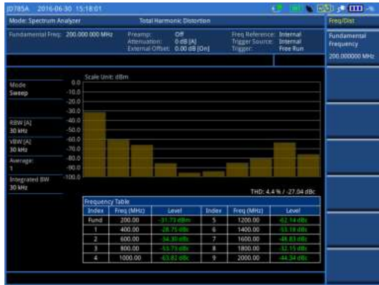
Figure 43 Total harmonic distortion screen
