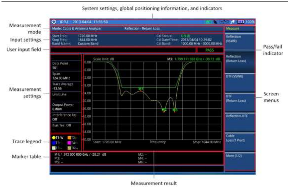
Figure 313 Reflection measurement screen
