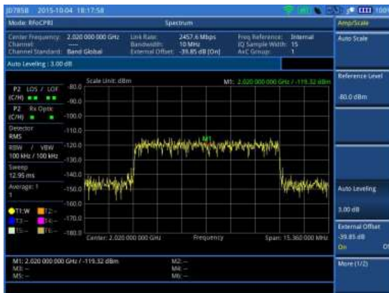
Figure 341 After enabling Auto Leveling
