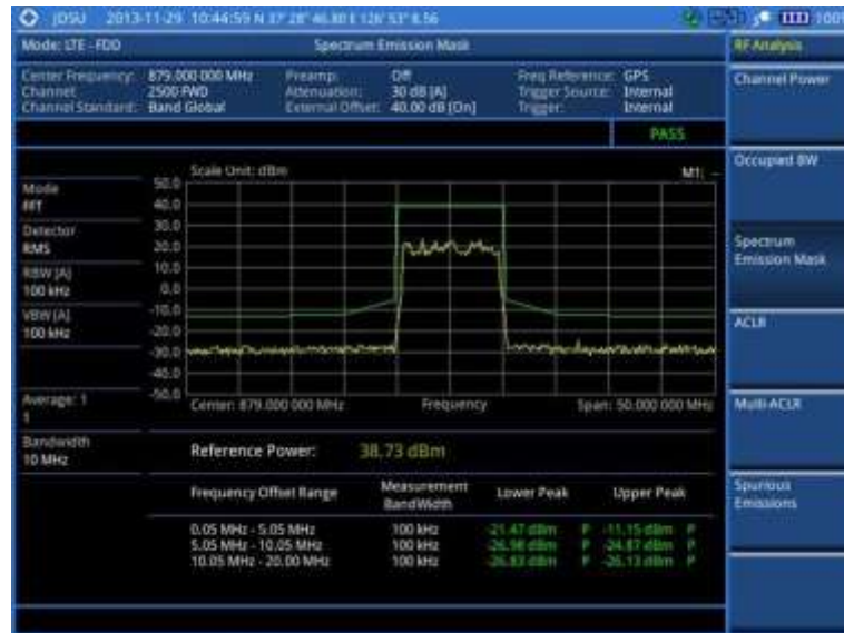
Figure 116 SEM measurement with LTE-FDD signal analyzer
