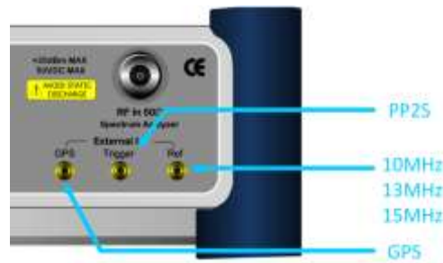
Figure 256 Connection ports for external reference clock
