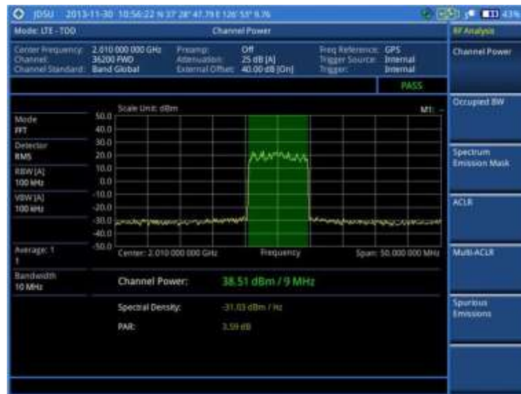
Figure 165 Channel power measurement with LTE-TDD signal analyzer
