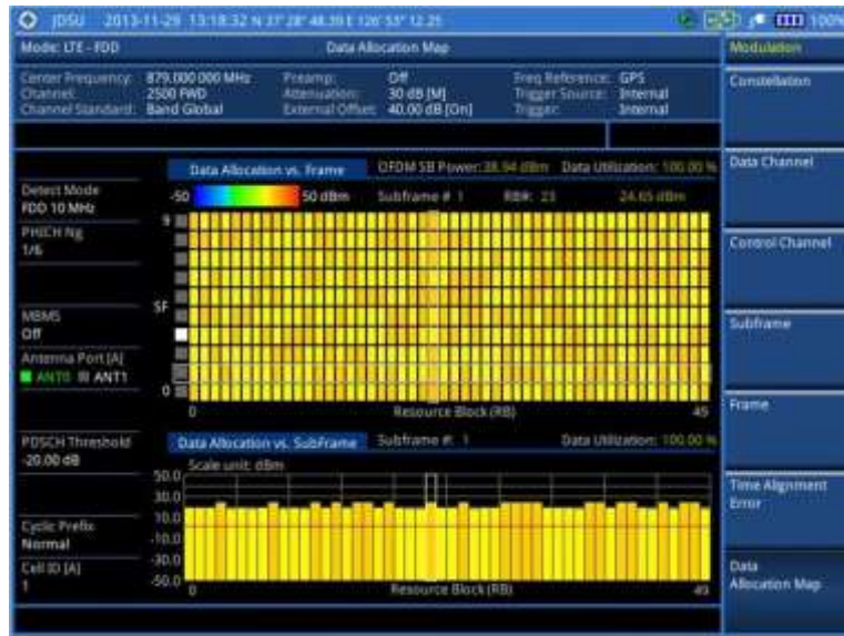
Figure 134 Data allocation map measurement with LTE-FDD signal analyzer
