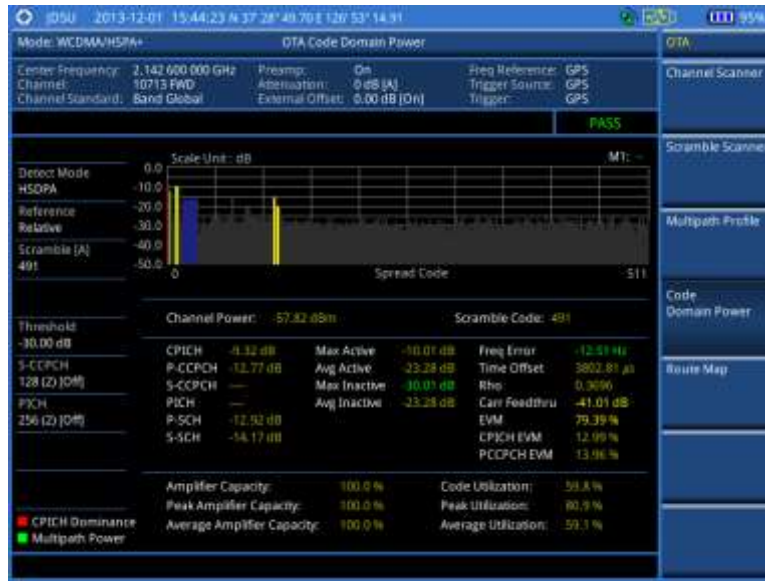
Figure 104 Code domain power measurement with WCDMA/HSPA+ OTA signal analyzer
