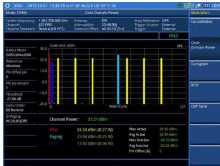
Figure 217 Code domain power measurement with CDMA signal analyzer
