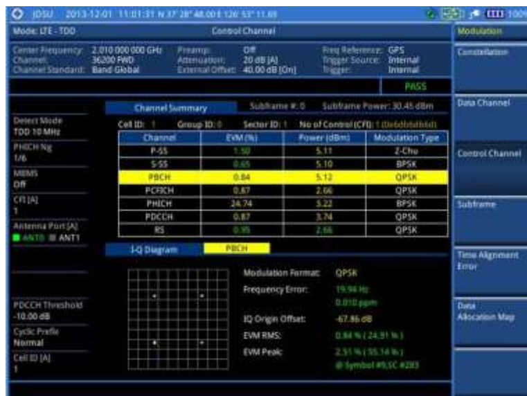
Figure 177 Control channel measurement with LTE-TDD signal analyzer
