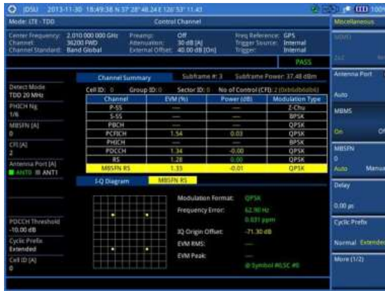
Figure 178 Control channel measurement with LTE-TDD signal analyzer (MBMS On)
