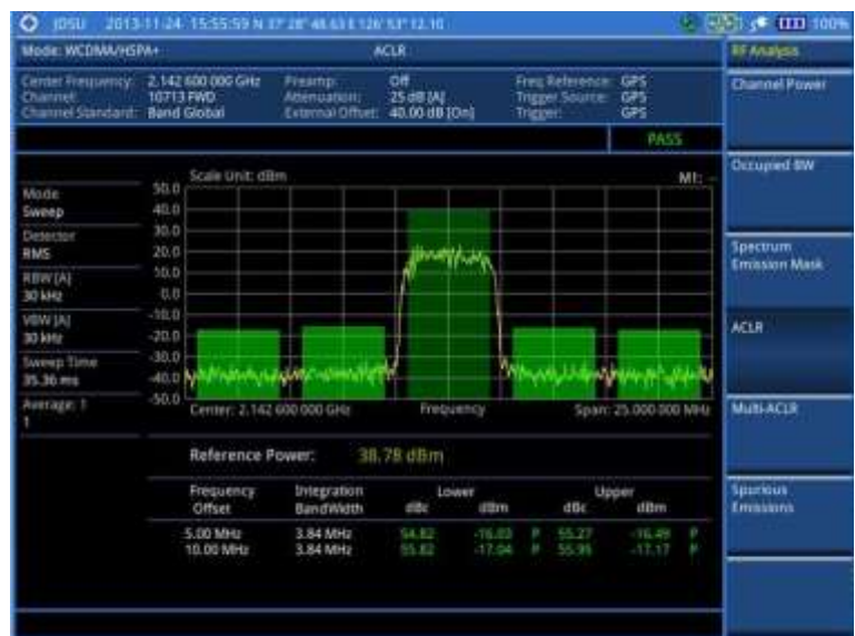
Figure 91 ACLR measurement with WCDMA/HSPA+ signal analyzer
