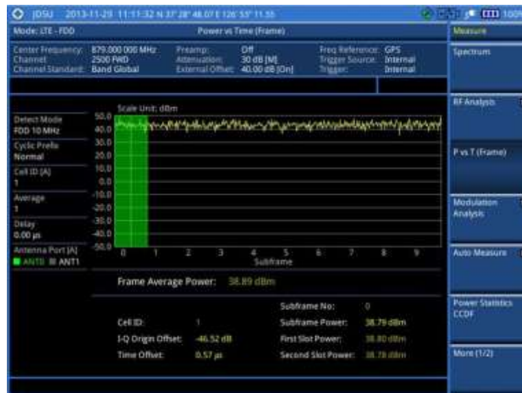
Figure 120 Power vs. time (frame) measurement with LTE – FDD signal analyzer
