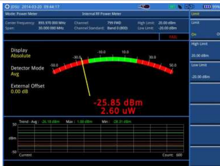
Figure 447 Internal power measurement
