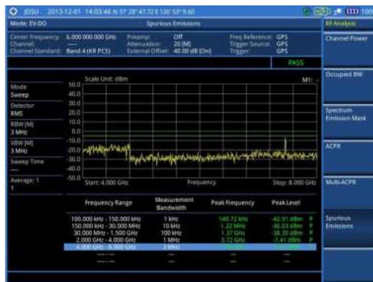
Figure 238 Spurious emissions measurement with EV-DO signal analyzer
