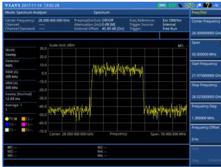
Figure 17 Spectrum measurement with spectrum analyzer (on 28 GHz downconverter)
