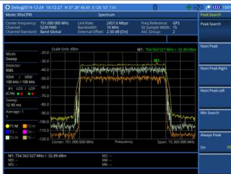
Figure 347 RFoCPRI spectrum analysis on LTE Uplink 10 MHz, antenna 2
