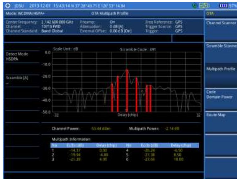
Figure 103 Multipath profile measurement with WCDMA/HSPA+ OTA signal analyzer
