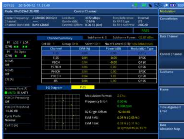
Figure 431 Control channel measurement with RFoOBSAI LTE-FDD signal analyzer
