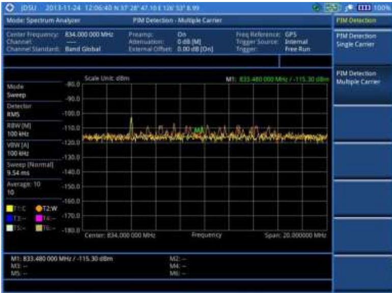
Figure 42 PIM detection for multiple carriers
