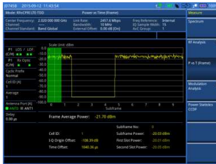
Figure 378 Power vs. time (frame) measurement with RFoCPRI LTE-TDD signal analyzer
