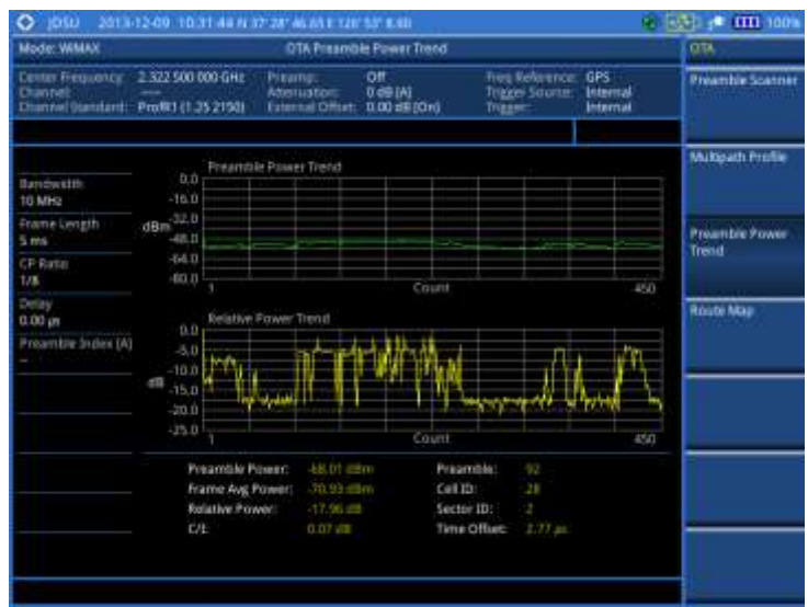
Figure 295 Preamble power trend with Mobile WiMAX OTA signal analyzer
