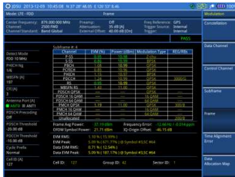
Figure 132 Frame measurement with LTE-FDD signal analyzer (MBMS On)
