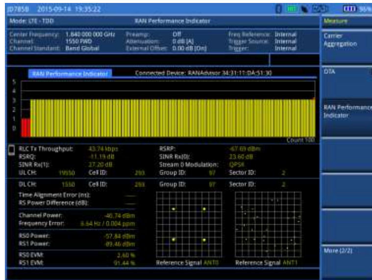
Figure 203 RAN performance indicator with LTE-TDD signal analyzer
