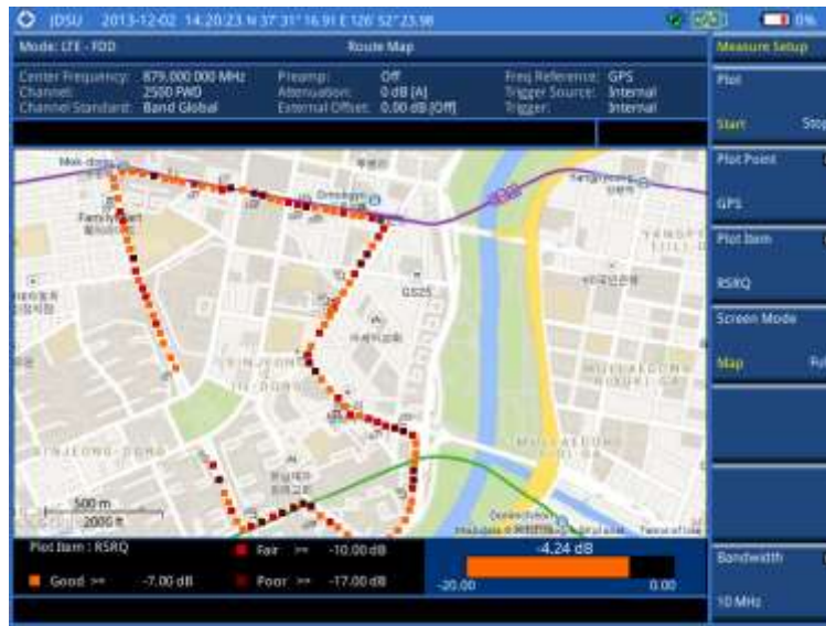
Figure 150 Route map measurement (RS-SINR) with LTE-FDD OTA signal analyzer
