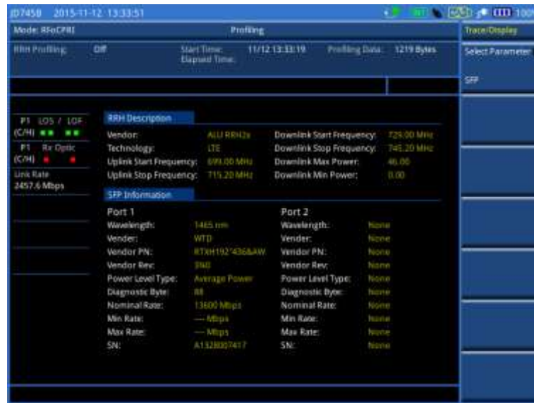
Figure 390 Example of RRH profiling results with SFP information
