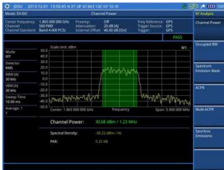
Figure 233 Channel power measurement with EV-DO signal analyzer
