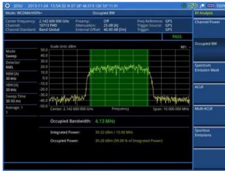
Figure 89 Occupied bandwidth measurement with WCDMA/HSPA+ signal analyzer
