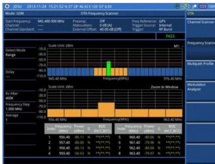
Figure 79 Frequency scanner measurement with GSM OTA signal analyzer
