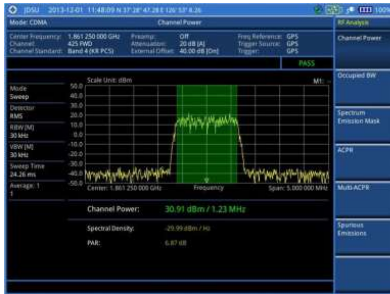
Figure 210 Channel power measurement with CDMA signal analyzer
