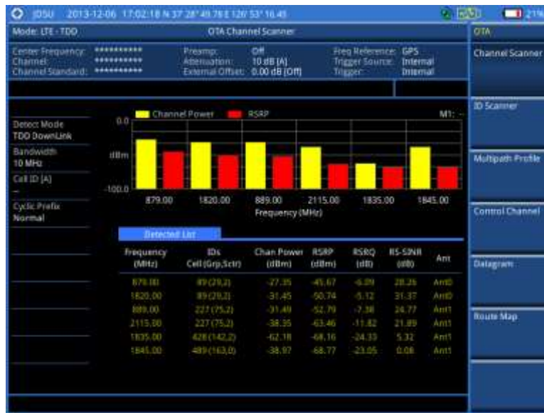
Figure 190 Channel scanner measurement with LTE-TDD OTA signal analyzer
