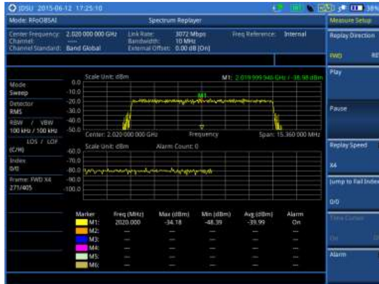
Figure 421 RFoBSAI spectrum replay
