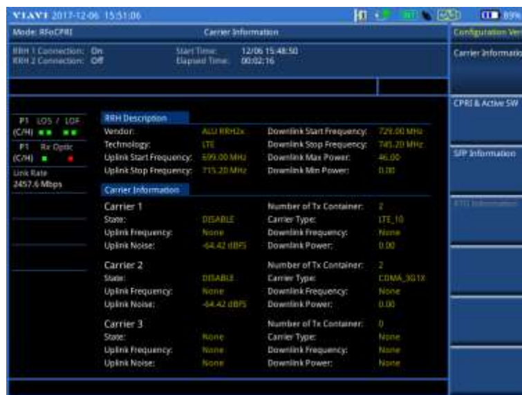
Figure 392 Example of verification of carrier configuration
