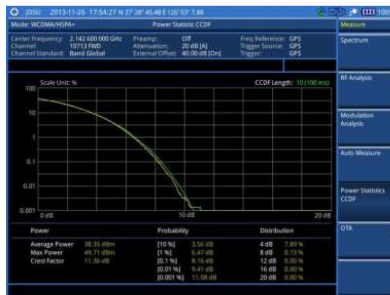
Figure 100 CCDF measurement with WCDMA/HSPA+ signal analyzer
