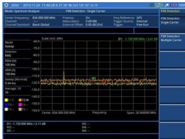
Figure 41 PIM detection for single carrier
