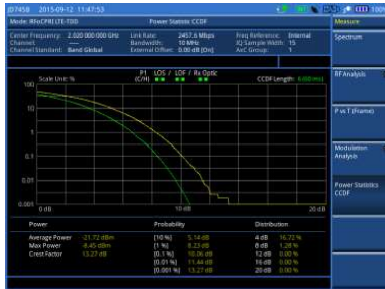
Figure 385 CCDF measurement with RFoCPRI LTE-TDD signal analyzer
