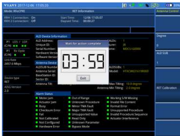
Figure 411 Example of RET calibration in RET information
