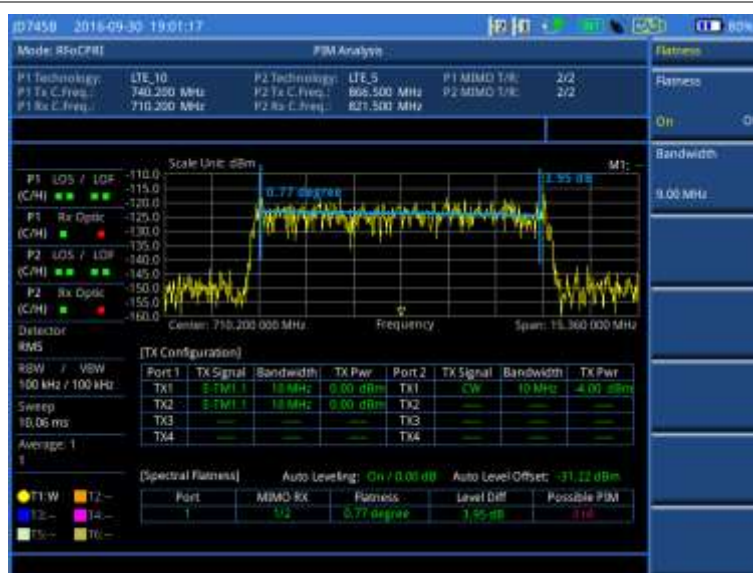
Figure 406 Example of Wideband Mode PIM analysis in BBU emulation
