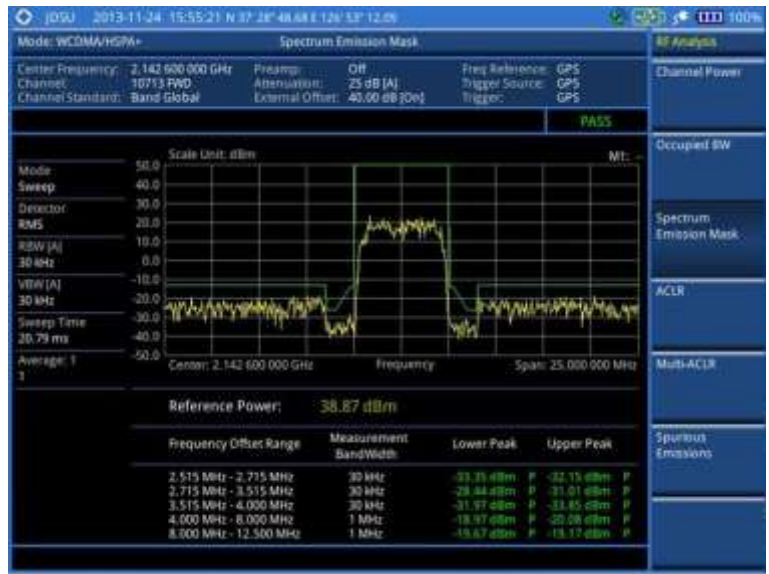
Figure 90 SEM measurement with WCDMA/HSPA+ signal analyzer
