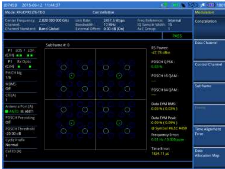
Figure 379 Constellation measurement with RFoCPRI LTE-TDD signal analyzer
