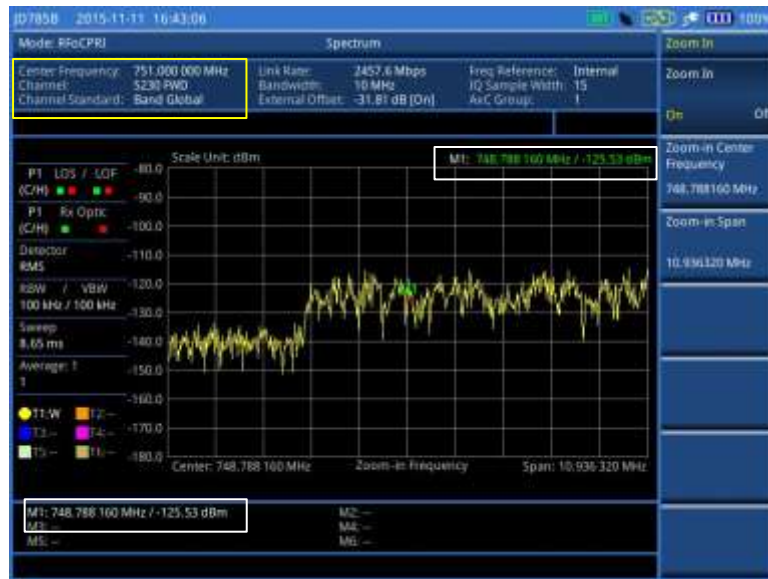
Figure 356 Zoomed-in spectrum view in RFoCPRI interference analyzer
