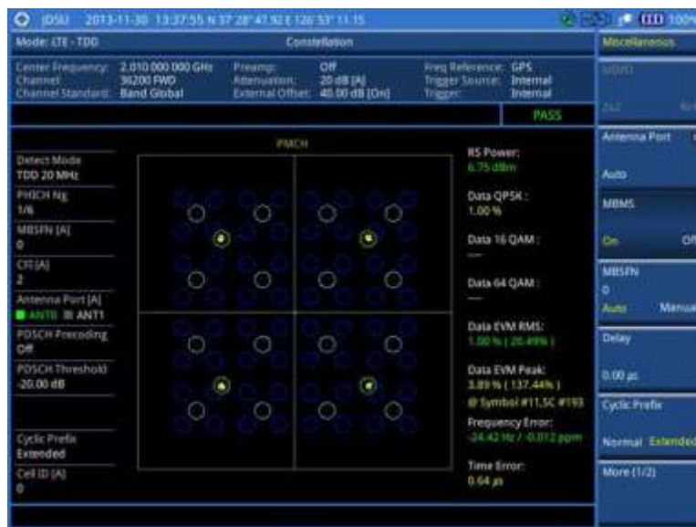
Figure 174 Constellation measurement with LTE-TDD signal analyzer (MBMS On)
