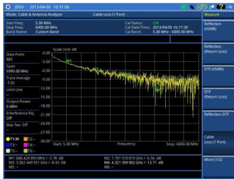
Figure 329 Cable loss (1 port) measurement
