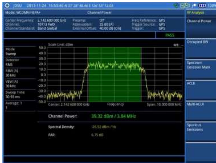
Figure 88 Channel power measurement with WCDMA/HSPA+ signal analyzer
