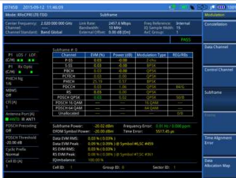
Figure 382 Subframe measurement (regular view) with RFoCPRI LTE-TDD signal analyzer
