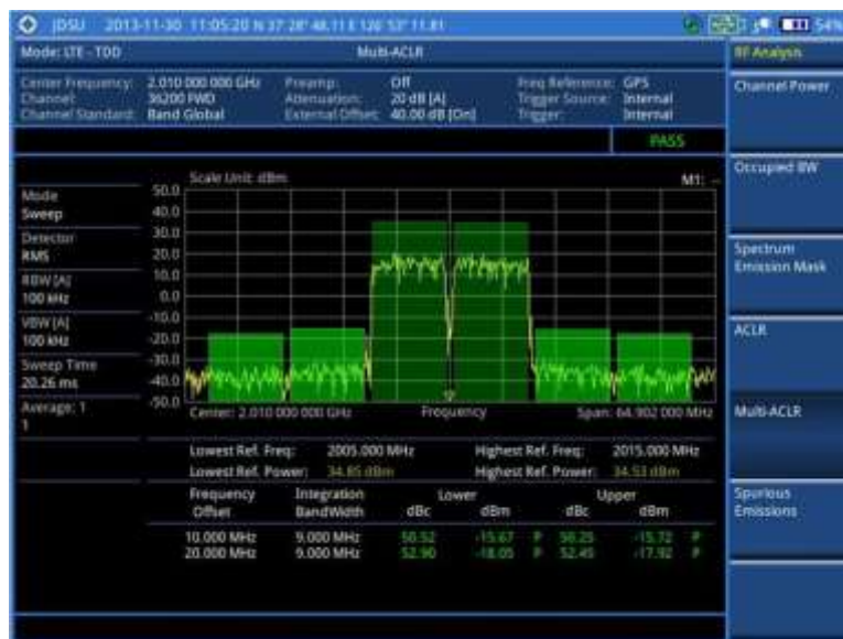
Figure 169 Multi-ACLR measurement with LTE-TDD signal analyzer
