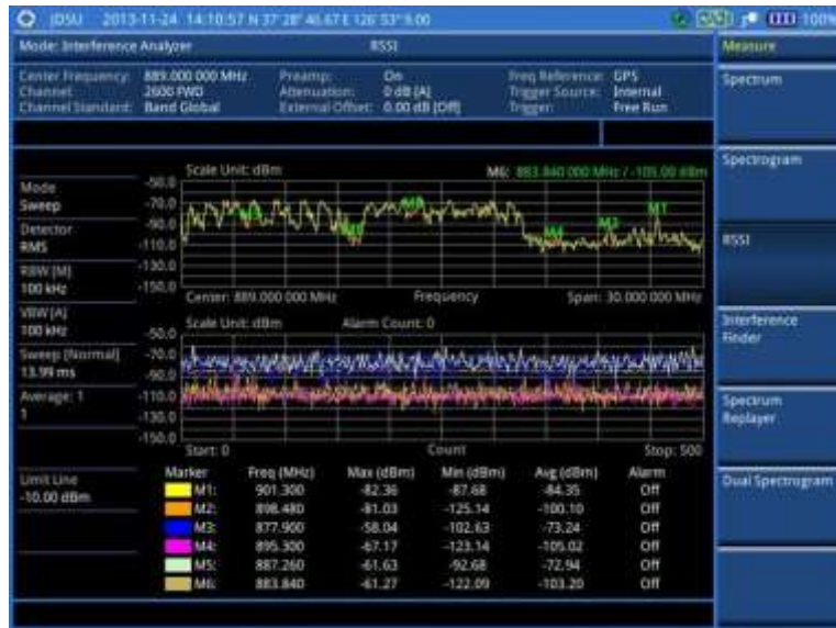
Figure 54 Interference measurement in RSSI (on 28 GHz downconverter)
