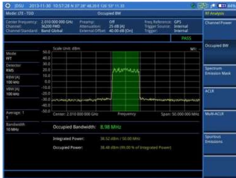
Figure 166 Occupied bandwidth measurement with LTE-TDD signal analyzer
