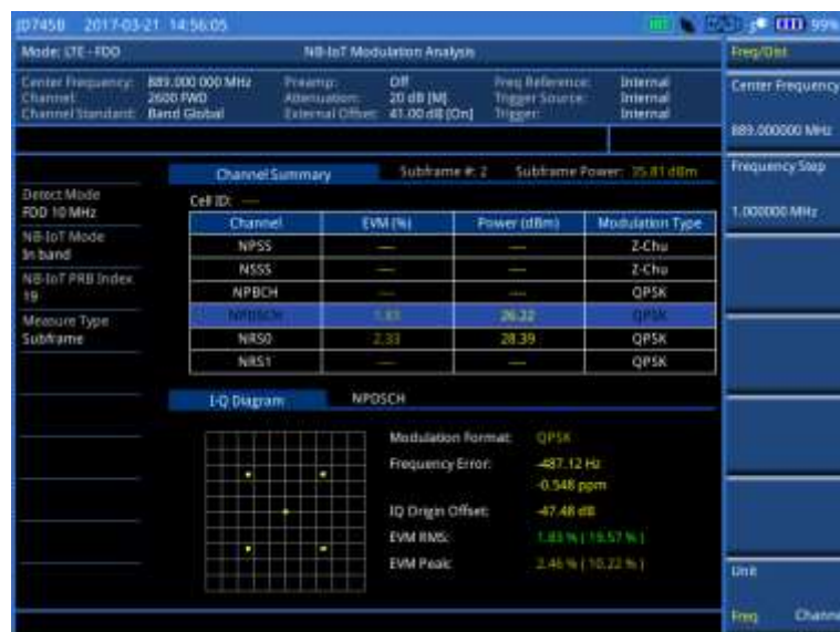
Figure 158 NB-IoT modulation measurement with LTE-FDD signal analyzer (Subframe 2)
