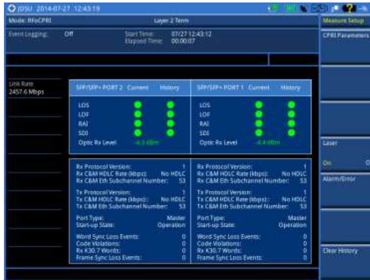
Figure 338 CPRI layer 2 term test
