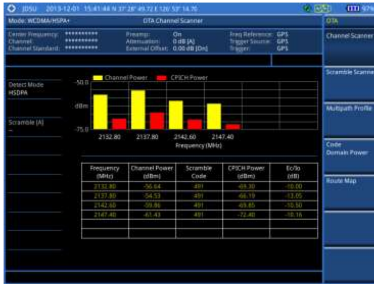
Figure 101 Channel scanner measurement with WCDMA/HSPA+ OTA signal analyzer
