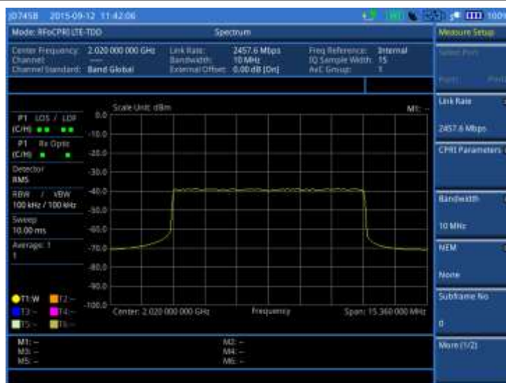
Figure 375 Spectrum measurement with RFoCPRI LTE-TDD signal analyzer
