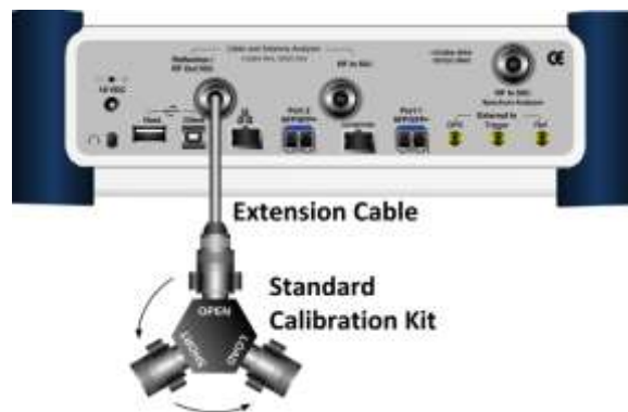
Figure 314 1-port calibration connection with mechanical Y-Cal kit
