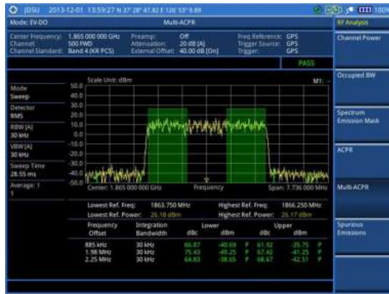
Figure 237 Multi-ACPR measurement with EV-DO signal analyzer
