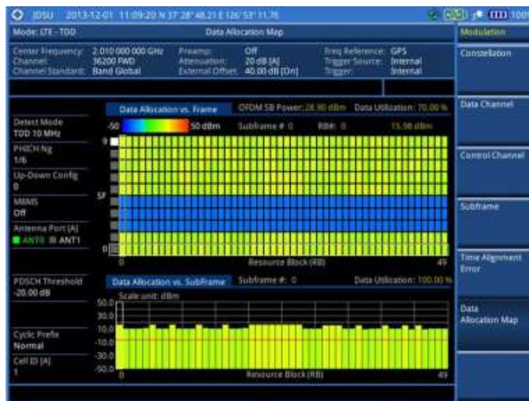
Figure 183 Data allocation map measurement with LTE-TDD signal analyzer
