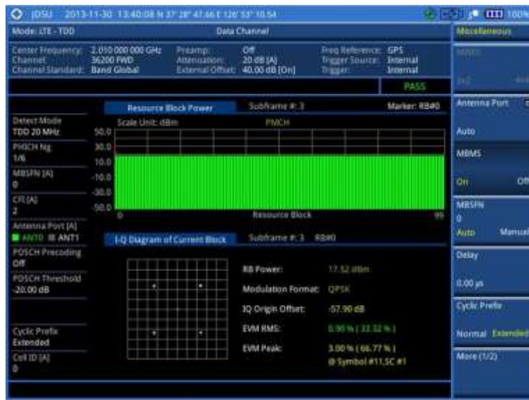
Figure 176 Data channel measurement with LTE-TDD signal analyzer (MBMS On)
