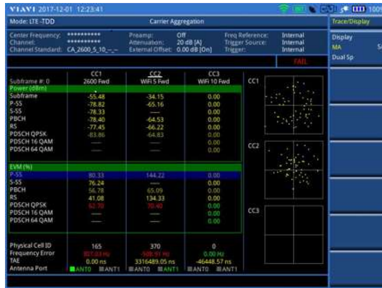
Figure 188 Carrier aggregation measurement with LTE-TDD signal analyzer (SA with Wi-Fi on)
