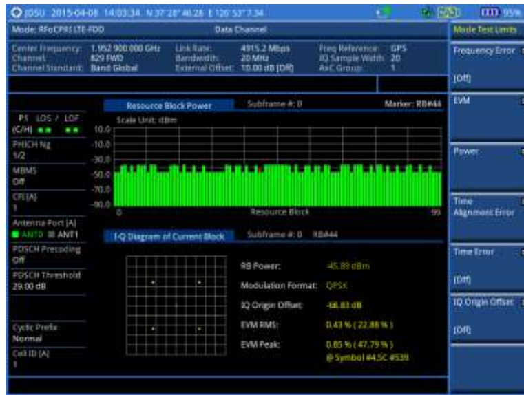
Figure 367 Data channel measurement with RFoCPRI LTE-FDD signal analyzer
