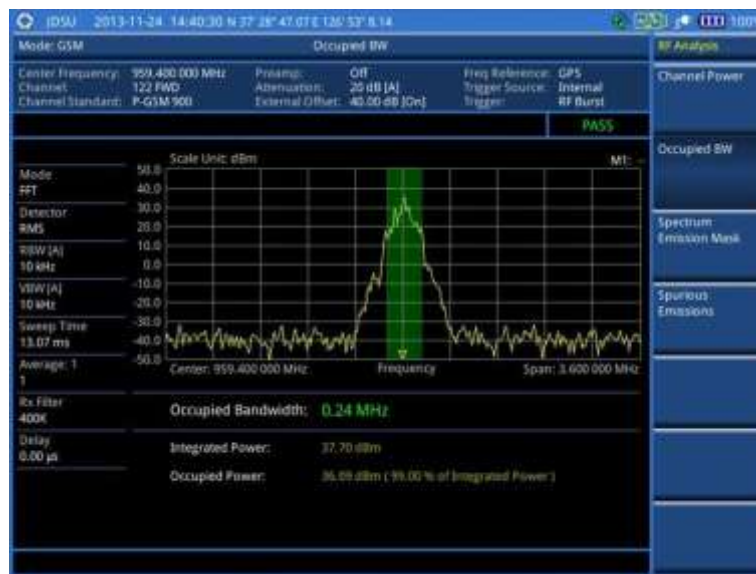
Figure 69 Occupied bandwidth measurement with GSM signal analyzer
