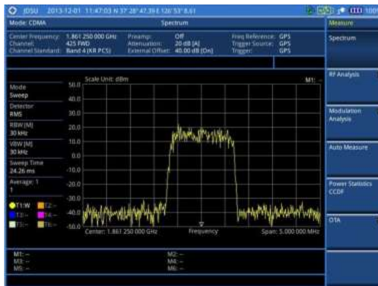
Figure 209 Spectrum measurement screen with CDMA signal analyzer
