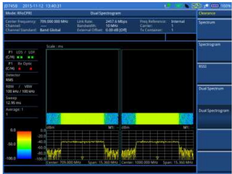
Figure 401 Example of dual spectrogram analysis in BBU emulation
