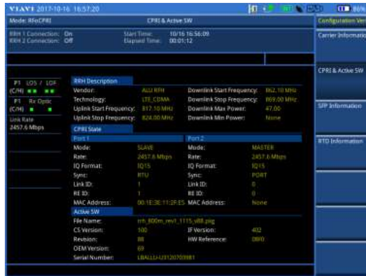
Figure 393 Example of verification of CPRI state and active software
