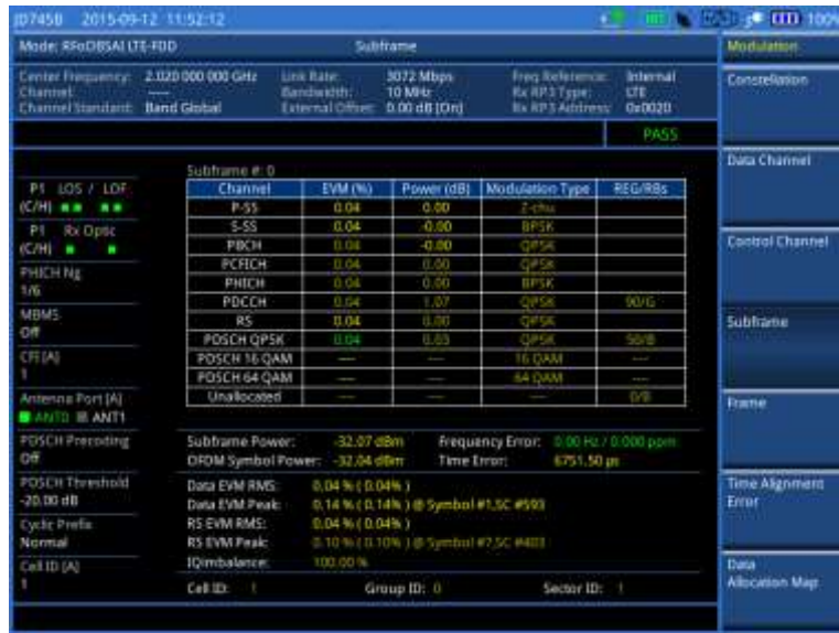
Figure 432 Subframe measurement with RFoOBSAI LTE-FDD signal analyzer
