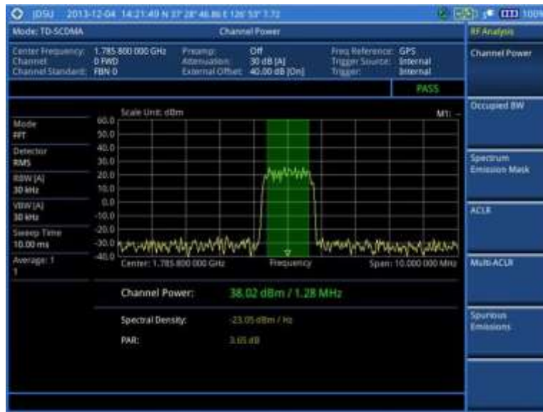
Figure 258 Channel power measurement with TD-SCDMA signal analyzer
