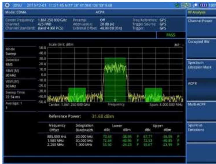
Figure 213 ACPR measurement with CDMA signal analyzer
