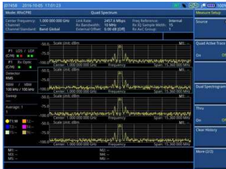
Figure 352 RFoCPRI quad spectrum with quad active trace on
