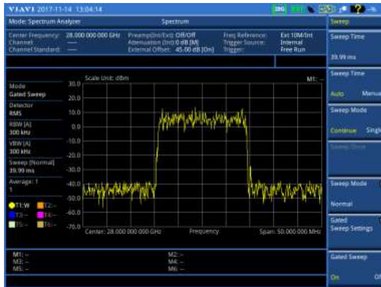
Figure 19 Gated sweep measurement with spectrum analyzer (on 28 GHz downconverter)
