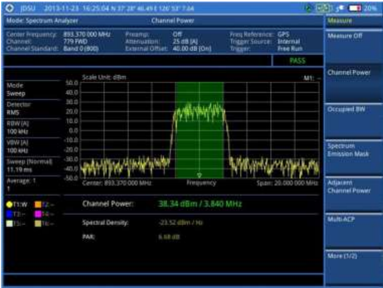
Figure 21 Channel power measurement with spectrum analyzer
