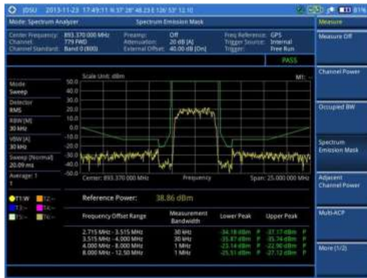
Figure 27 Spectrum emission mask measurement with spectrum analyzer (on 28 GHz downconverter)
