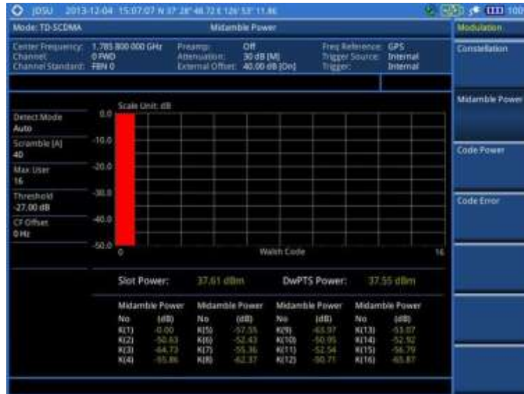
Figure 269 Midamble measurement with TD-SCDMA signal analyzer
