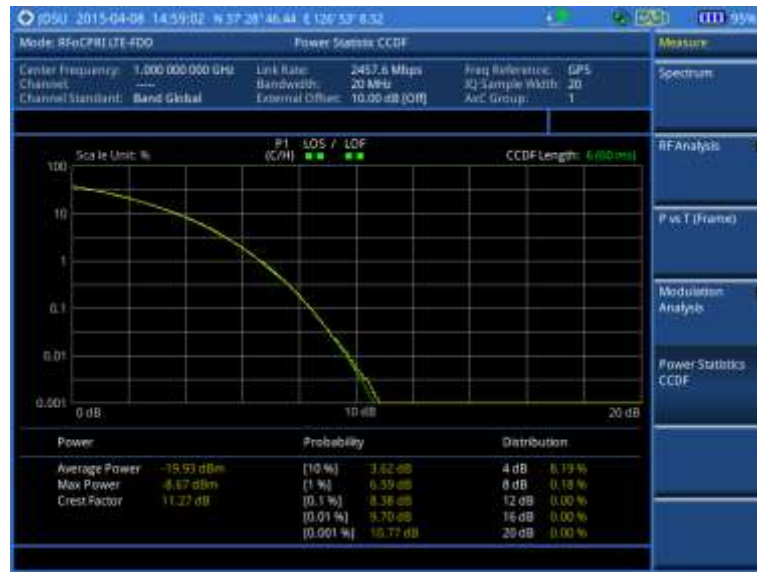
Figure 373 CCDF measurement with RFoCPRI LTE-FDD signal analyzer
