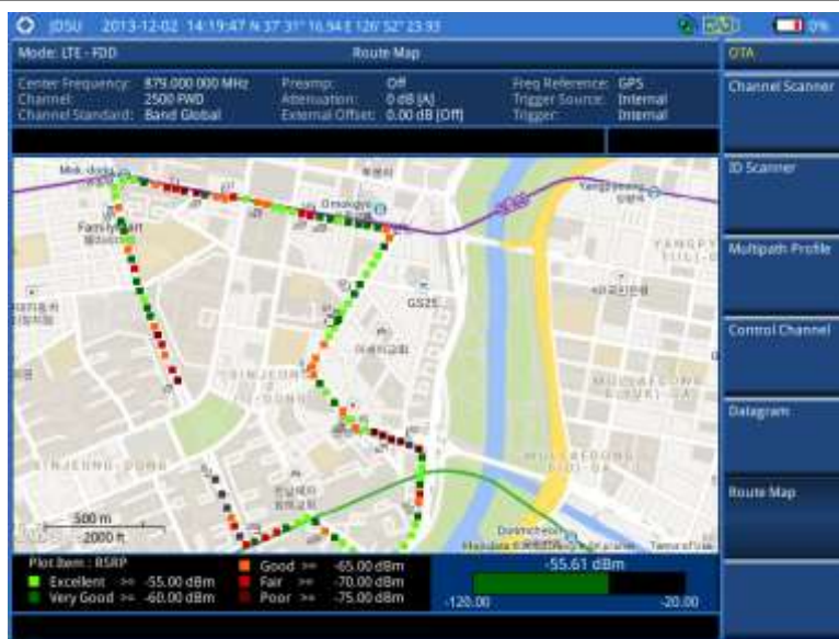
Figure 148 Route map measurement (RSRP) with LTE-FDD OTA signal analyzer
