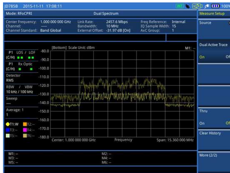
Figure 350 RFoCPRI dual spectrum with dual active trace on
