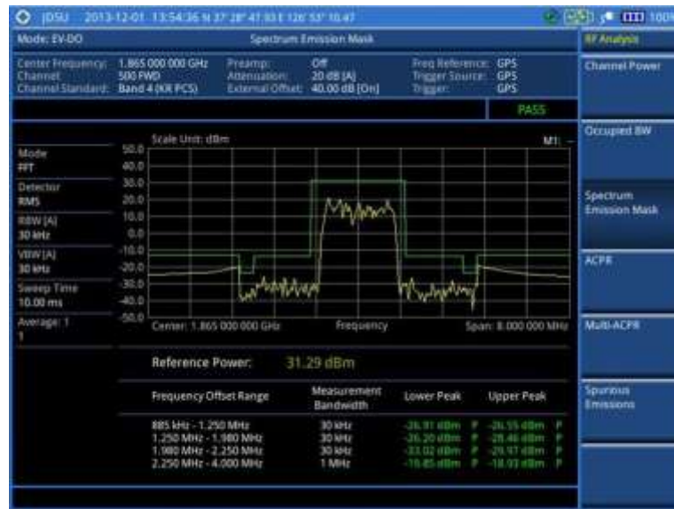
Figure 235 SEM measurement with EV-DO signal analyzer
