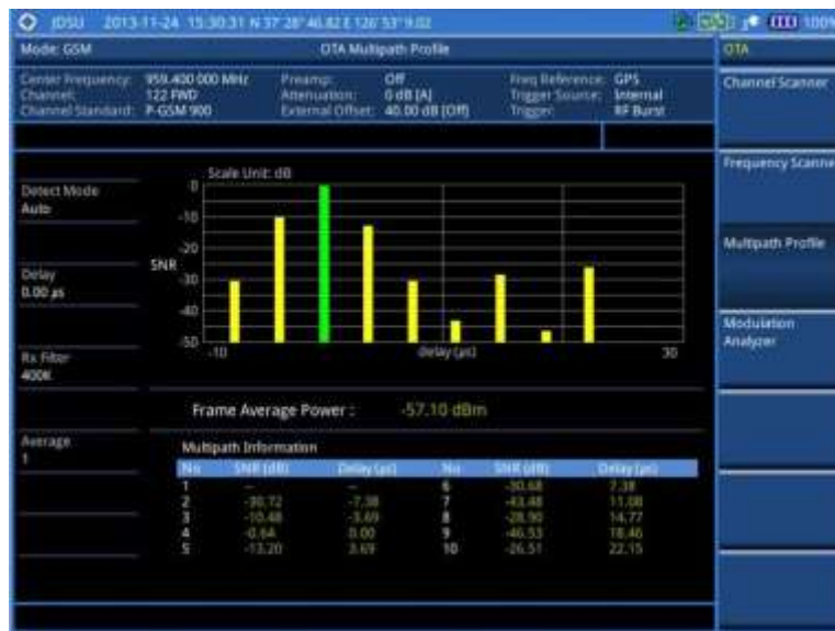
Figure 80 Multipath profile measurement with GSM OTA signal analyzer
