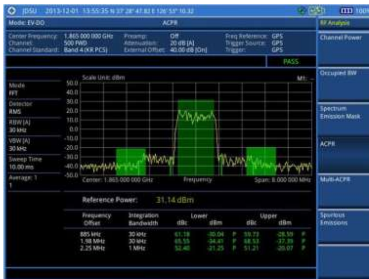
Figure 236 ACPR measurement with EV-DO signal analyzer
