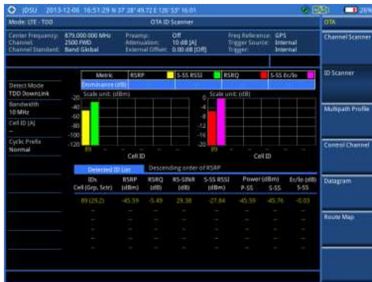
Figure 191 ID scanner measurement with LTE-TDD OTA signal analyzer
