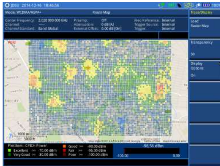
Figure 107 Raster image overlaid on the base map in WCDMA/HSPA+ OTA signal analyzer
