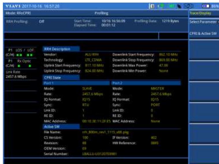
Figure 389 Example of RRH profiling results with CPRI state and activated SW
