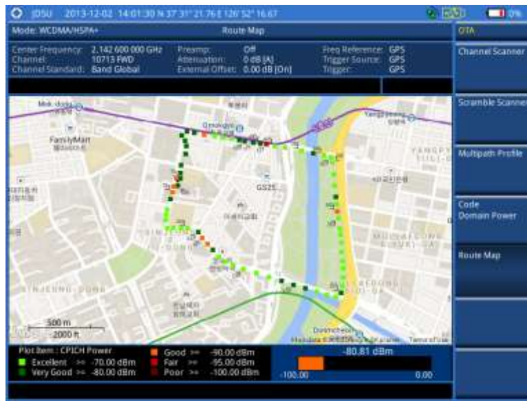
Figure 106 Route map measurement (CPICH Ec/Io) with WCDMA/HSPA+ OTA signal analyzer
