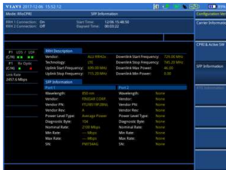
Figure 394 Example of verification of SFP information
