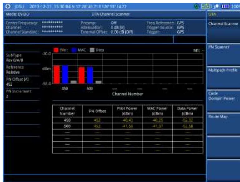
Figure 247 Channel scanner measurement with EV-DO OTA signal analyzer
