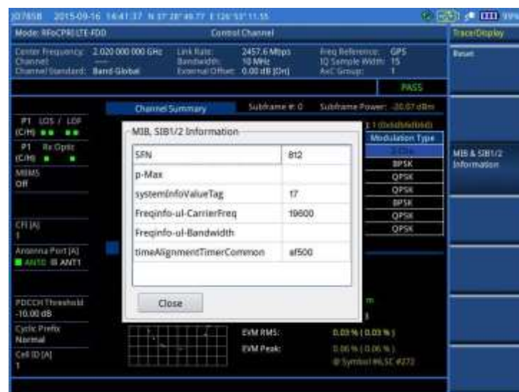
Figure 361 Decoded MIB & SIB1/2 information in RFoCPRI LTE-FDD signal analyzer
