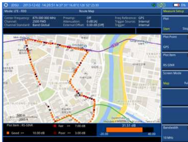
Figure 150 Route map measurement (RS-SINR) with LTE-FDD OTA signal analyzer
