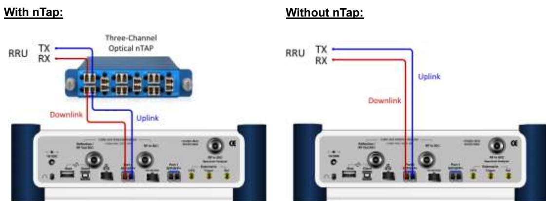
Figure 415 Connection diagram for Layer-2 term testing mode
