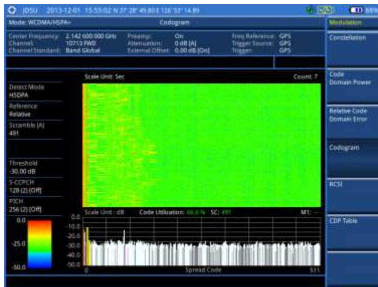
Figure 97 Codogram in full view with WCDMA/HSPA+ signal analyzer
