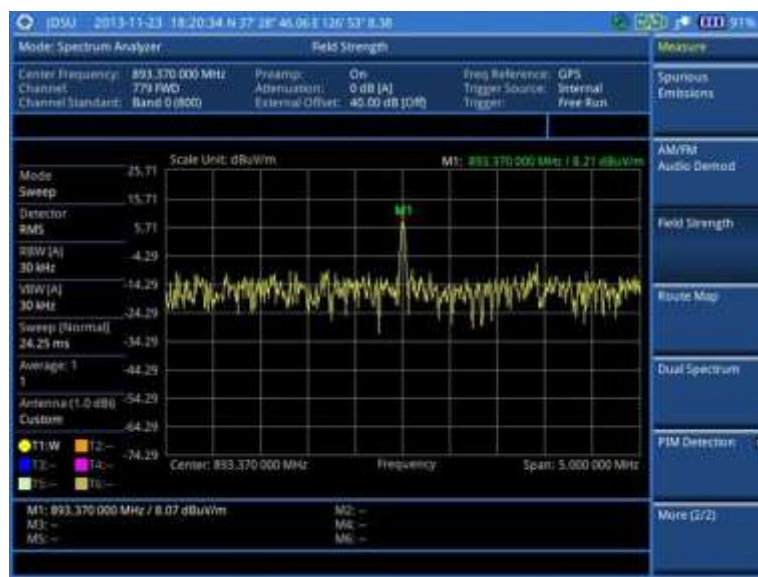
Figure 37 Field strength measurement with spectrum analyzer (on 28 GHz downconverter)
