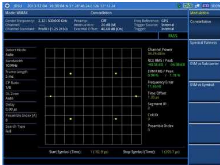
Figure 288 Constellation measurement with Mobile WiMAX signal analyzer
