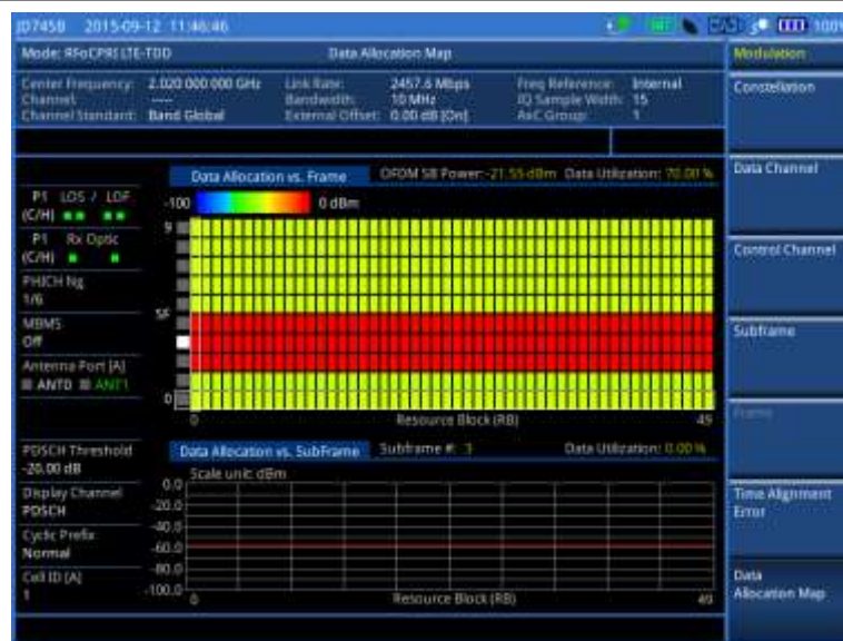
Figure 384 Data allocation map measurement with RFoCPRI LTE-TDD signal analyzer
