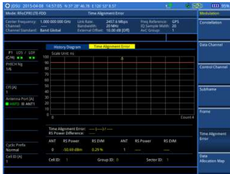
Figure 371 Time alignment error measurement with RFoCPRI LTE-FDD signal analyzer
