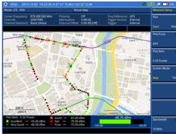
Figure 153 Route map measurement (S-SS Power) with LTE-FDD OTA signal analyzer
