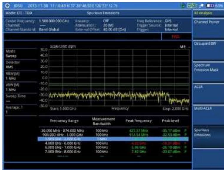
Figure 170 Spurious emissions measurement with LTE-TDD signal analyzer
