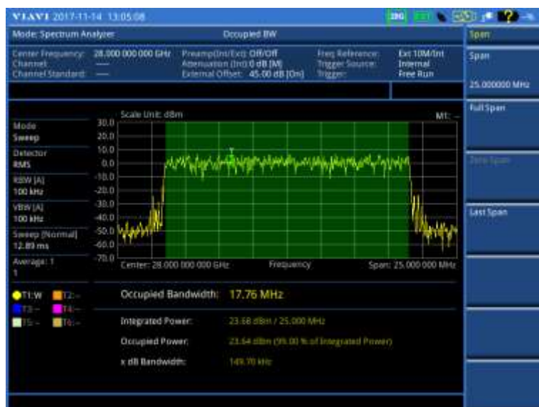
Figure 25 Occupied bandwidth measurement with spectrum analyzer (on 28 GHz downconverter)
