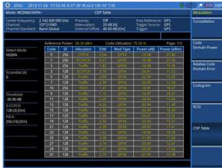
Figure 99 CDP Table measurement with WCDMA/HSPA+ signal analyzer
