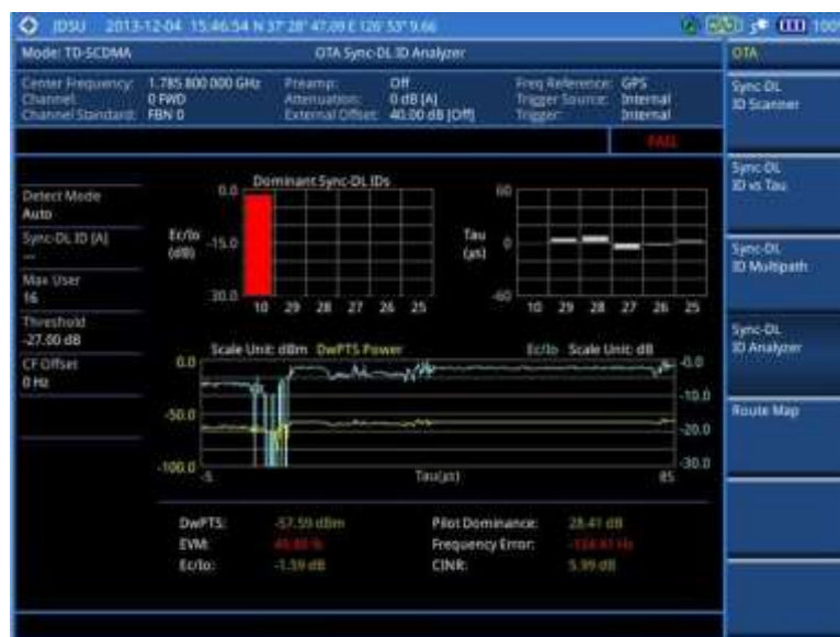
Figure 275 Sync-DL ID analyzer measurement with TD-SCDMA OTA signal analyzer
