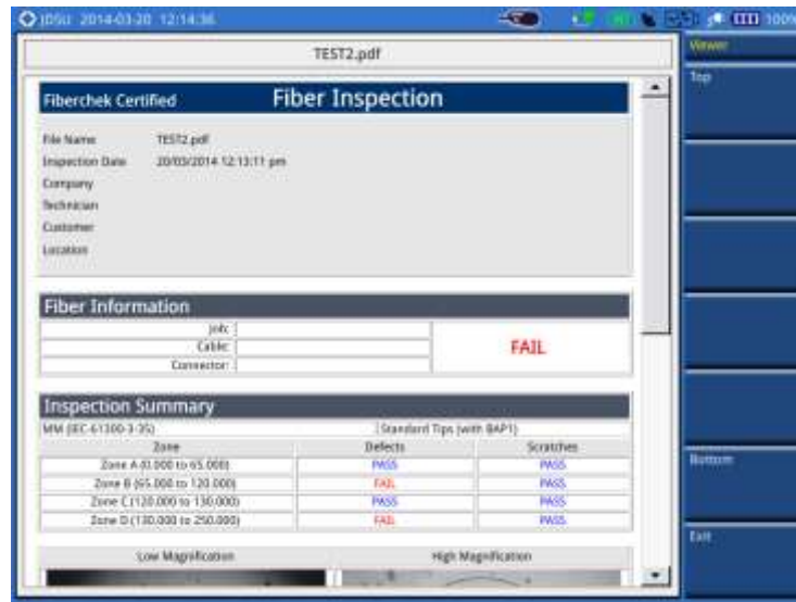
Figure 455 Fiber inspection report
