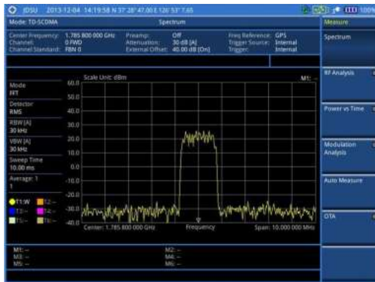
Figure 257 Spectrum measurement screen with TD-SCDMA signal analyzer
