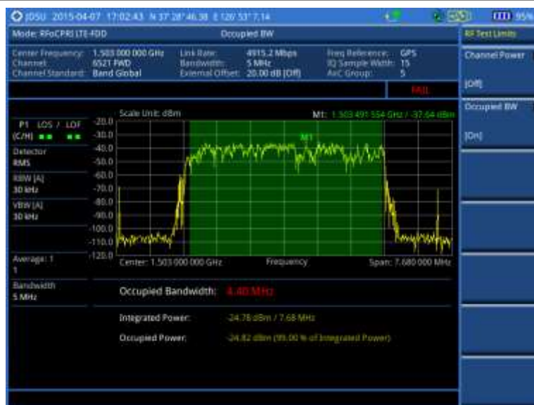
Figure 364 Occupied bandwidth measurement with RFoCPRI LTE-FDD signal analyzer
