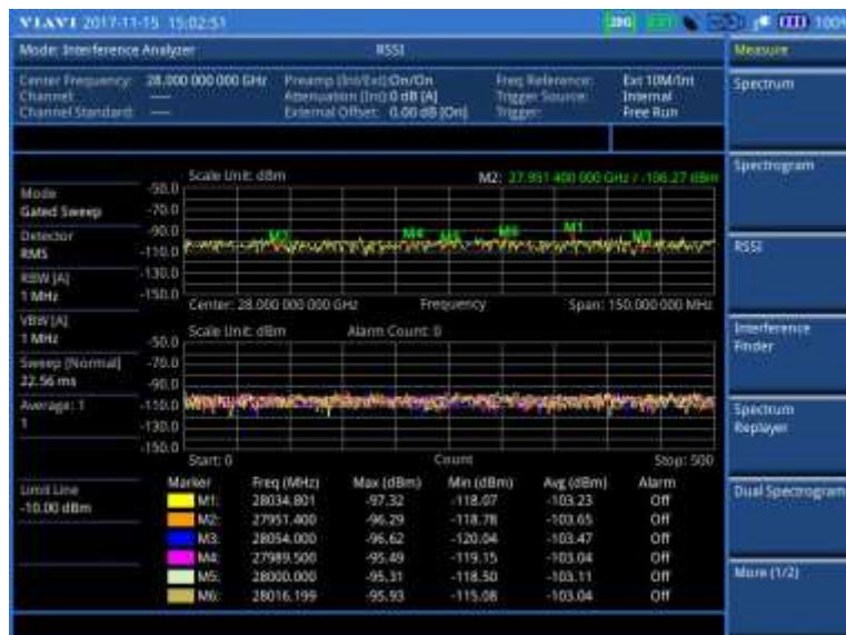
Figure 54 Interference measurement in RSSI (on 28 GHz downconverter)
