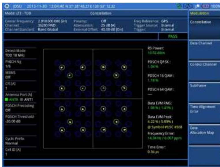
Figure 173 Constellation measurement with LTE-TDD signal analyzer
