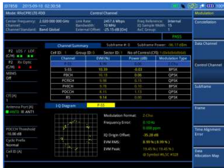
Figure 368 Control channel measurement with RFoCPRI LTE-FDD signal analyzer
