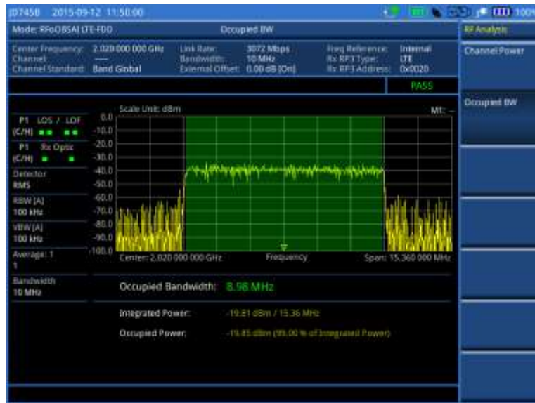
Figure 427 Occupied bandwidth measurement with RFoBSAI LTE-FDD signal analyzer
