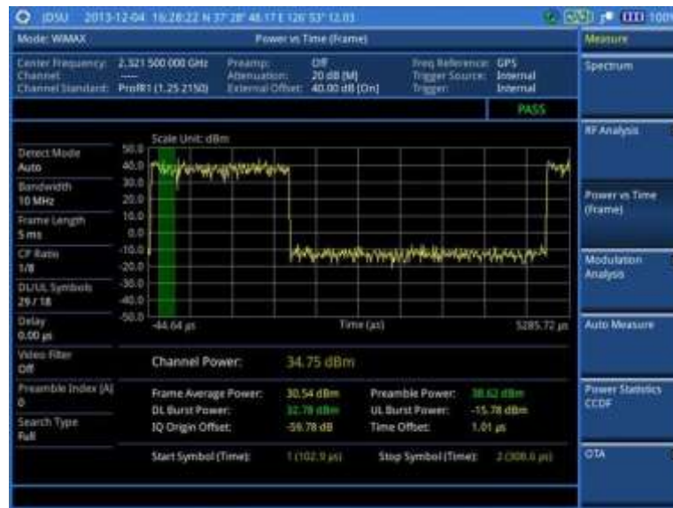
Figure 287 Power vs. time (frame) measurement with Mobile WiMAX signal analyzer
