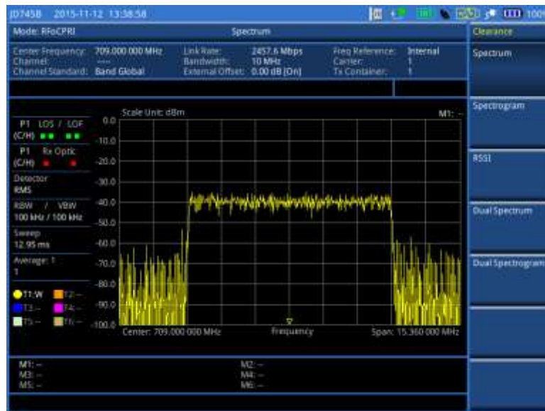
Figure 398 Example of spectrum measurement in BBU emulation
