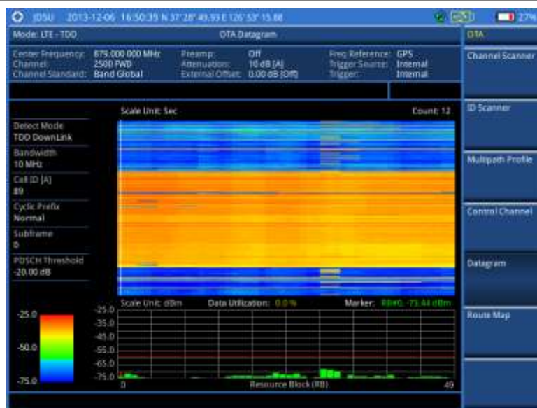
Figure 194 Datagram measurement with LTE-TDD signal analyzer
