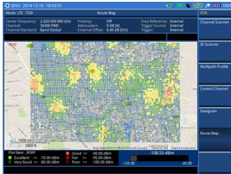
Figure 202 Raster image overlaid on the base map with LTE-TDD OTA signal analyzer
