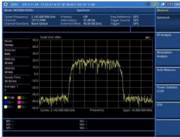
Figure 87 Spectrum measurement screen with WCDMA signal analyzer
