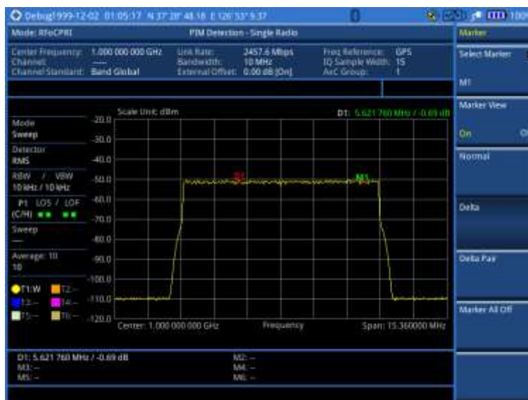
Figure 359 PIM detection of single radio
