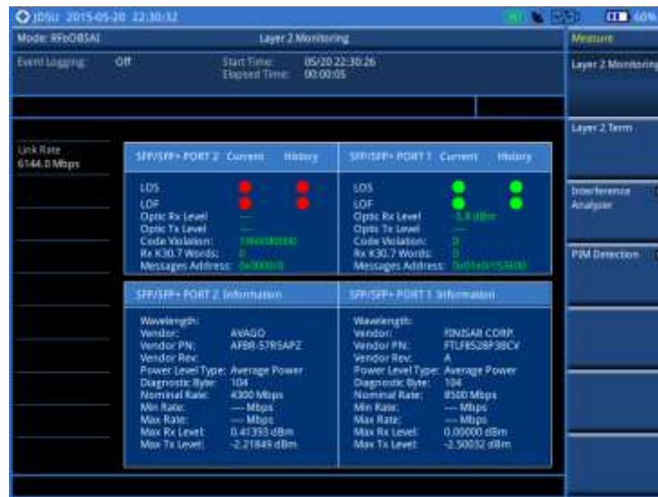
Figure 414 OBSAI RP3 layer 2 monitoring
