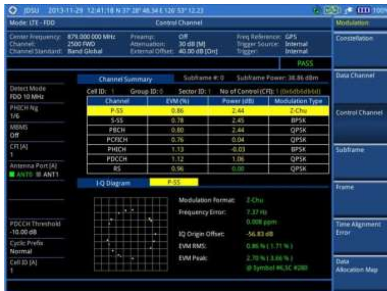
Figure 126 Control channel measurement with LTE-FDD signal analyzer
