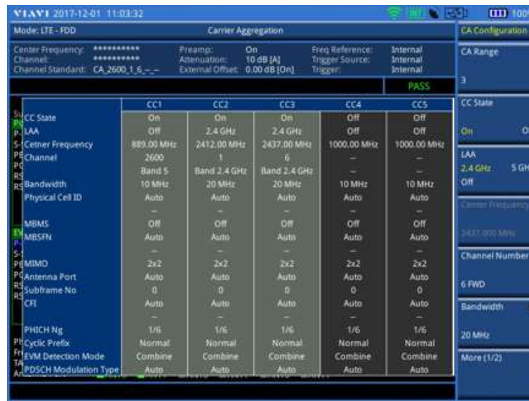
Figure 139 LAA (Licensed Assited Access) measurement with LTE-FDD signal analyzer
