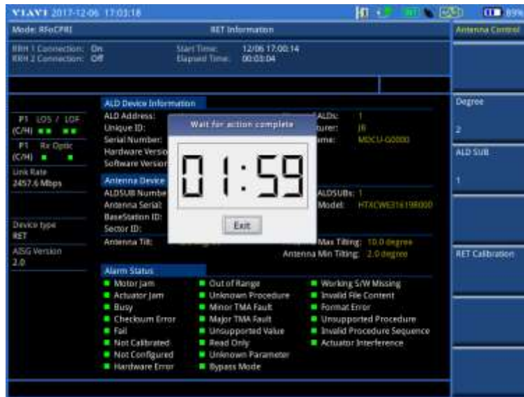
Figure 410 Example of antenna tilting in RET information
