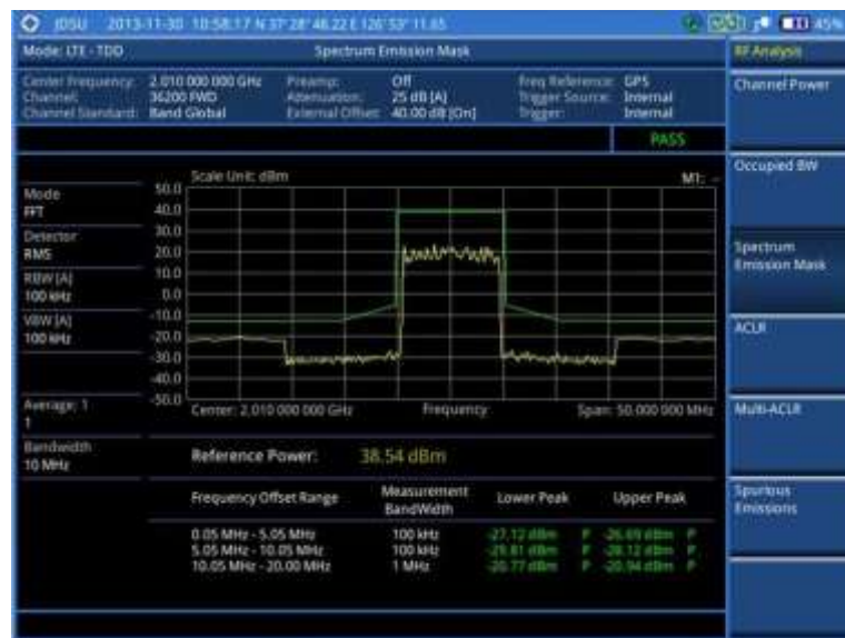
Figure 167 SEM measurement with LTE-TDD signal analyzer
