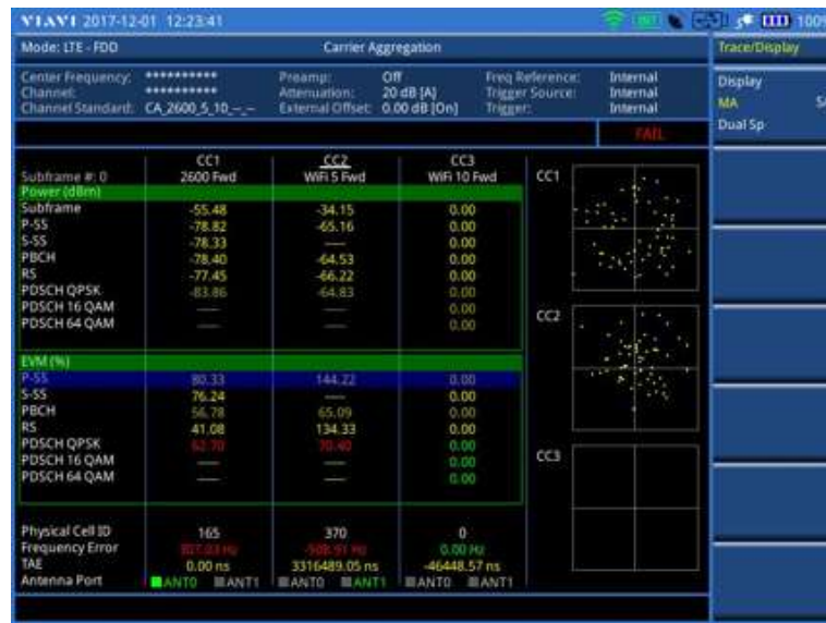
Figure 140 Carrier aggregation measurement with LTE-FDD signal analyzer (MA)
