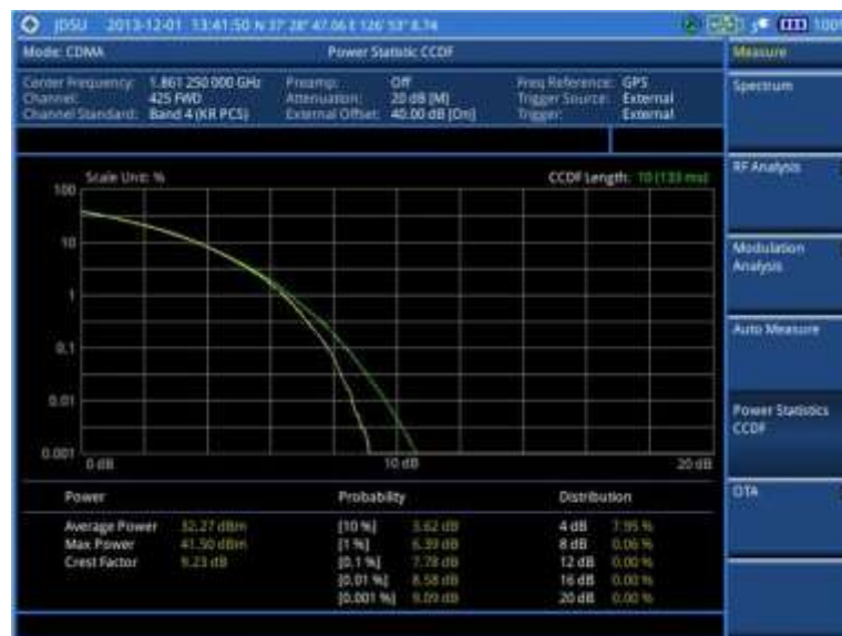
Figure 221 CCDF measurement with CDMA signal analyzer
