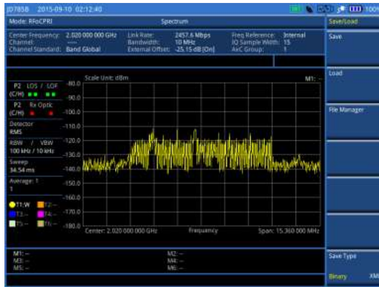
Figure 345 RFoCPRI spectrum measurement
