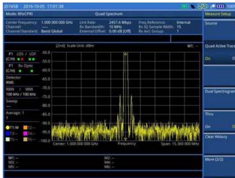
Figure 351 RFoCPRI quad spectrum with quad active trace off
