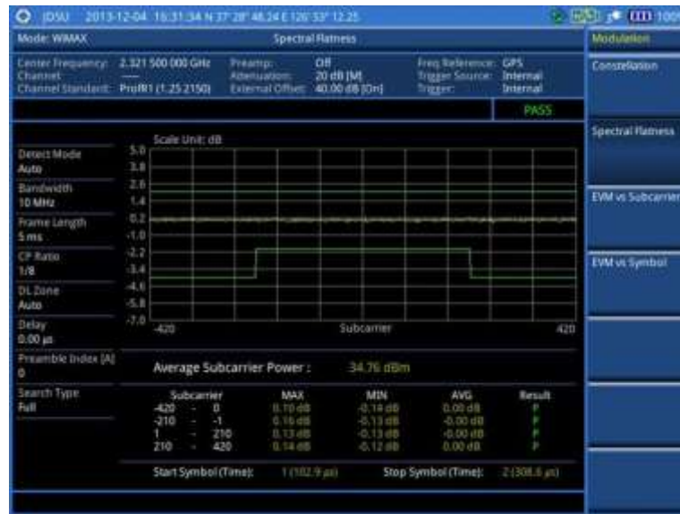
Figure 289 Spectral flatness measurement with Mobile WiMAX signal analyzer
