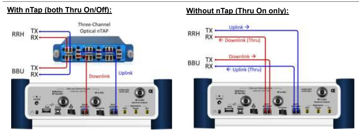
Figure 335 Connection diagram for Layer-2 monitoring mode
