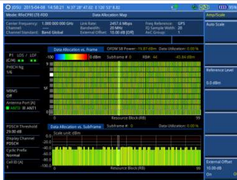
Figure 372 Data allocation map measurement with RFoCPRI LTE-FDD signal analyzer
