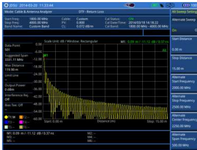
Figure 325 DTF measurement with the alternate sweep on
