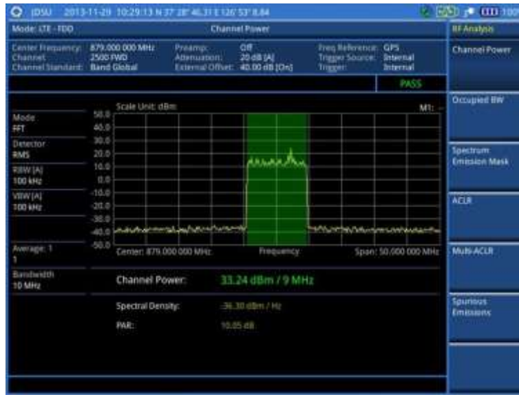
Figure 114 Channel power measurement with LTE-FDD signal analyzer
