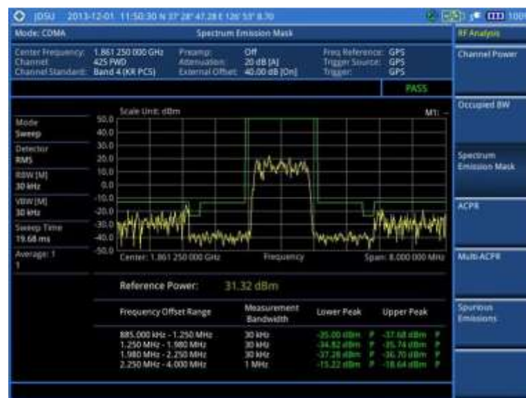
Figure 212 SEM measurement with CDMA signal analyzer
