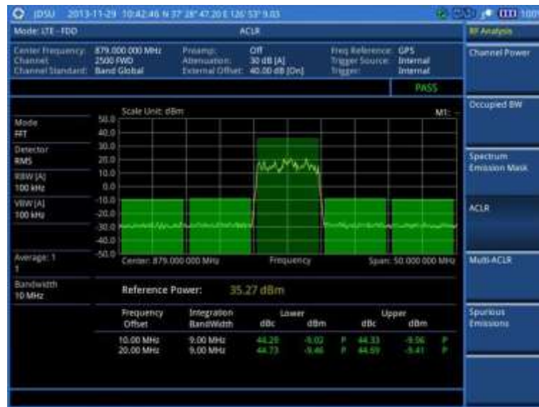
Figure 117 ACLR measurement with LTE-FDD signal analyzer
