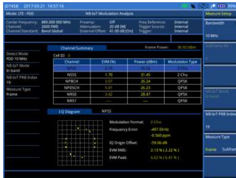
Figure 157 NB-IoT modulation measurement with LTE-FDD signal analyzer (Frame)
