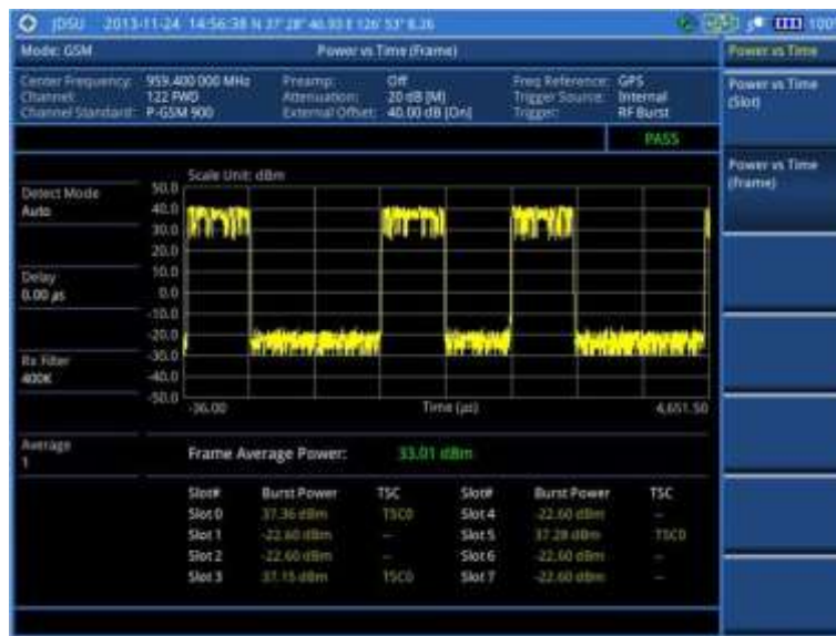
Figure 75 Power vs. time (frame) measurement with GSM signal analyzer
