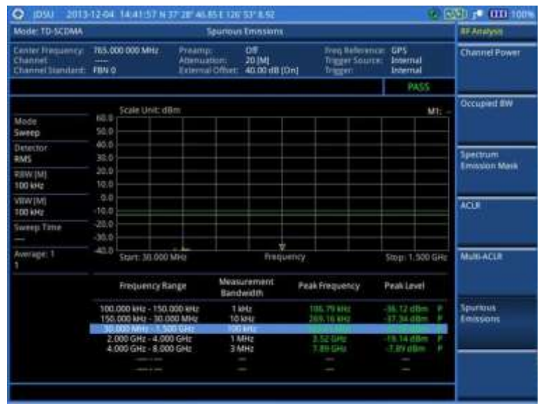
Figure 263 Spurious emissions measurement with TD-SCDMA signal analyzer
