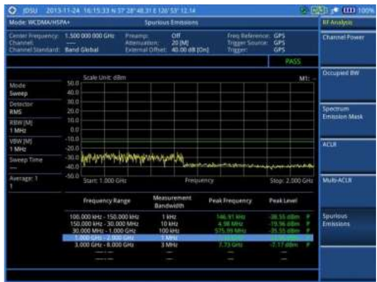
Figure 93 Spurious emissions measurement with WCDMA/HSPA+ signal analyzer
