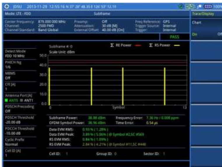
Figure 129 Subframe measurement with LTE-FDD signal analyzer (Chart On)
