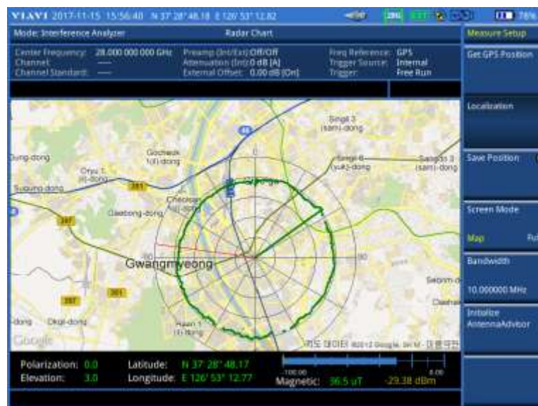
Figure 62 Localized RSSI data on the radar chart (on 28 GHz downconverter)
