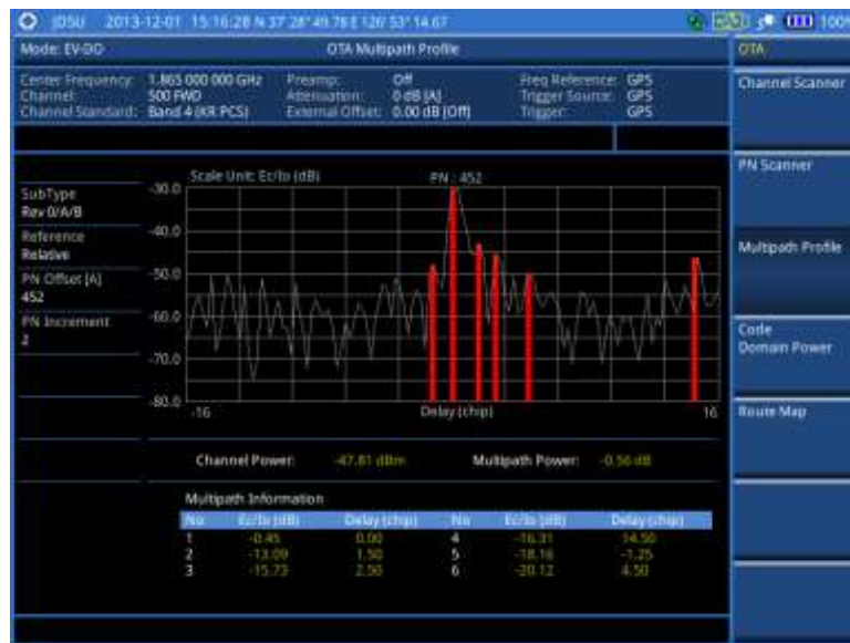
Figure 249 Multipath profile measurement with EV-DO OTA signal analyzer
