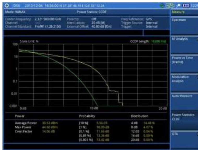
Figure 292 CCDF measurement with Mobile WiMAX signal analyzer
