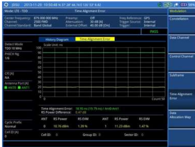
Figure 182 Time alignment error measurement with LTE-TDD signal analyzer
