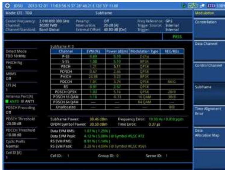
Figure 179 Subframe measurement with LTE-TDD signal analyzer
