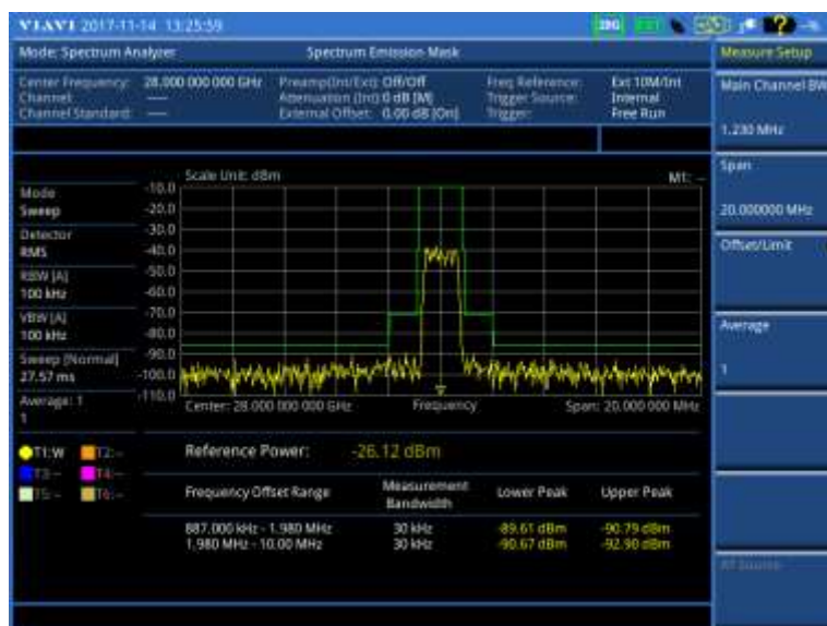
Figure 27 Spectrum emission mask measurement with spectrum analyzer (on 28 GHz downconverter)
