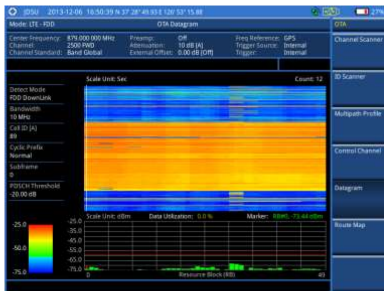
Figure 147 Datagram measurement with LTE-FDD signal analyzer
