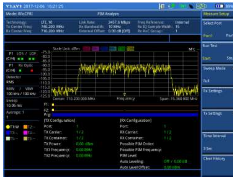
Figure 404 Example of single port sweep mode PIM Analysis in BBU emulation
