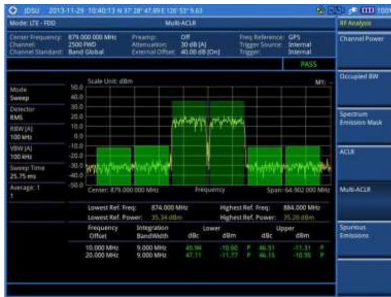
Figure 118 Multi-ACLR measurement with LTE-FDD signal analyzer
