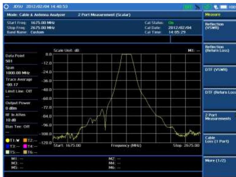
Figure 333 2-port scalar measurement
