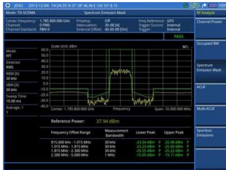
Figure 260 SEM measurement with TD-SCDMA signal analyzer
