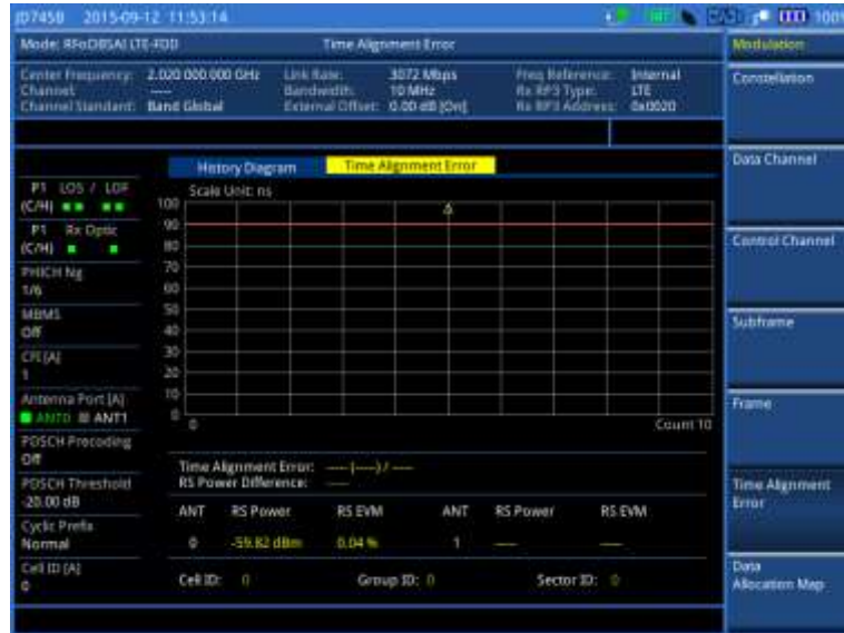
Figure 434 Time alignment error measurement with RFoBSAI LTE-FDD signal analyzer
