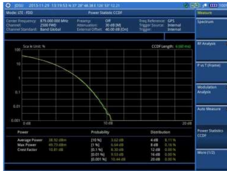
Figure 138 CCDF measurement with LTE-FDD signal analyzer
