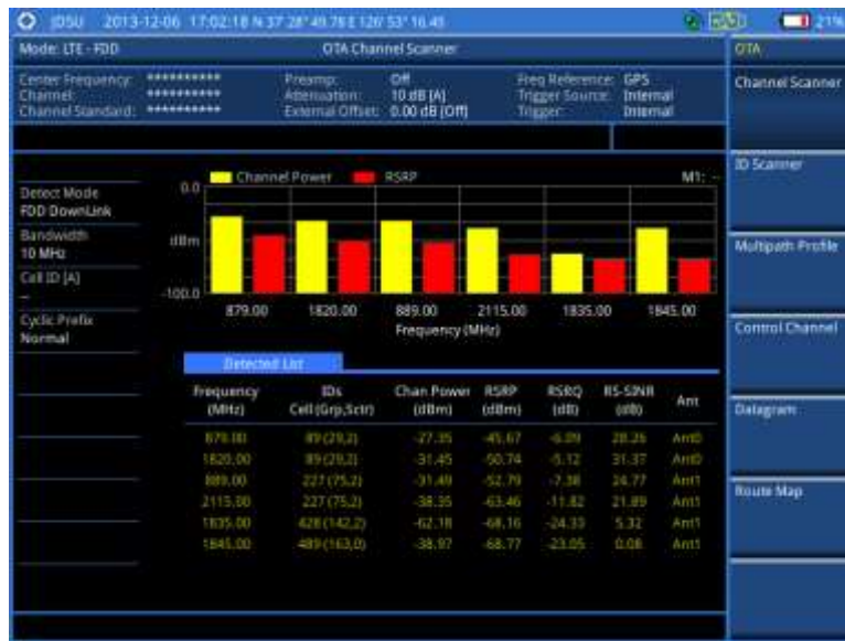
Figure 143 Channel scanner measurement with LTE-FDD OTA signal analyzer
