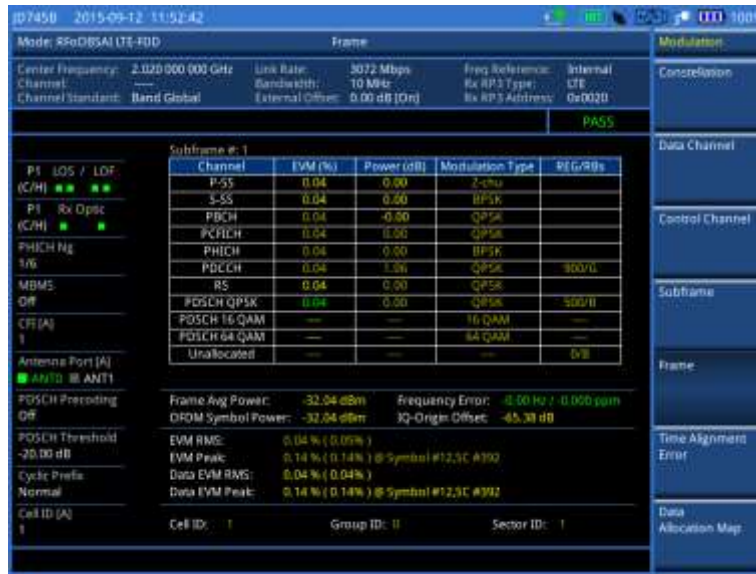
Figure 433 Frame measurement with RFoBSAI LTE-FDD signal analyzer
