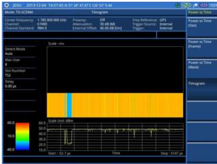
Figure 267 Timogram with TD-SCDMA signal analyzer
