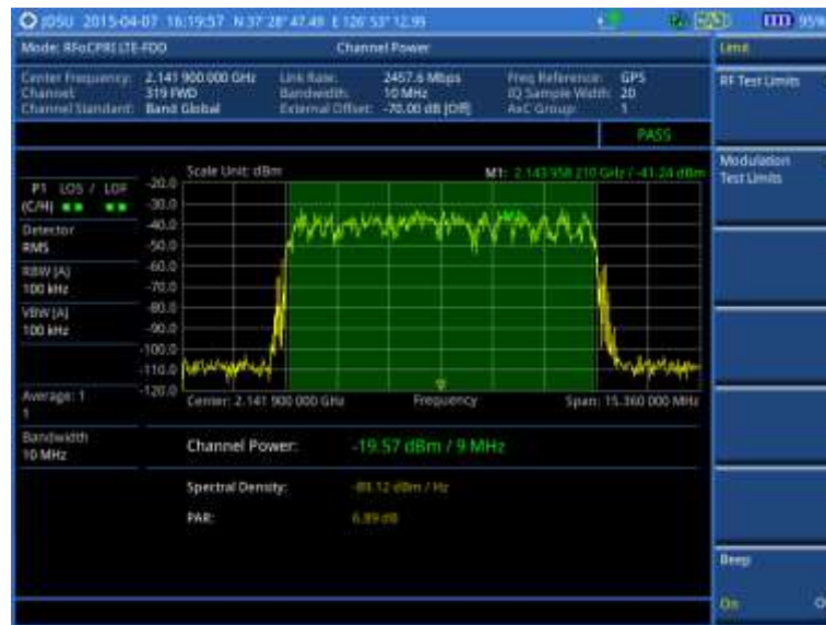
Figure 363 Channel power measurement with RFoCPRI LTE-FDD signal analyzer
