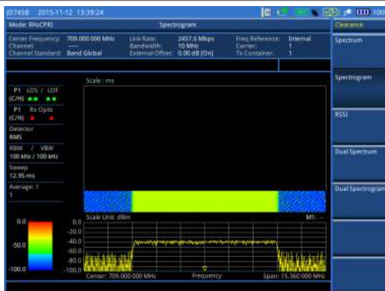
Figure 400 Example of spectrogram in BBU emulation
