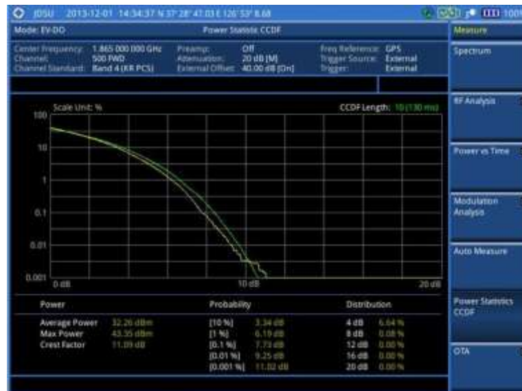
Figure 246 CCDF measurement with EV-DO signal analyzer
