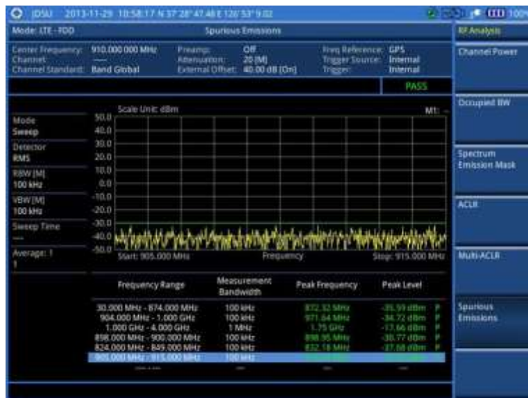
Figure 119 Spurious emissions measurement with LTE-FDD signal analyzer
