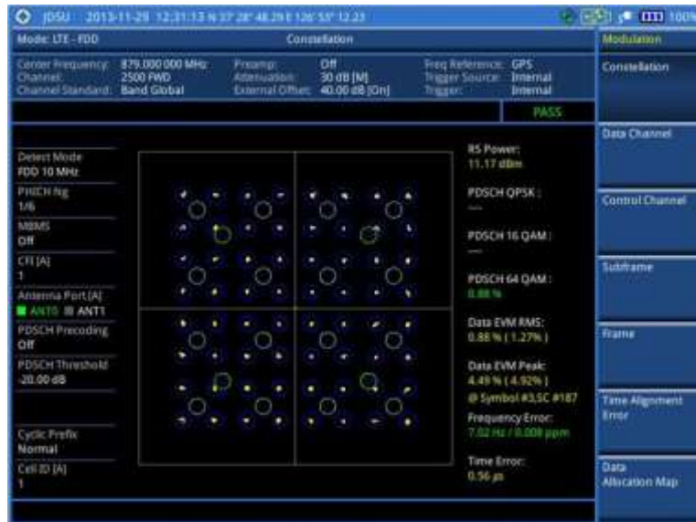
Figure 121 Constellation measurement with LTE-FDD signal analyzer
