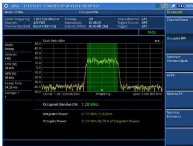
Figure 211 Occupied bandwidth measurement with CDMA signal analyzer
