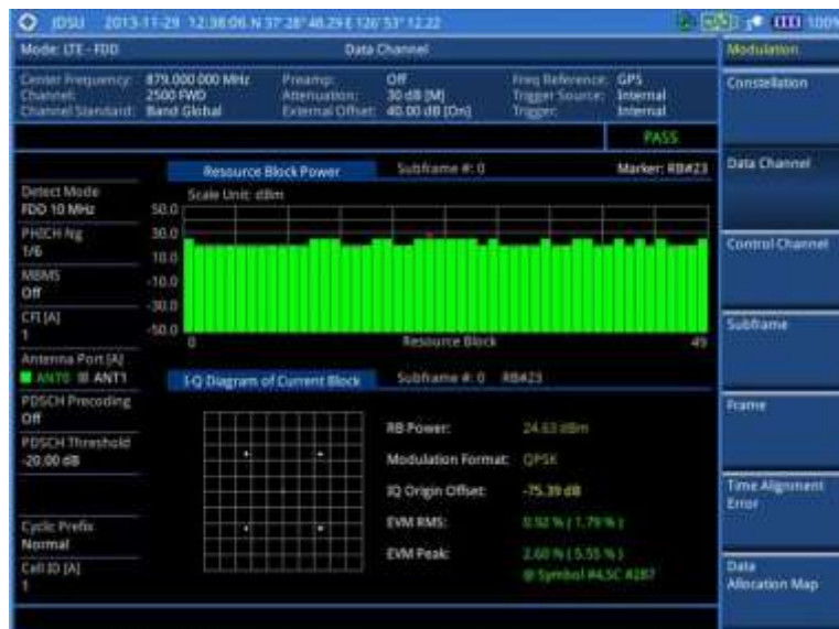
Figure 123 Data channel measurement with LTE-FDD signal analyzer
