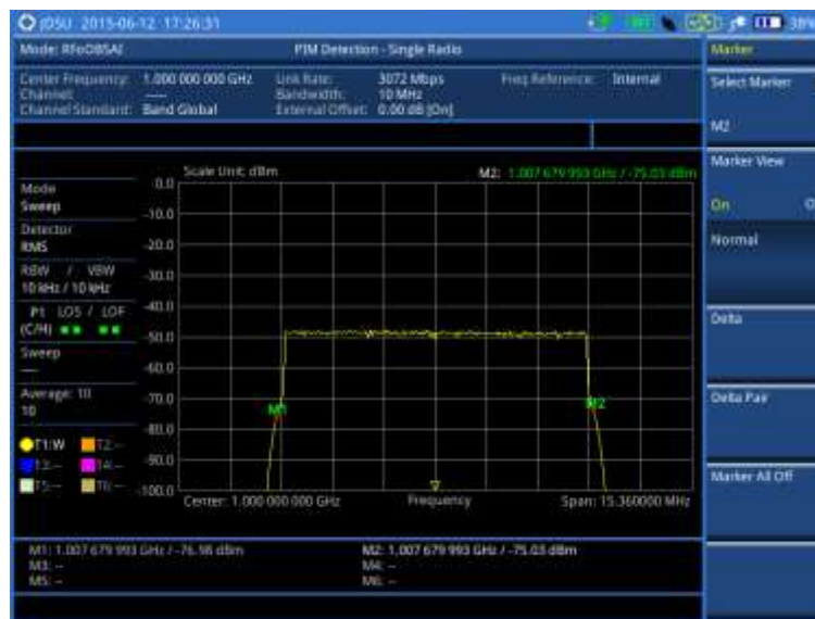
Figure 423 PIM detection of single radio
