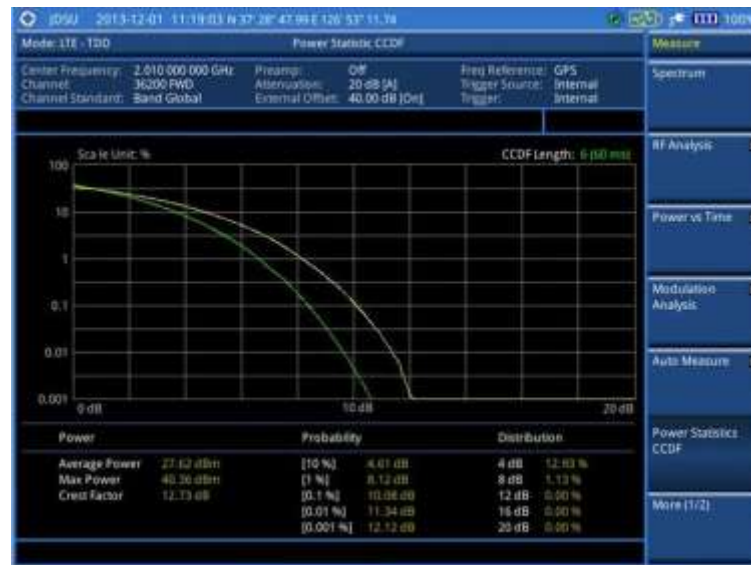
Figure 186 CCDF measurement with LTE-TDD signal analyzer
