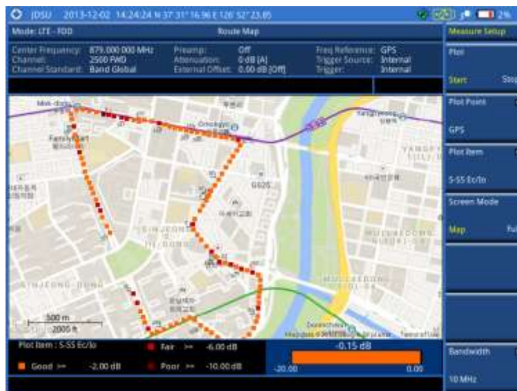
Figure 154 Route map measurement (S-SS Ec/Io) with LTE-FDD OTA signal analyzer
