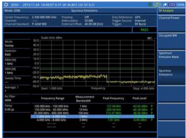
Figure 72 Spurious emissions measurement with GSM signal analyzer
