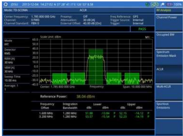
Figure 261 ACLR measurement with TD-SCDMA signal analyzer
