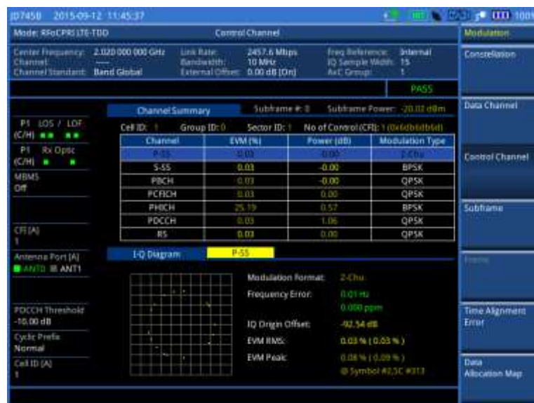
Figure 381 Control channel measurement with RFoCPRI LTE-TDD signal analyzer
