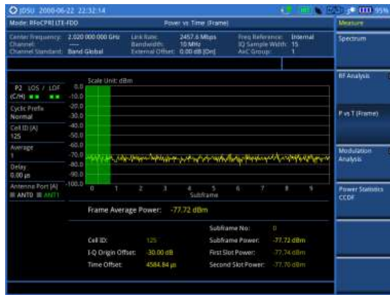
Figure 365 Power vs. time (frame) measurement with RFoCPRI LTE-FDD signal analyzer
