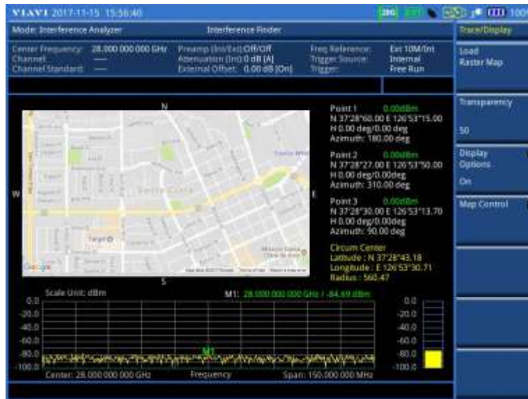
Figure 58 Raster image overlaid on the map in interference finder (on 28 GHz downconverter)
