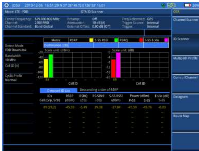
Figure 144 ID scanner measurement with LTE-FDD OTA signal analyzer
