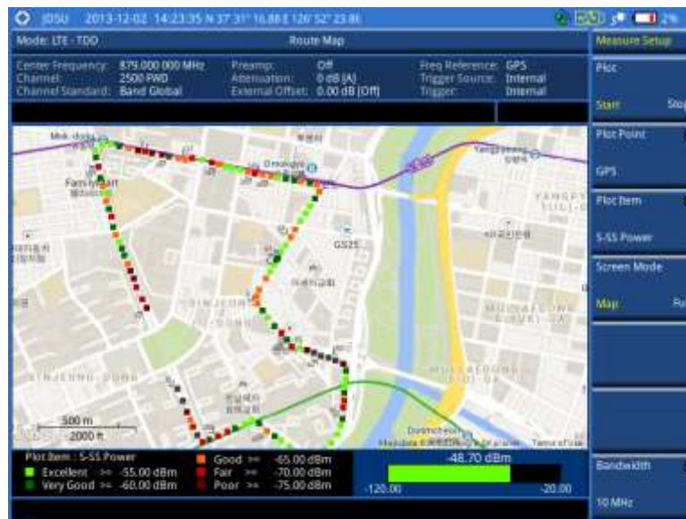
Figure 200 Route map measurement (S-SS Power) with LTE-TDD OTA signal analyzer
