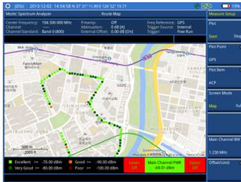
Figure 38 Route map measurement screen with GPS
