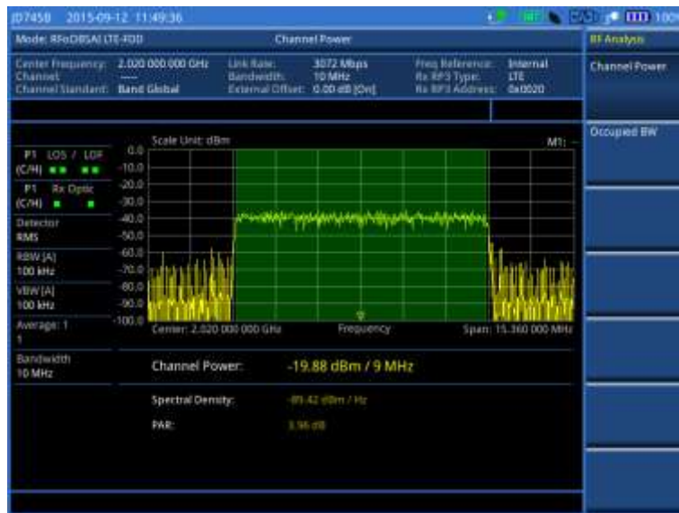
Figure 426 Channel power measurement with RFoOBSAI LTE-FDD signal analyzer
