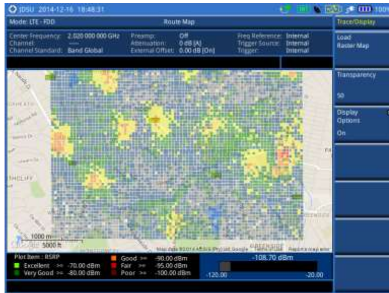
Figure 155 Raster image overlaid on the base map with LTE-FDD OTA signal analyzer
