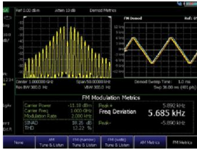
Characterize AM/FM signals using AM/FM demodulation
