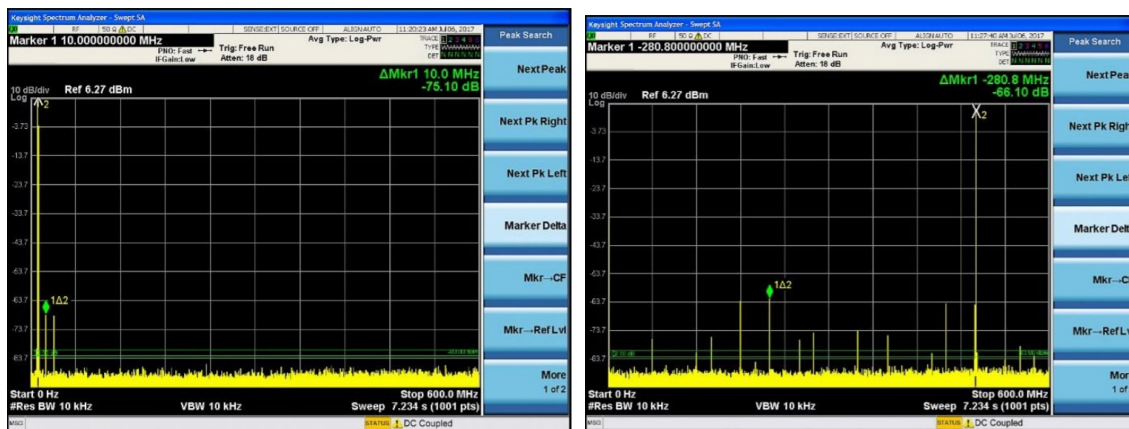
Figure 3. (Left) Measured IQ output, 10 MHz tone spectrum. (Right) Measured IQ output, 500 MHz tone spectrum.
