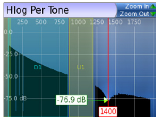
A bridged tap causes a dip on the Hlog graph; this example shows a bridged tap length of approximately 8 m
