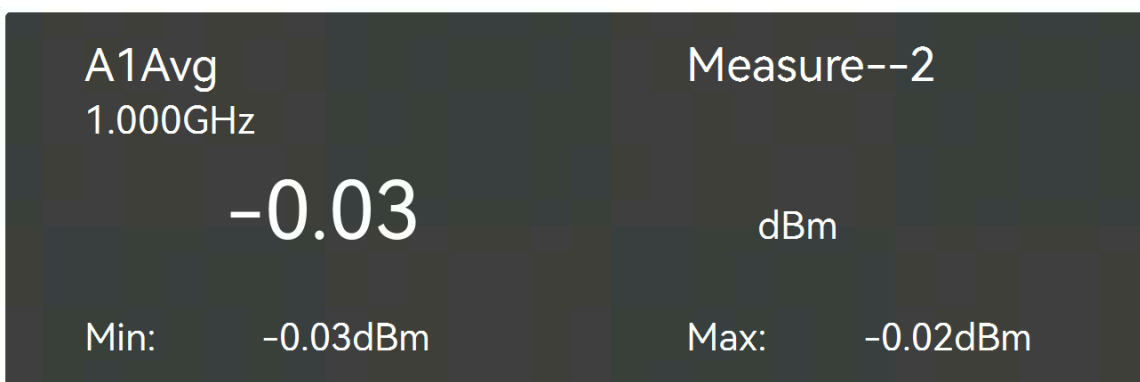
Figure 4.19 Power display window
