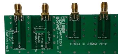
Termination board tuned at 2500MHz:
