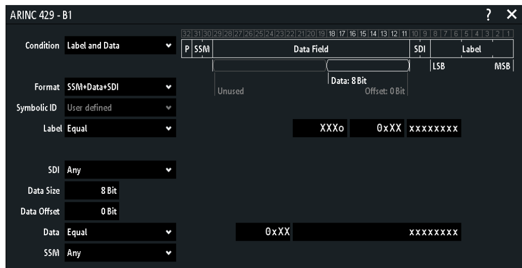
Figure 13-49: Settings for search on ARINC 429 bus
