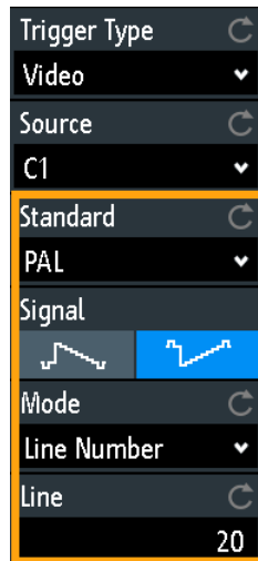
Figure 6-5: Video trigger menu
