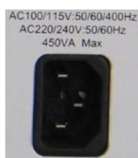
110 V/220 V self-adaptive AC power module
