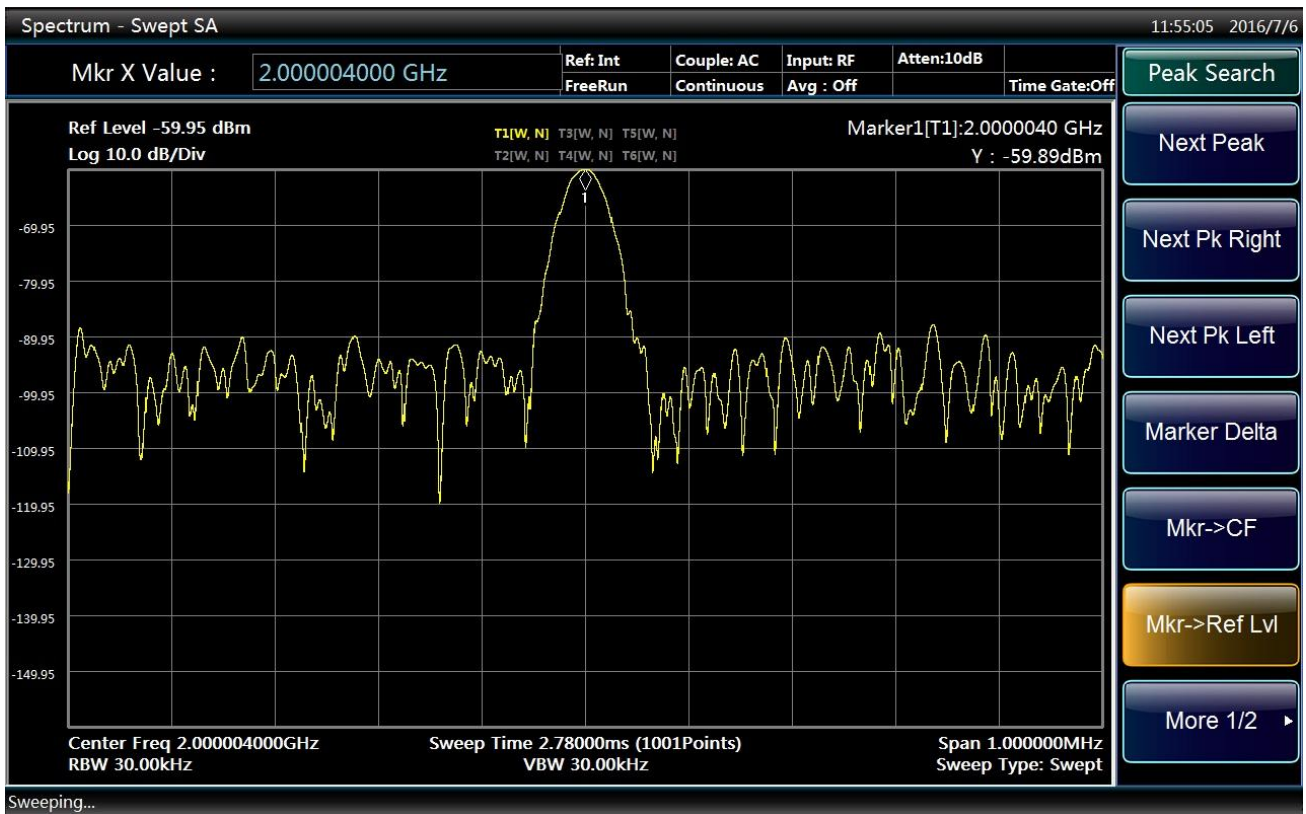
Fig. 4.22 Display interface of second harmonic amplitude
