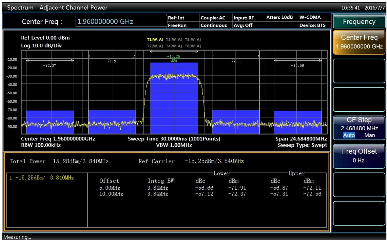
Fig 4.66 Results of Adjacent Channel Power Measurement
