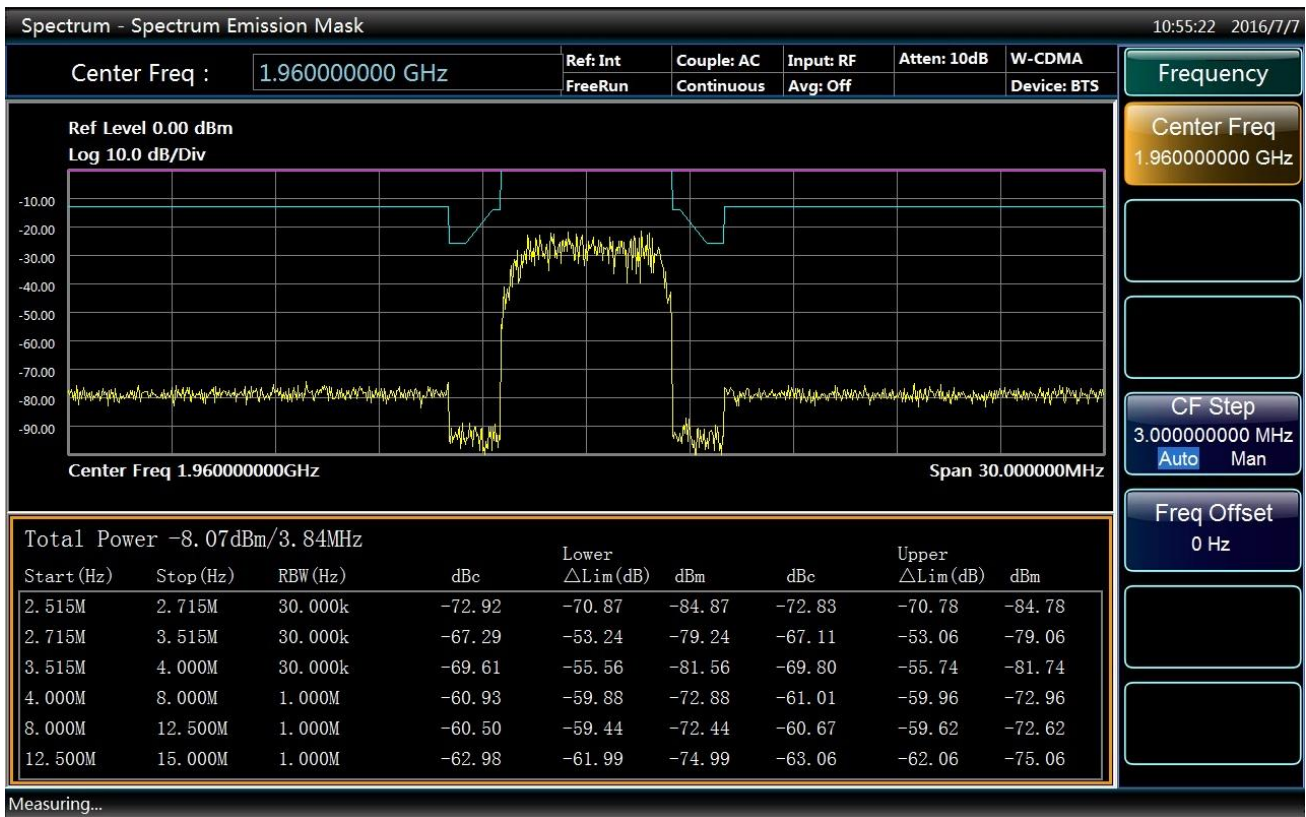
Fig. 4.83 Results of Spectrum Emission Mask Measurements
