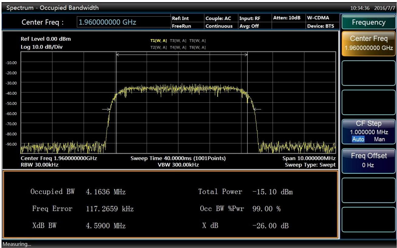
Fig. 4.64 Results of occupied bandwidth measurements
