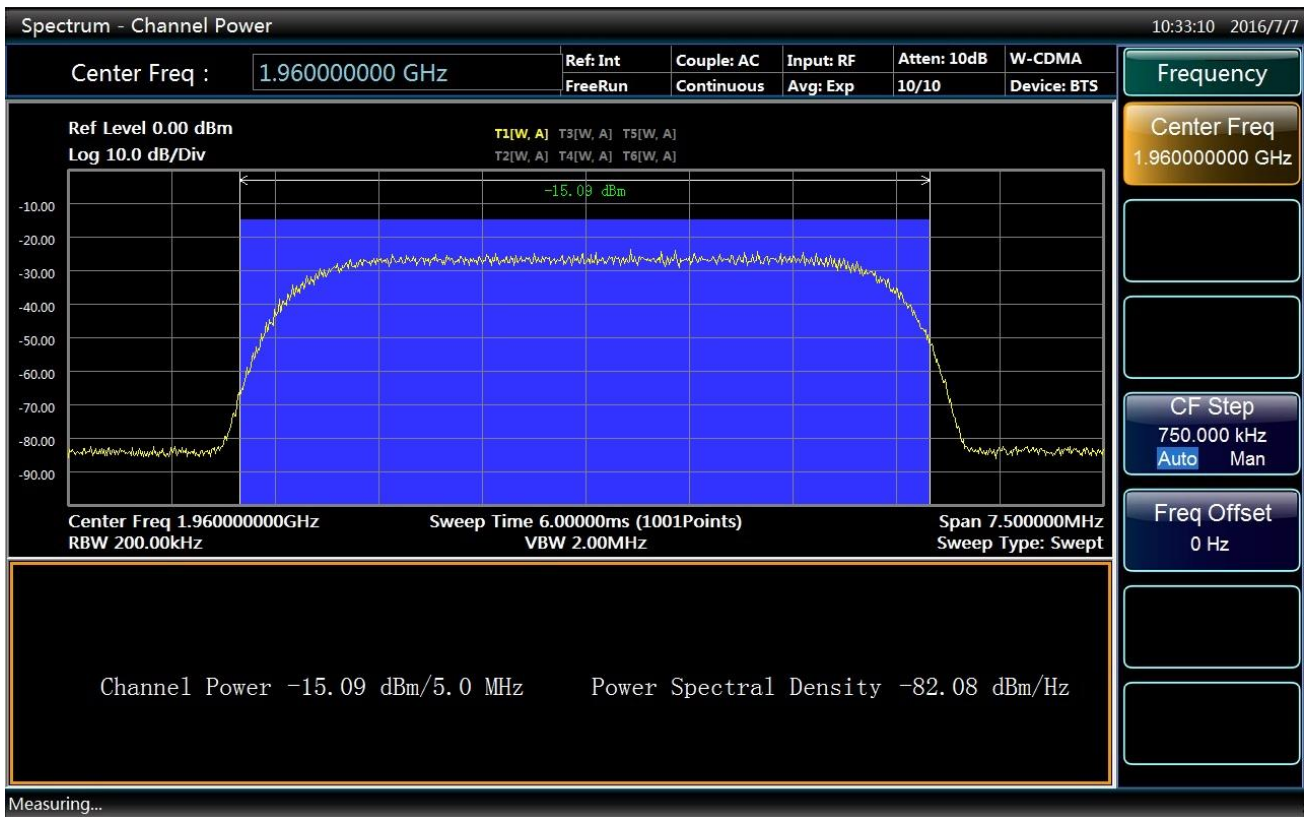
Fig 4.62 Results of channel power measurement
