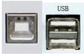
Fig. 2.24 USB Connector (the Type B/Type A Configurations are On the Left/Right Side)
