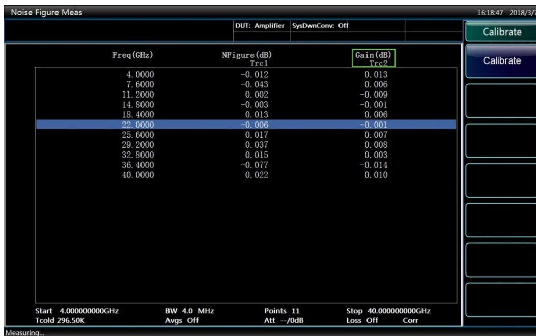
Figure 3.2 Typical Table Display Result after Calibration
