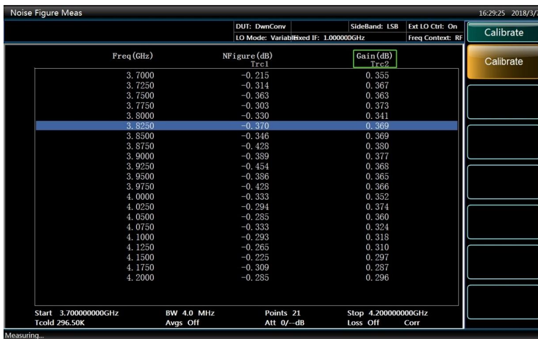
Fig.3.10 Typical calibrated results at the downconverter measurement mode
