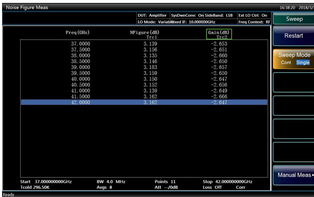
Fig.3.20 Typical Measurement Values at System Downconverter Measurement Mode
