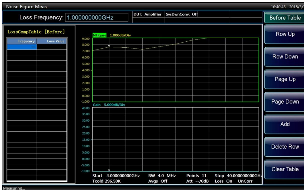
Figure 3.27 Empty loss table
