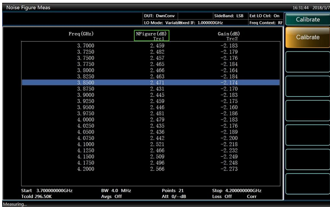
Fig.3.12 Typical measurement values at the downconverter measurement mode
