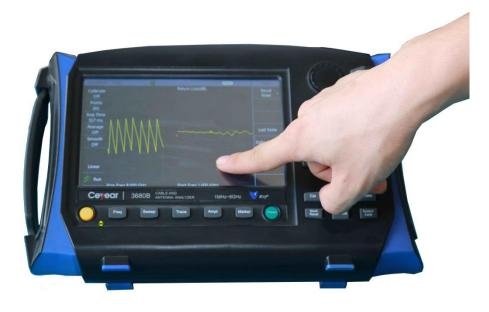
Finger sliding to switch measurement types
