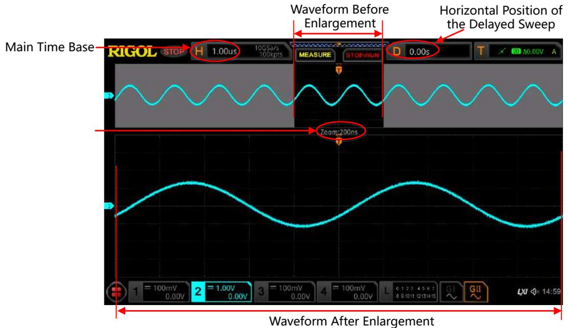
**Figure 6.1 Delayed Sweep Mode**
