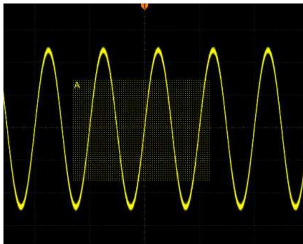
If you enable Zone A, select CH1 as Source A and select "Intersect" as the condition, the following figure is displayed.
