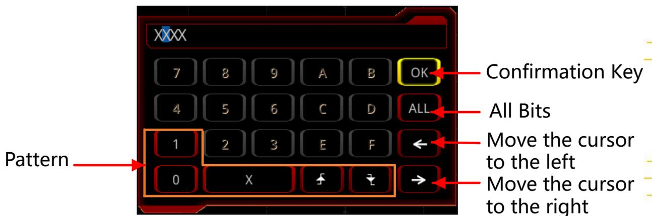
**Figure 8.6 Virtual Keypad for Pattern Setting**
