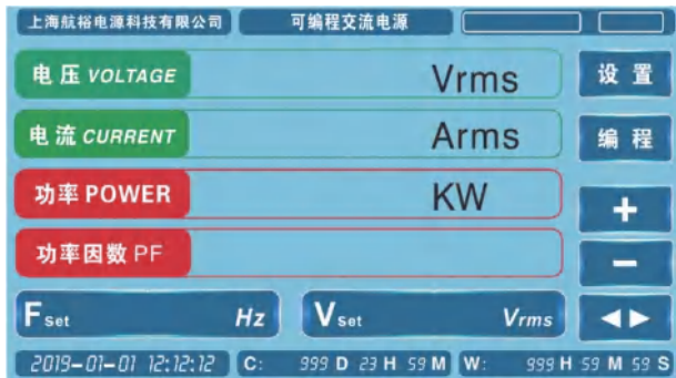
Single phase power supply main interface
